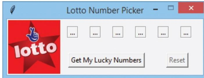
Static text appears on the window title bar and on the Button widgets, the window's resize button is disabled, the small Labels contain their initial ellipsis text values, and the "Reset" button is in its initial disabled state.
