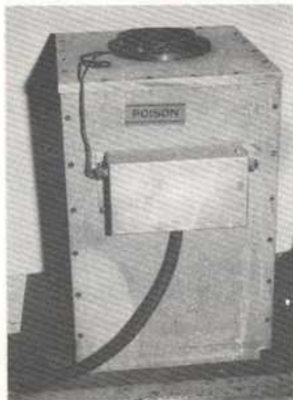
Fig. 57 A pot furnace suitable for temperatures up to 950°C.
