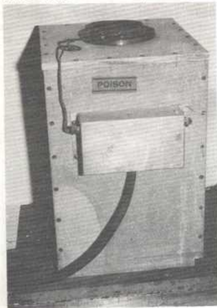
Fig. 34 The author's laboratory type Austenising salt-pot furnace. Construction is described on page 98. Note that the "POISON" label refers to previous use with a cyanide hardening pot.
