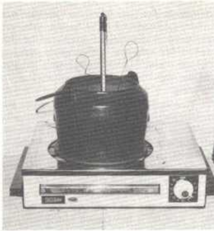
Fig. 20 A simple tempering salt bath. The outer case of a cast-iron glue-pot is set on an electric boiling ring. Note the protective case on the thermometer. Normally a glass-fibre insulating blanket is wrapped round the pot, but was removed for the photograph.
