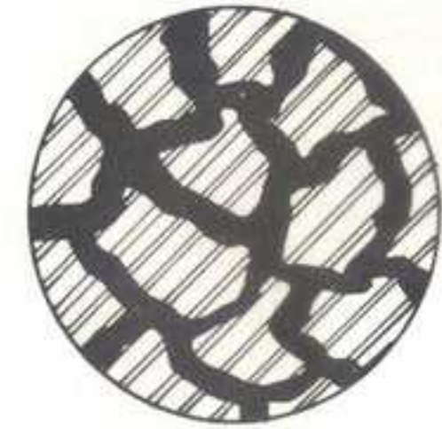
Fig. 14 Grains of Pearlite surrounded by borders of Iron Carbide (Cementite).
