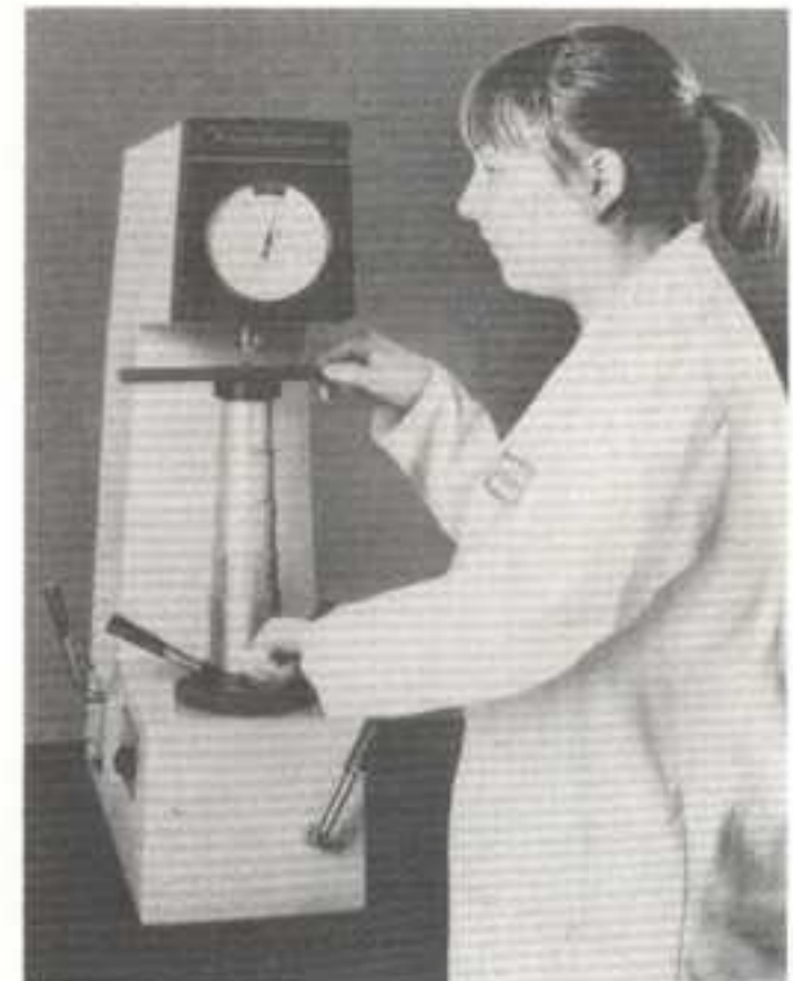
Fig. 47 Hardness testing using a Rockwell type machine. The depth of the impression is shown on the large dial indicator. (Courtesy Avery-Denison Ltd).
