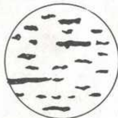
Fig. 5 Structure of wrought iron "along the grain" showing the slag inclusions.
