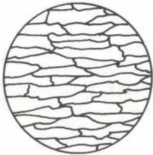
Fig. 40 Elongation of the grains of steel caused by mechanical forming processes.
