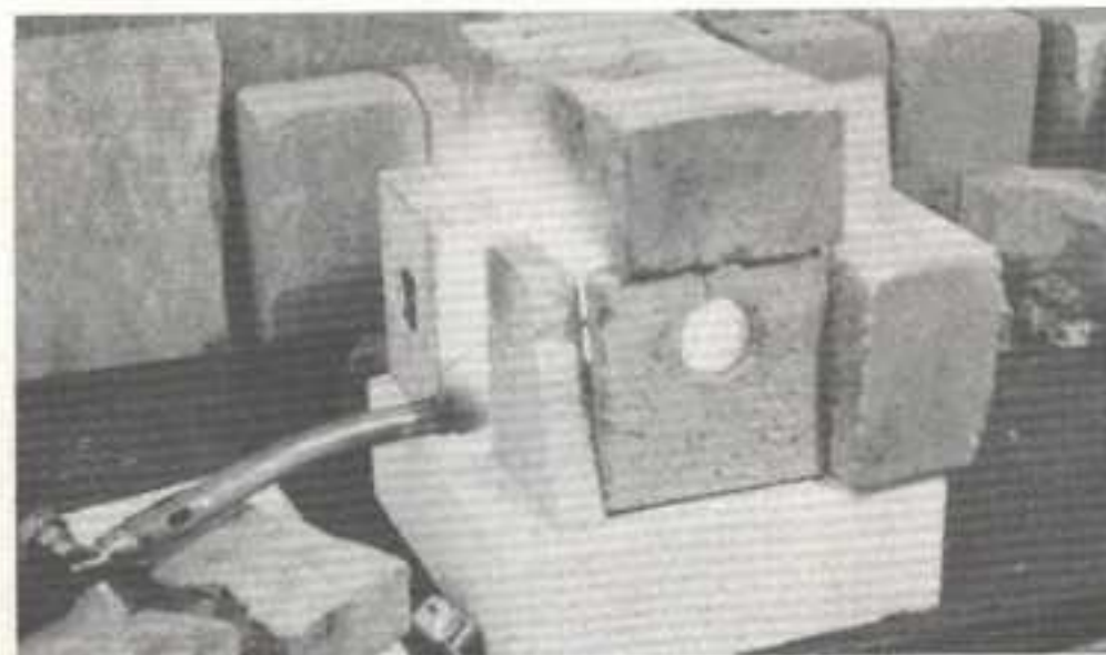
Fig. 31 A very simple gas-fired tube furnace.
