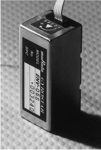
Figure 8. The Gyrostar manufactured by Murata Electronics. This is a small, relatively inexpensive, single-axis piezoelectric rate gyroscope originally developed for the automobile market and active suspension systems. (See B. Barshan and H. F. Durrant-Whyte, IEEE Trans. Robot. Autom. 11 (3), 328–342, June 1995. Copyright IEEE, 1995.)
