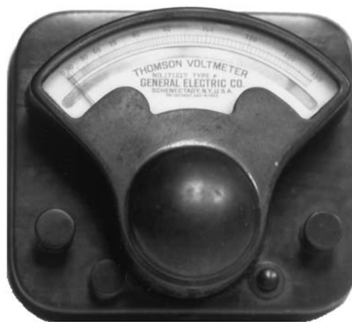
Figure 9. Example ac voltmeter incorporating full-wave rectification technique. Photo by Bill Dabbs.
