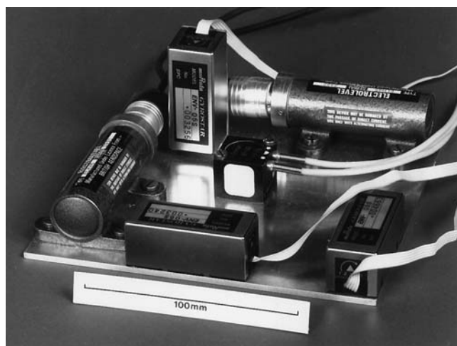
Figure 22. A low-cost INS comprising three gyroscopes, a triaxial accelerometer and two tilt sensors, developed for a mobile robot platform. (See B. Barshan and H. F. Durrant-Whyte, IEEE Trans. Robot. Automa. 11 (3), 328–342, June 1995. Copyright IEEE, 1995.)
