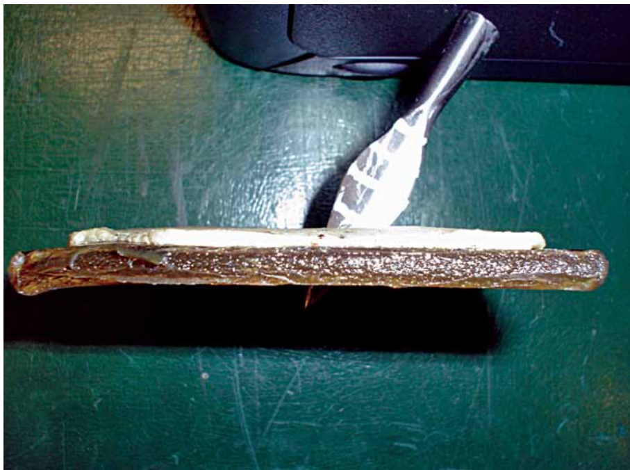
Figure 8. A side view of a specimen of boiled rawhide with a surface coating of crushed marble in hide glue. The arrowhead projects 9 mm from the rear face. Photograph by Edward Cheshire.
