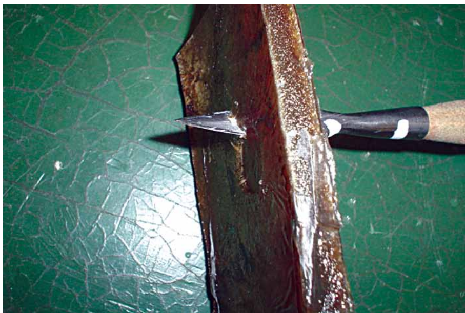
Figure 20. The arrowhead projects 19 mm from the rear face of the armour, but because of the thick padding there was no 'wound' in the plasticine except for a fabric impression 12 mm in diameter. The wearer would have received a bruise and perhaps a wound a few millimeters deep, depending on the impact site. Photograph by Edward Cheshire.
