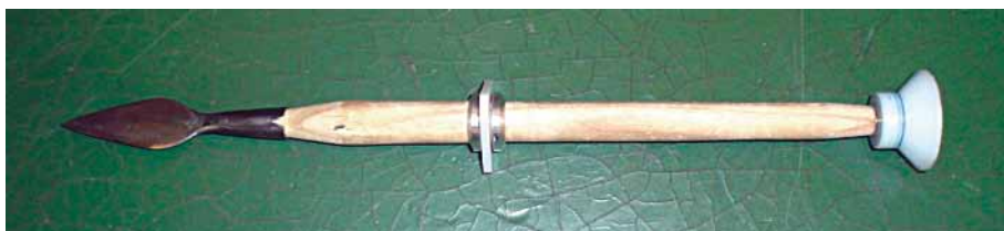
Figure 13. Typical trials arrow with piston seal and central 'spider'. Photograph by Edward Cheshire.
