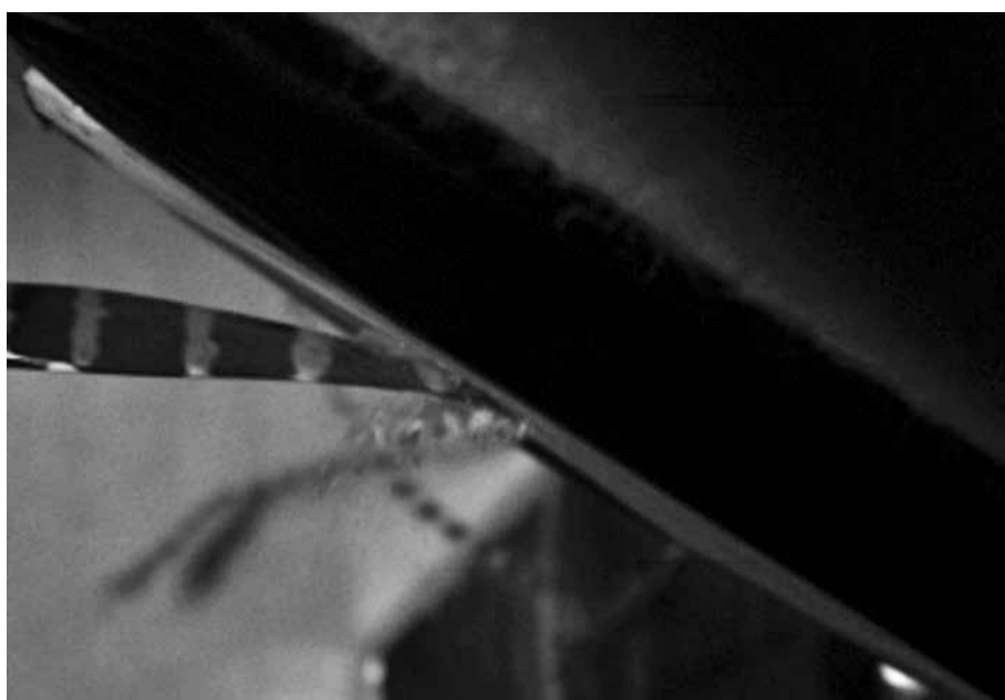
Figure 23. The arrowhead approaching from the left is bent downwards by the impact, 0.29 milliseconds after the initial contact. A small amount of marble facing is peeling off just below the point of the arrowhead. Photograph by Edward Cheshire.
