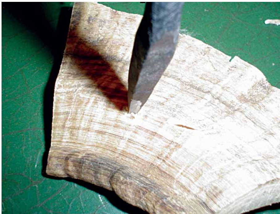
Figure 25. Ram's horn offers good resistance to penetration by arrows. Photograph by Edward Cheshire.
