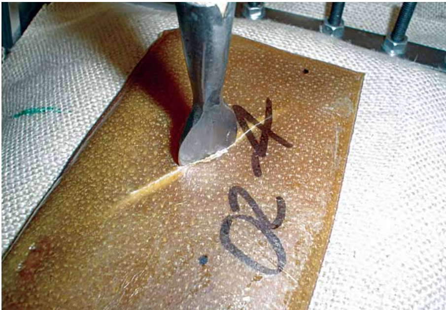
Figure 16. Tensile stress has caused cracks to start in this rawhide boiled in hide glue, but the fibrous structure of hide has permitted very little opening of the cracks and the arrow has been stopped with 14 mm projection from the rear face. Worn over a padded aketon this armour would have prevented a wound more than a few millimeters deep. Photograph by Edward Cheshire.
