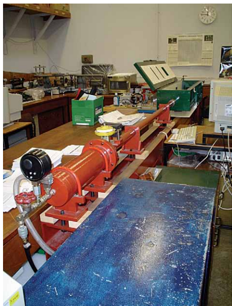
Figure 12. A view of the air gun looking from the breech end towards the arrow containment box, the lid of which is open. The larger red tube in the foreground is the air pressure vessel and the butterfly valve to release the compressed air to propel the arrow is yellow. The gun is muzzle loaded. Photograph by Edward Cheshire.
