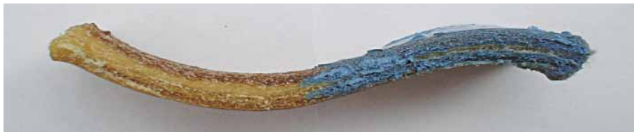
Figure 6. Rawhide after immersion in boiling water. The left side is natural material which has curled toward the flesh side because this face has taken up water faster. The flesh side on the right has been painted to slow down the ingress of liquid, so the curl is in the opposite direction. The cut edges swell first because of the larger area exposed. Photograph by Edward Cheshire.
