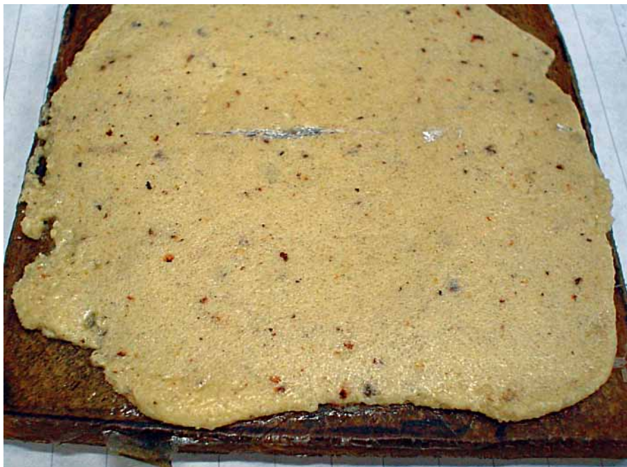
Figure 24. The marble facing received a minor scratch 18 mm long (visible running horizontally above the centre of the picture). Photograph by Edward Cheshire.
