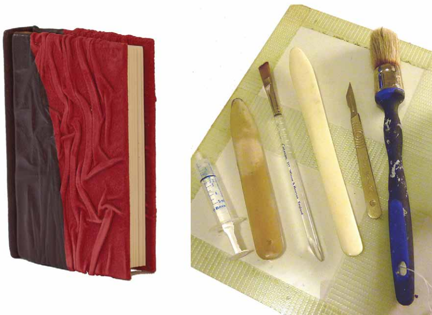
Figure 6. Left: Book with new leather binding. Right: Tools used in bookbinding and fine interior work. From left to right: Polyvinyl acetate (PVA) syringe; horn bone folder; small brush; bone folder; scalpel; paste brush; cotton wool; all resting on paring glass. Photographs by Laura Youngson Coll.
