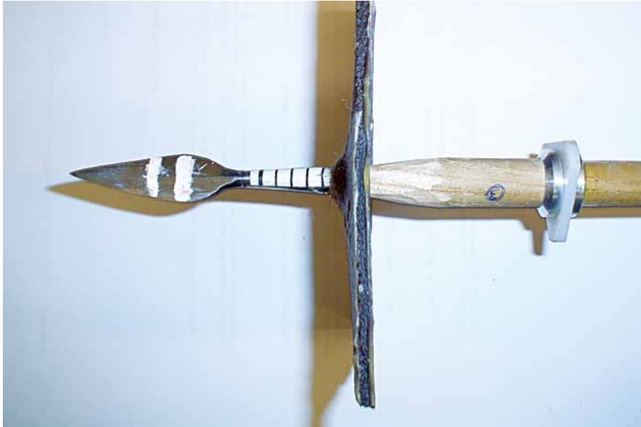
Figure 21. The arrowhead projects 88 mm from the rear face of leather impregnated with beeswax and would have penetrated much further into flesh rather than plasticine (about 200 mm if it did not hit bone). Photograph by Edward Cheshire.
