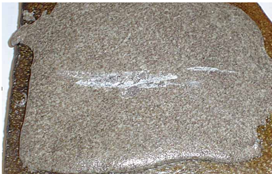
Figure 7. A typical specimen of hard-surfaced boiled rawhide. In this case the surface coating comprises carborundum grit and finely crushed marble in a matrix of hide glue. The scratches are from an arrow ricocheting without penetrating. Photograph by Edward Cheshire.
