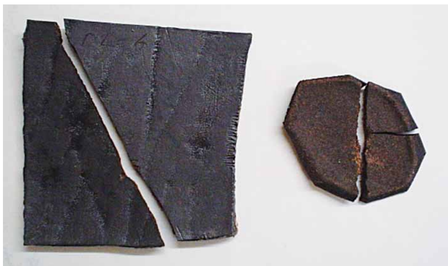
Figure 15. Boiled leather is brittle and shatters when struck by an arrow. Photograph by Edward Cheshire.
