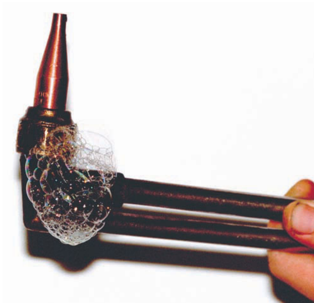
Figure 6.15 Checking a cutting tip for leaks
