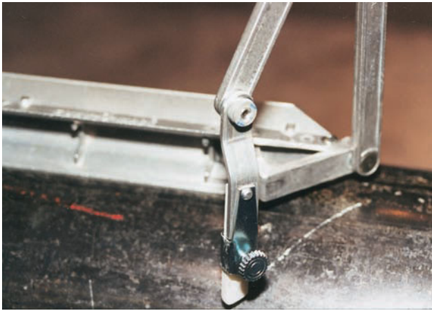
Figure 4.23 Pipe lateral being laid out with contour marker
