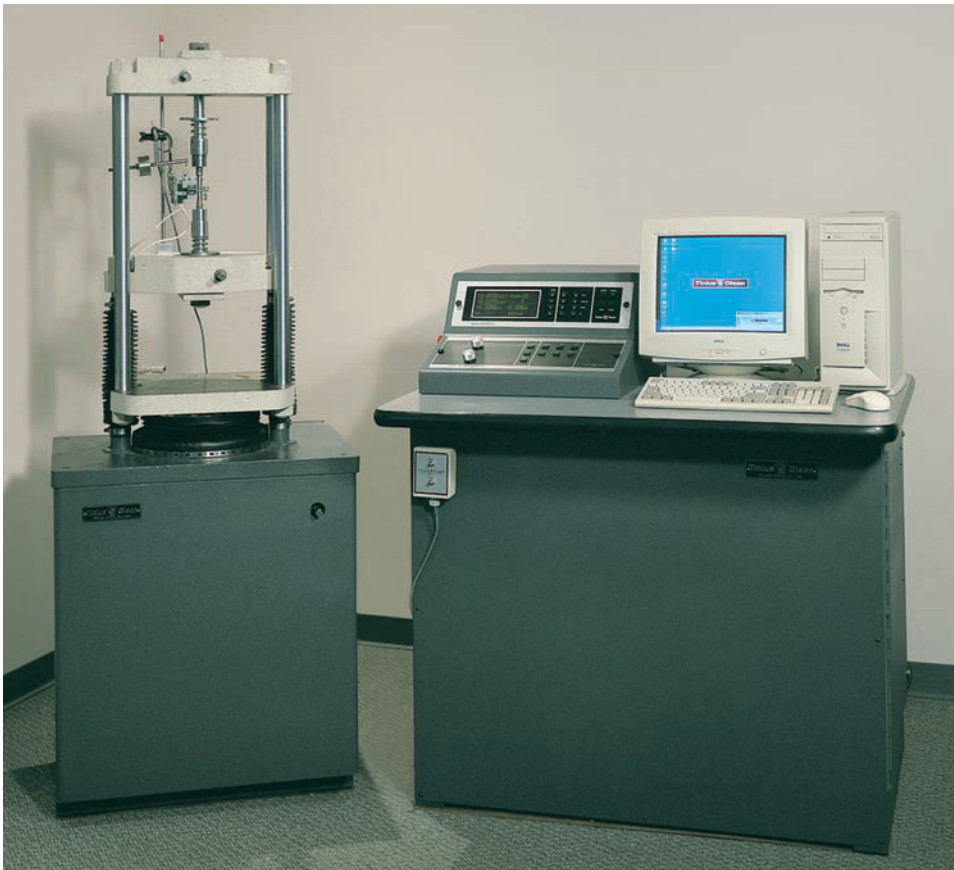
Figure 9.21 Typical tensile tester used for measuring the strength of welds (60,000-lb universal testing machines)
