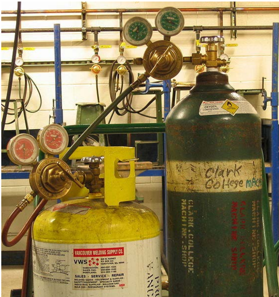
Compressed gas cylinders containing oxygen and MAPP gas.
