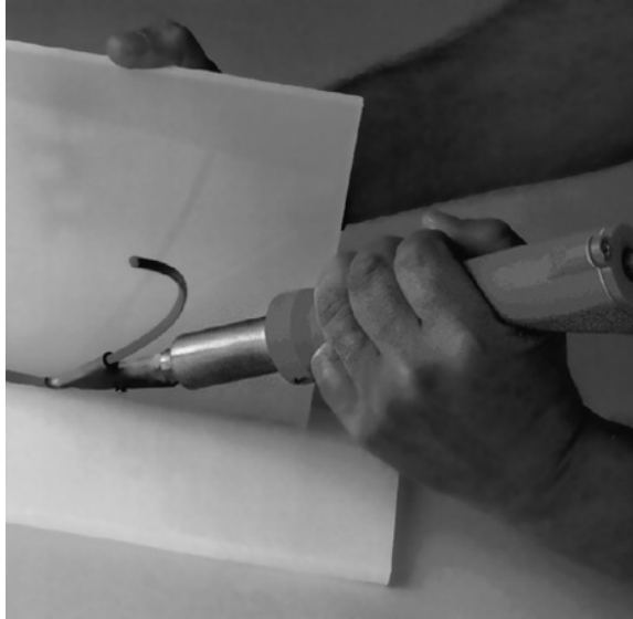
Figure 6.8 Hot gas welding of plastic (Source: Dr. Avi Benatar, The Ohio State University)
