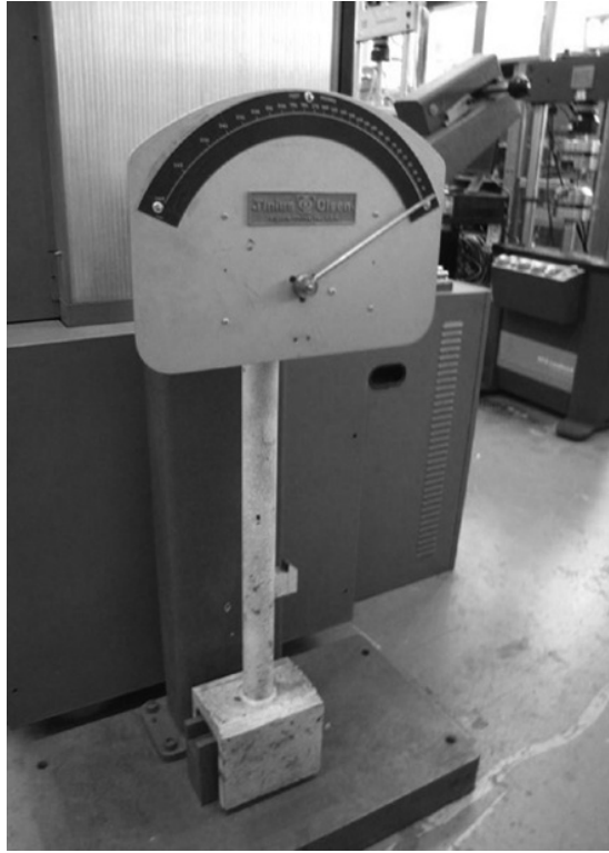
Figure 7.2 Impact test machine for assessing toughness
