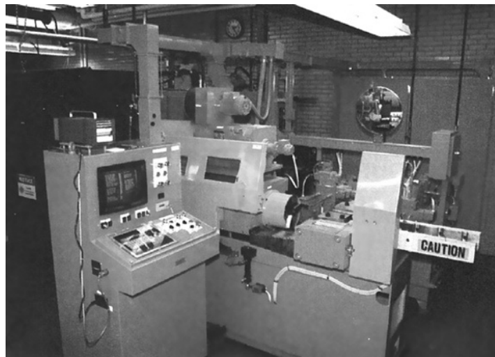
Figure 4.9 Continuous drive friction welding machine (Source: Reproduced by permission of American Welding Society, ©Welding Handbook)
