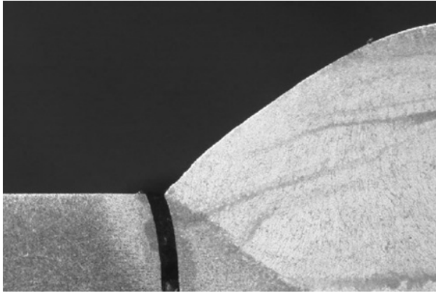
Figure 7.1 Typical location of a fatigue crack
