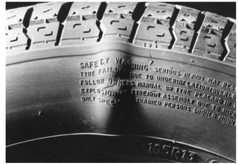
Bulge, due to kerb or pothole damage
