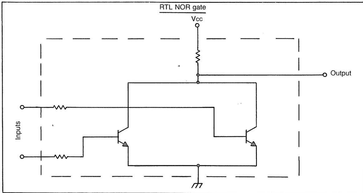
Fig. 7-4. RTL means Resistor-Transistor Logic and refers to the resistor inputs in the base circuits of the transistors.
