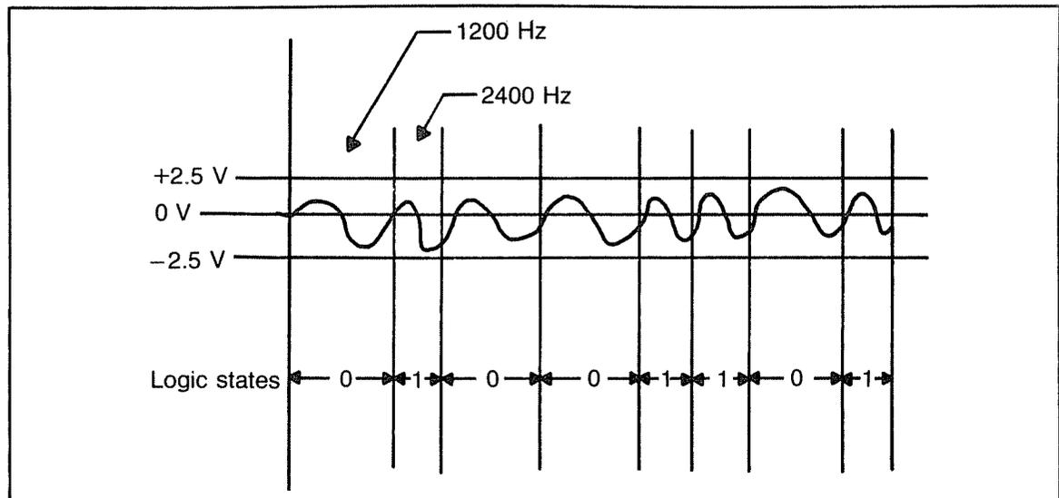
Fig. 19-3. The logic states must be coded into sinewaves before they are sent to the tape recorder. The code is a sinewave of  $1200\text{ Hz}$  to represent a 0 and  $2400\text{ Hz}$  to represent a 1.
