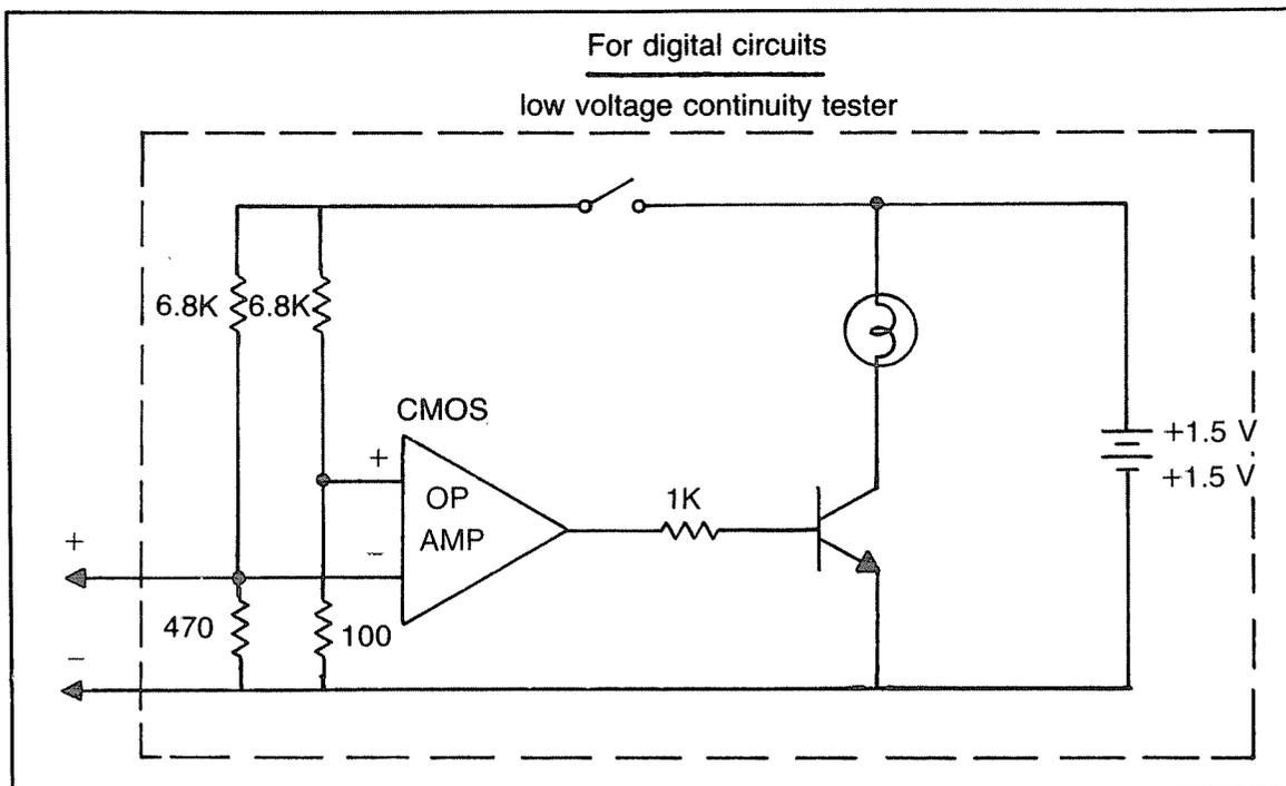
Fig. 14-7. This shows a commonly used continuity tester that digital technicians make for themselves with a few parts. Only  $\frac{1}{4}$  of a volt can reach the sensitive microscopic components on a chip, rather than 1.5-3 volts that the usual continuity tester or vom would apply.
