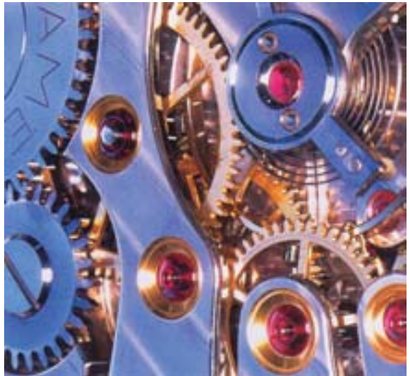
Gear trains inside a mechanical watch
