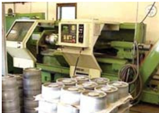
CNC lathe at a turning centre.
