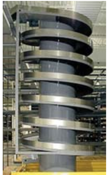
A spiral elevator conveyor for material handling.
