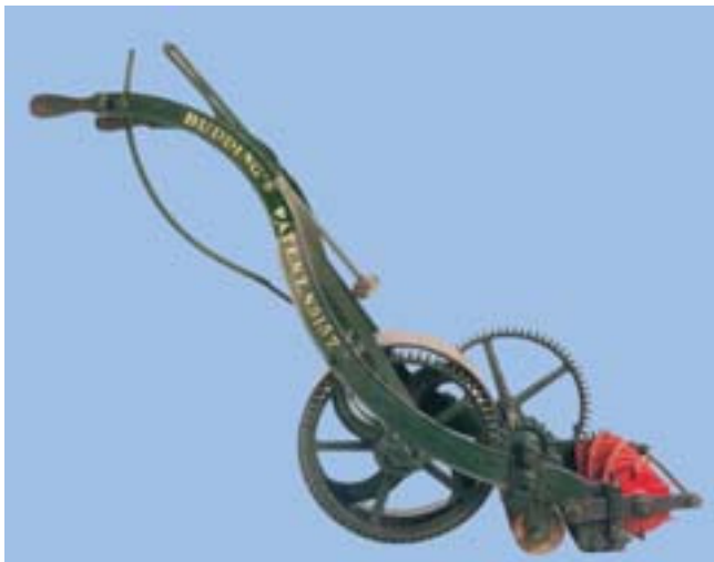
Lawn-mover is a combination of kinematic links.
