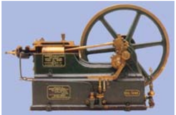
The above picture shows the reciprocating parts of a 19th century oil engine.
