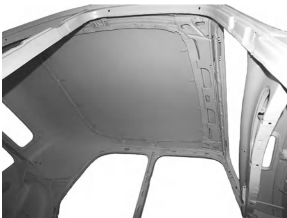
Fig. 2.14 Roof structure of the Citroën 11 CV unitized body (Picture taken at Rétromobile, Paris, 2009)
