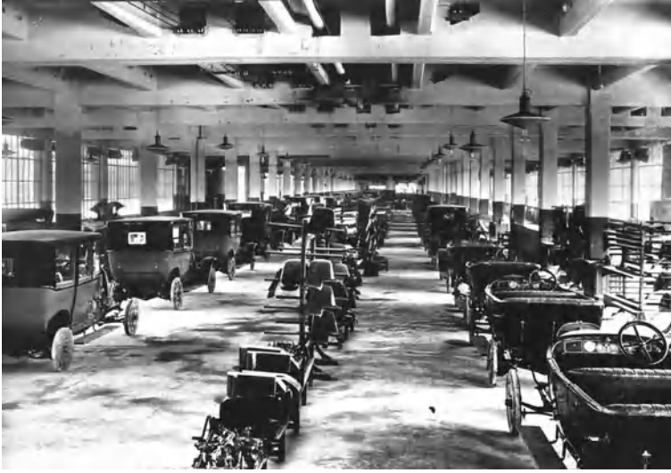
Fig. 5.3 Assembly line where all parts had to be adapted in place starting from raw materials, as cloth, leather, cables, pipes, etc (Courtesy of FIAT Historical Archives)
