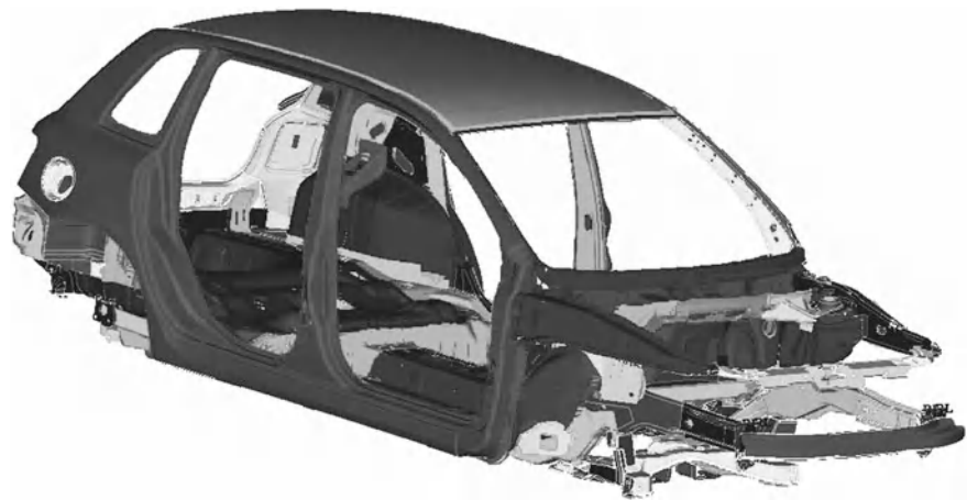
Fig. 8.11 A complete body-in-white (courtesy of Fiat)
