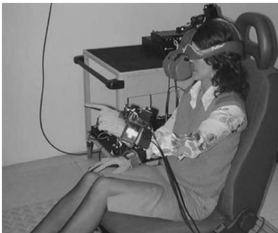
Fig. A.25 The user observes the virtual world (in this case the interior of a passenger compartment) through a helmet with a binocular display. The seat is a real physical prototype; controls are simulated by means of a haptic glove (from Morello et al. 2011)
