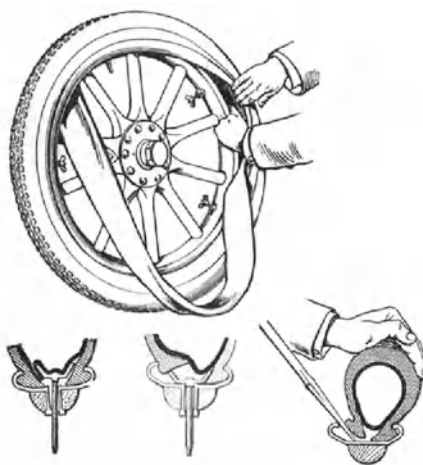
Fig. 3.34 In the 1917 Panhard & Levassor the one piece rim cannot be disassembled from the wheel. The figure on the right shows how tire and tube can be changed
