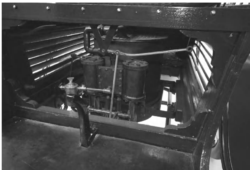
Fig. 4.63 The most important developments in the 1904 Stanley are the fast boiler and the distributor regulation of the propulsion system (National Automobile Museum of Torino)
