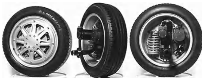
Fig. 16.4 The active wheel built by Michelin: a complete corner unit, provided with drive motor, brake, suspension and steering
