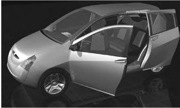
Fig. A.23 Virtual reality model of the exterior shape of a car obtained by CAD surface mathematical models (from Morello et al. 2011)
