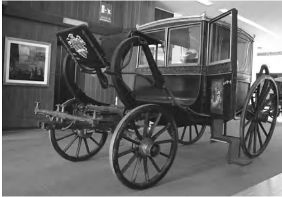
Fig. 3.1 This coach, built around 1650, shows a suspension made by four leaf springs and leader belts (National Automobile Museum of Torino)
