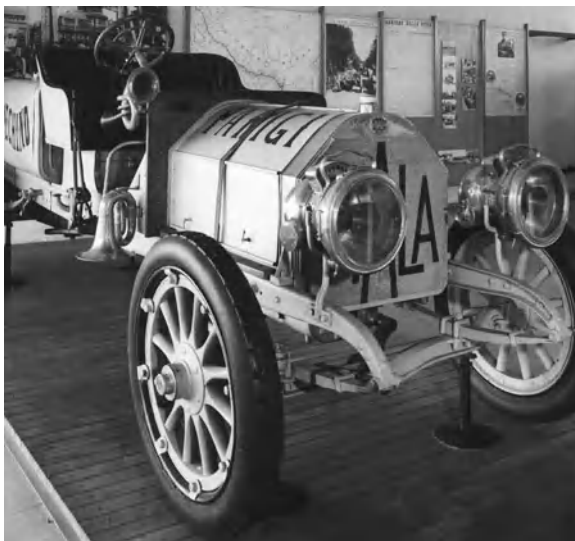
Fig. 3.33 In this car the rim can be disassembled in three parts; the tire can be removed without any deformation of the bead that can be, in this case, very massive and robust (National Automobile Museum of Torino)
