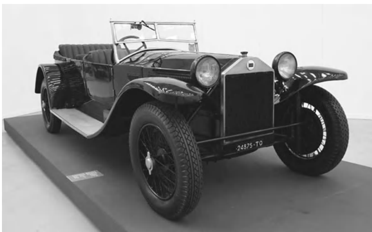
Fig. 2.12 The body of the 1922 Lancia Lambda was very low over the ground, thanks to the integration of the chassis function (National Automobile Museum of Torino)
