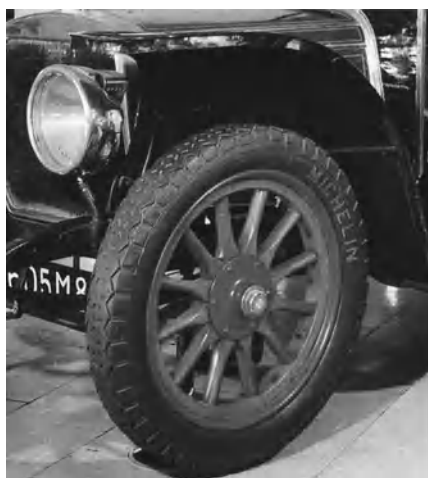
Fig. 3.34 In the 1917 Panhard & Levassor the one piece rim cannot be disassembled from the wheel. The figure on the right shows how tire and tube can be changed
