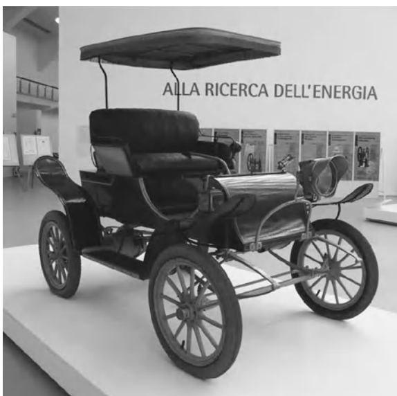
Fig. 4.58 Pope Model 1901; note the electric motor integral with the rear axle (National Automobile Museum of Torino)
