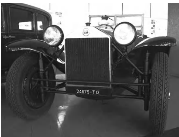
Fig. 3.13 The front view of the Lancia Lambda shows the front suspension and the gate structure of connection to the body (National Automobile Museum of Torino)
