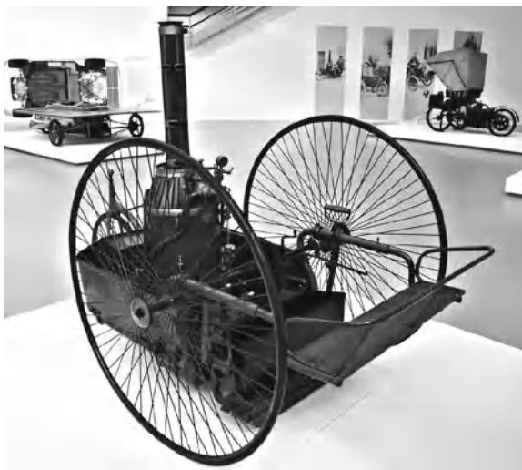
Fig. 4.60 In the 1891 Pecori steam car the position of the boiler allows the driver to feed the furnace (National Automobile Museum of Torino)
