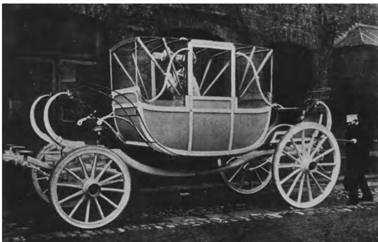
Fig. 2.5 Coach during the fabrication process, before exterior panels were assembled (from Morello et al. 2011)
