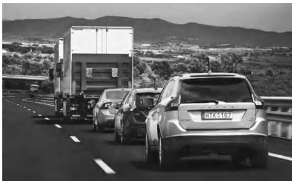
Fig. 15.1 A 'road train' made of vehicles that follow automatically a lead vehicle driven by a human driver. Picture from the SATRE project by Volvo
