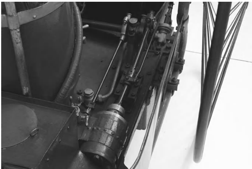
Fig. 4.61 One of the two engine cylinders acting on a transversal crankshaft; this drives directly the differential through a chain (National Automobile Museum of Torino)
