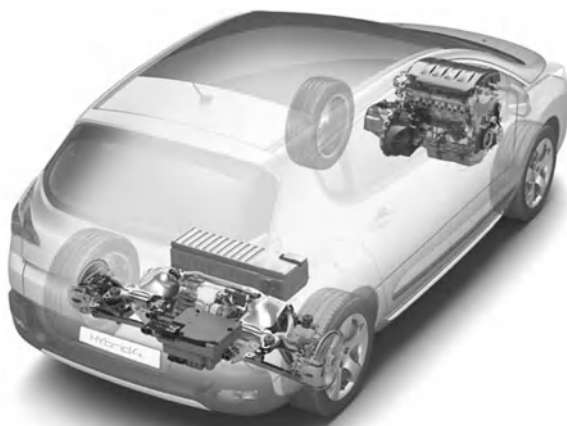
Fig. 12.9 The Peugeot 3,008 Hybrid 4 is the first hybrid car available with a diesel engine; it is a two-axis parallel hybrid system, in which the internal combustion engine works on the front wheels and the electric motor on the rear axle (courtesy of Peugeot)
