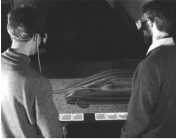
Fig. A.27 Virtual wind tunnel for scale model of a vehicle (from Morello et al. 2011)
