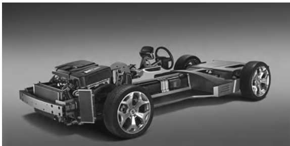
Fig. 12.11 The battery of the Opel Ampera is T-shaped; one branch of the T is along the floor tunnel while the other is across the car, under the rear seat (courtesy of Opel)
