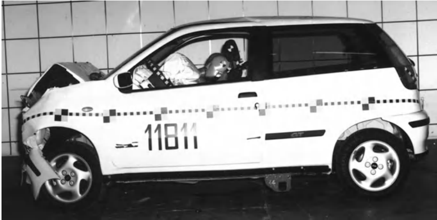
Fig. 8.6 The result of a crash test against a fixed barrier at 60km/h performed on a Fiat Uno (courtesy of Fiat)
