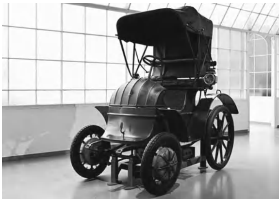
Fig. 12.7 The Lohner-Porsche Elektromobil was built in 1900 as a BEV, but was then converted into a hybrid vehicle
