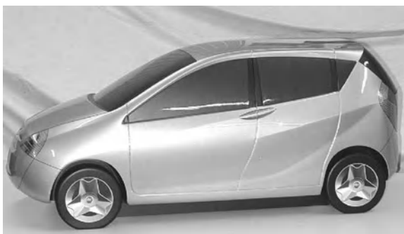
Fig. A.9 Milled surface cut from a sawdust and epoxy resin block, treated with plaster and paint, to simulate the final appearance (from Morello et al. 2011)
