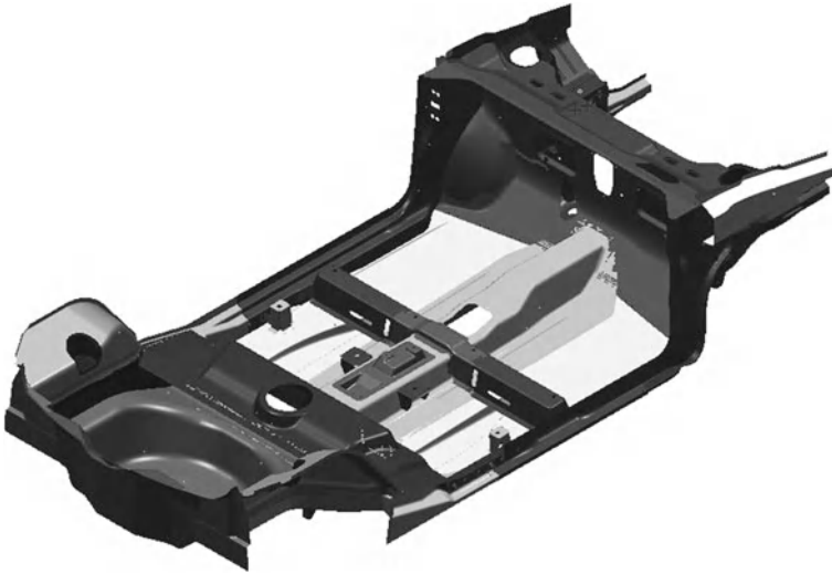
Fig. 8.3 A typical body frame for a unibody of present day configuration (courtesy of Fiat)
