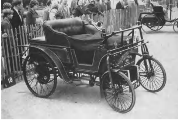
Fig. 3.11 The vertical telescopic independent suspension was probably introduced by Stephens in 1898 (from Genta and Morello 2009)
