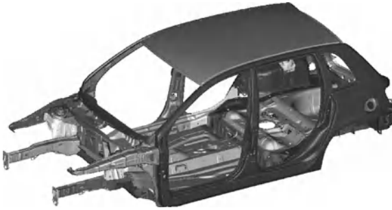
Fig. A.17 DMU of a complete body shell. This figure reproduces what displayed by a computer monitor, showing the product breakdown structure on the left, with the names and part numbers of each component or subassembly included in the model (from Morello et al. 2011).
