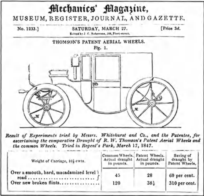
Fig. 3.28 The cover of Mechanics' Magazine reporting the results of a pull test performed on a coach on macadam and gravel ground. The application of tires reduces the traction effort noticeably
