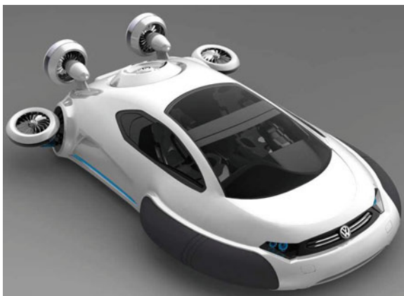
Fig. 16.8 Volkswagen Aqua, a hovercraft powered by hydrogen fuel cells that won a Volkswagen-sponsored design competition. Like for other futuristic vehicles, only a design or a mockup exists
