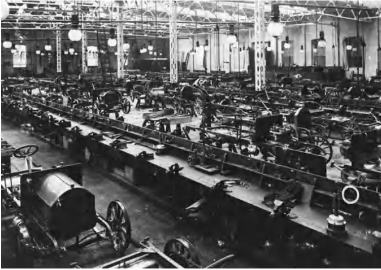
Fig. 5.2 In the assembling shop of that time, a number of benches equipped with vices were set close to each assembling post. Because the chip cutting process did not guarantee an immediate part matching with adequate clearance, parts had to be hand scrapped, verifying the fit by a trial and error procedure (Courtesy of FIAT Historical Archives)
