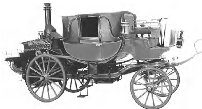
Fig. 3.2 The Bordino's steam coach was built in 1854. The suspension system is strictly derived from that of a horse carriage. The rear axle is shaped as a crankshaft, on which the connecting rods of the two cylinders operate directly (National Automobile Museum of Torino)
