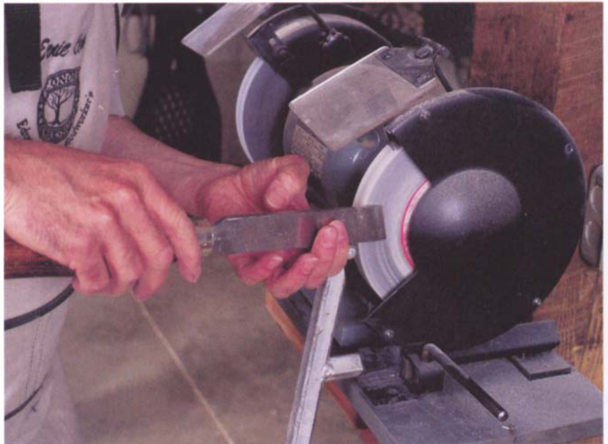
Grinding a skew on the side of a wheel is the only way to obtain a flat bevel. Grinder manufacturers don't recommend this, but it is safe if you use moderate pressure against a wheel that is \frac{1}{2} in. or wider.
