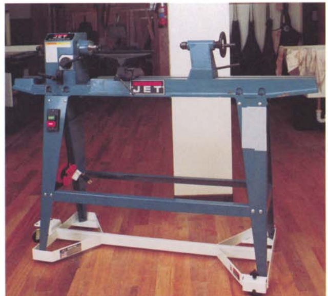
Based on the Delta 46-700, this Jet lathe is a good small lathe that offers good swing and between-center distances with a swing head for occasional larger faceplate work.
