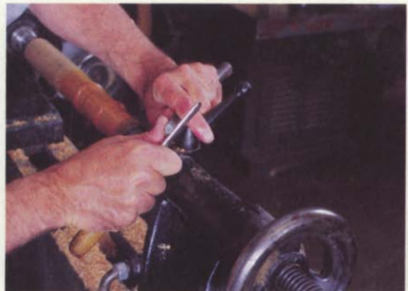
3 Use a cabinetmaker's burnisher to roll the edge. Considerable force is necessary, and a bit of wax helps in rolling the burr because it makes the burnish slide more easily. You may find clamping the tool in a vise helpful.
