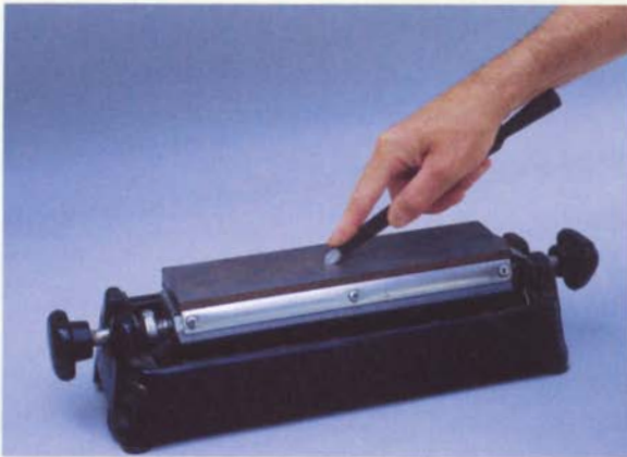
2 Use an oil stone to bring the bevel and back to a good finish.
