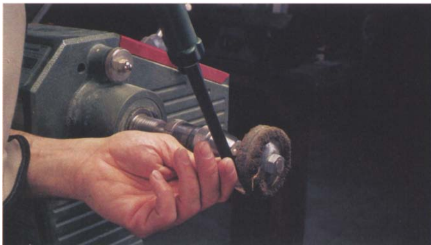
Mount the wheel and arbor in a drill chuck in the lathe.
