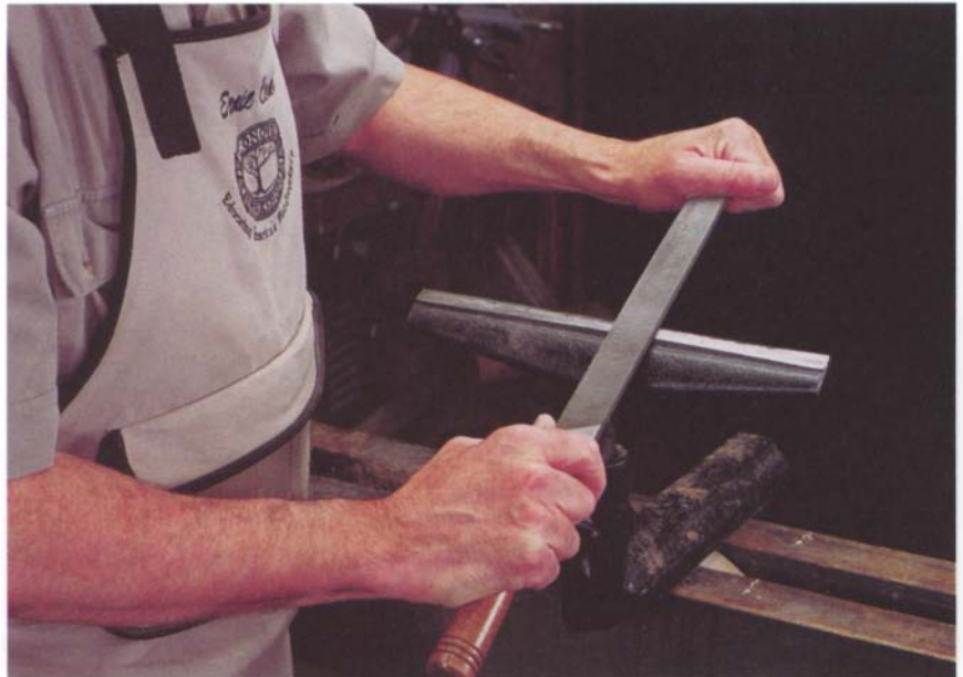
Draw-filing is the best way to redress a misshapen tool rest.
