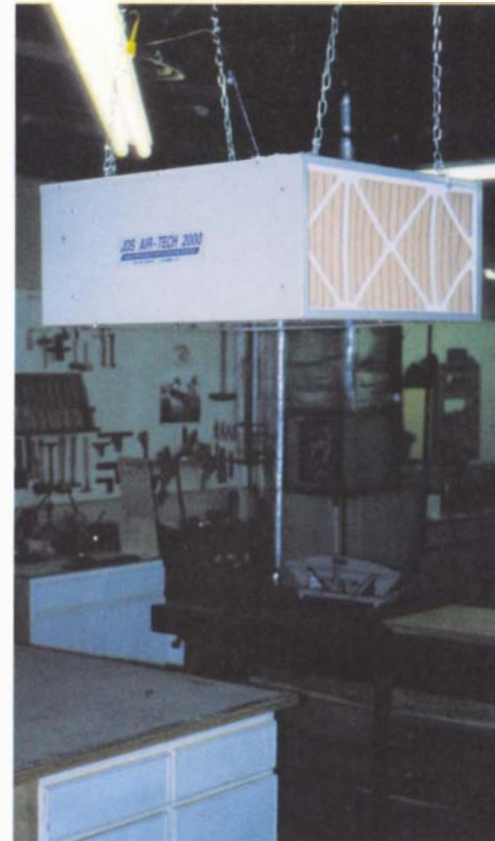
Air-filtration systems that continuously clean the air in your shop are a great second line of defense after a dust mask. They keep the shop cleaner as well. (Photo courtesy the JDS Company.)
