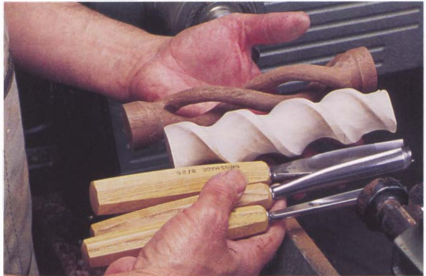
Here is a spiral column and a two-flute closed spiral of a tighter twist.
