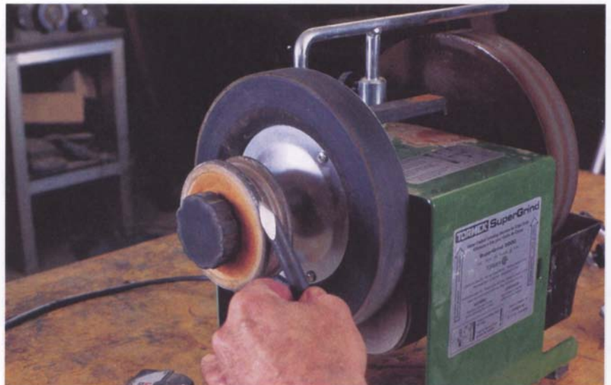
For the inside of gouges, the optional profile honing strop on a Tormek machine mounts outboard on the normal strop supplied with the machine.
