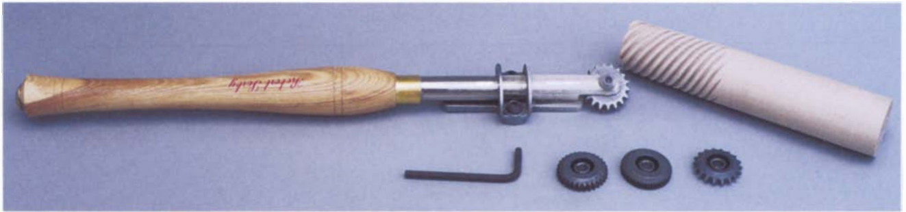
Sorby spiralling tools will cut multistart twists in spindles. The pitch of the spiral is controlled by how far the wheel is angled to the right or left.
