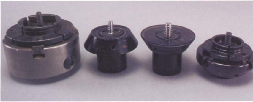
The scroll chuck shown on the left is a Oneway chuck, which has a screw included that turns it into a screw chuck. The two center screw chucks are by Jerry Glaser. On the right is a Nova lever scroll chuck with an included screw.
