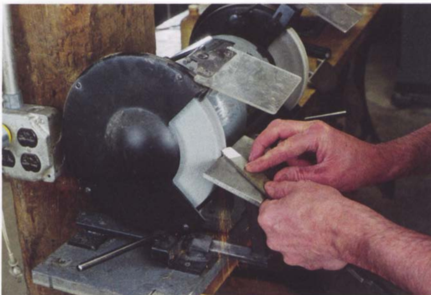
Grind to shape using your pattern as a guide. Everything should be undercut at least 5^\circ but no more than 15^\circ .
