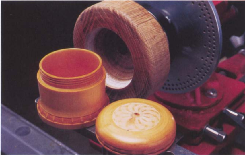
This screw-thread box (open) has a barleycorn pattern on the lid and side cutting on the lid and base.
