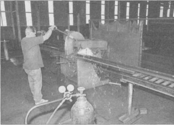
2.30 If you can't carry a 20-foot length of steel home with you, steel houses will generally make one "courtesy" cut for a small fee. Any cuts after that are expensive, so it's best if you have some method at home for cutting the metal for your projects.
