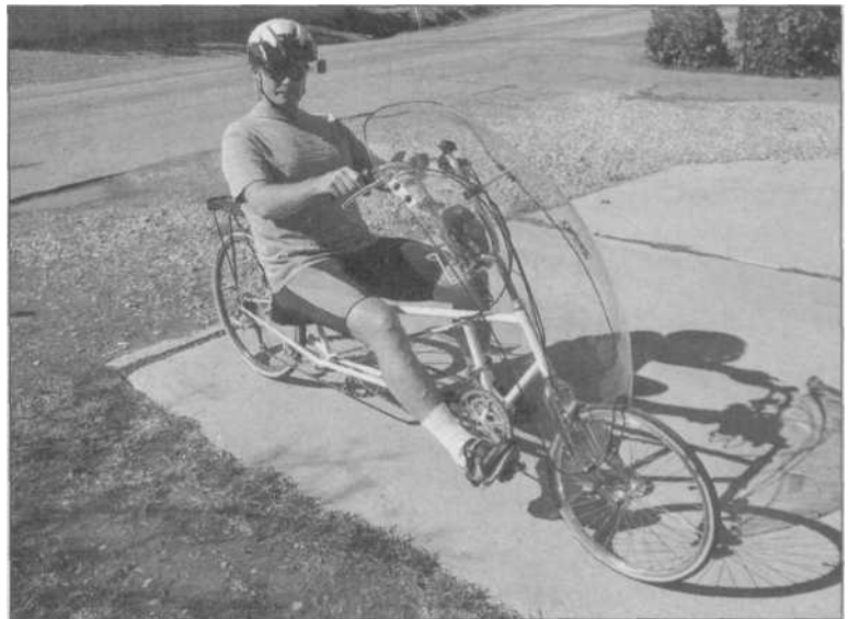
2.6 Weldor Bill Maguire fabricated this recumbent bicycle for himself from 4130 chrome-moly thinwall tubing, which is very strong but light. The idea was to reduce the bike weight, wind resistance and pedal effort. Bill joined the thin tubing with TIG welding.
