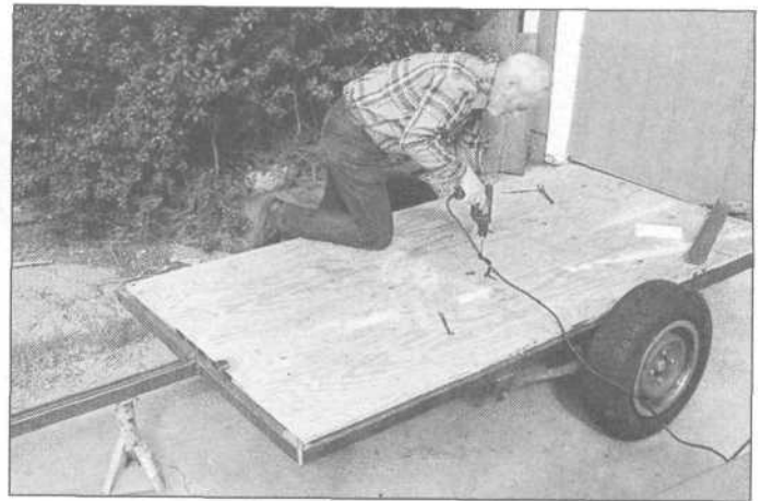
9.26 Locate where your tubes are and drill through the flooring and tubing, then bolt the floor down with carriage bolts, with the round heads on top so the floor is relatively smooth and a furniture dolly will go over the floor easily.
