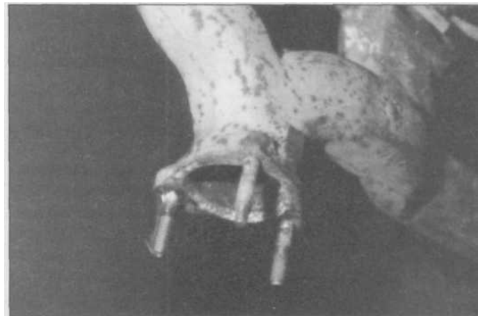
5.28 The new stud is now welded in place, with strength said to be up to 85% as good as original. This feature is a real time-saver for busy muffler businesses.
