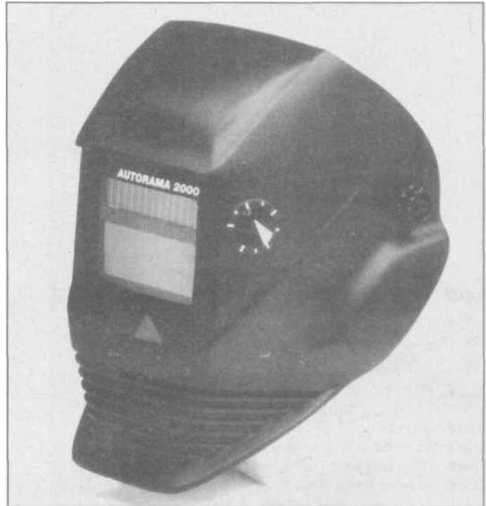
8.6 This Darth Vaderish design from ESAB is the Aurorama 2000, which one of a modern breed of welding helmet with an automatically-darkening lens. The lens is powered by solar cells, and turns dark as soon as the welding arc begins. These are considered by many weldors to be much easier to use than flipping a helmet up and down to set up each weld.
