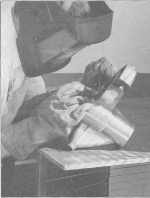
6.39 TIG welding is especially helpful in situations like this race-car suspension upright, where you have thin chrome-moly plate and tubing, and need total heat control. If you burn through on a job like this, the whole part may have to be scrapped.
