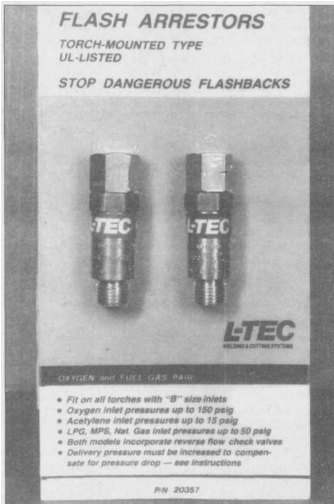
3.30 These prevent serious accidents from a flashback, indicated by a loud squealing noise. Flashbacks are caused by gasses burning inside the hose. For safety reasons, both hoses should be equipped with flash arrestors, which are reverse-flow check valves. Some readjustment of gauge pressures may be necessary when using check valves.
