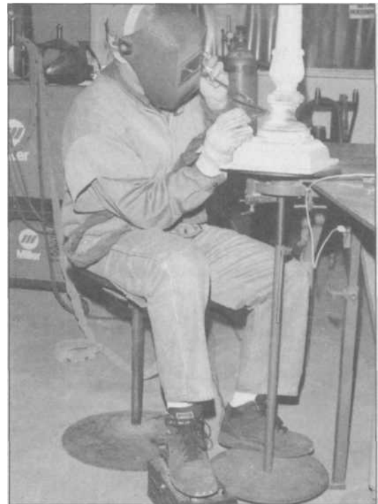
6.36 Welder Bill Maguire is TIG-welding the heated mailbox post, using his rotating welding stand he invented. At the bottom is a round disc you can spin with your foot, leaving your hands free to continue welding, especially where you have to go around something. These should be available for sale at the time of printing.
