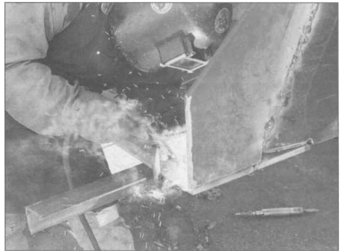
4.1 Arc welding will always be with us, as the best welding method for joining heavy plates for commercial, farm and industrial work. The weldor requires considerable protection from the spatter and radiation, usually wearing heavy leather protective gear.
