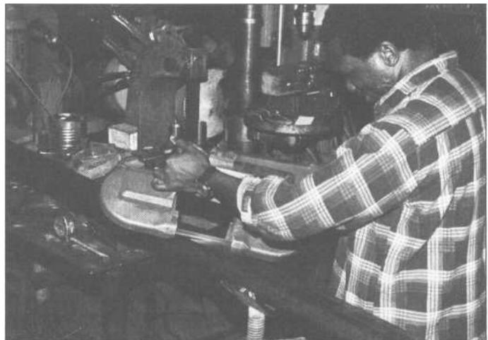
9.14 You can cut tubing and angle-stock with a hacksaw, but it is tedious. We borrowed a Milwaukee Port-A-Band hand-held bandsaw that made short, accurate work of fitting our tubing.
