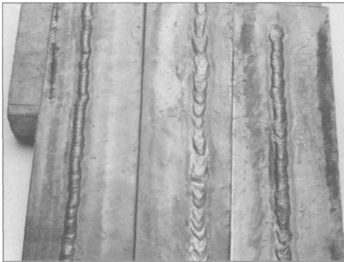
3.25 Heat in gas welding is controlled by matching the gas flow and tip size to the thickness of material. Your welding travel speed and tip-to-work distance will control the puddle size and penetration. With all things right, you should be able to heat your first puddle molten in about six seconds, then move along to make your bead. At left is a bead run too cold (bead stands up), at center is one run too hot and too fast, and at right is a better bead with good width and penetration.
