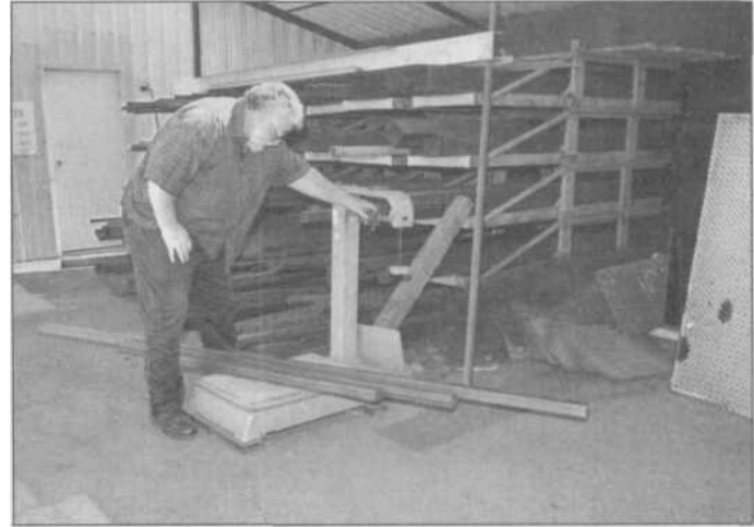
2.8 The welding supply store should be able to tell you where to buy steel locally, which you will probably use for most of your welding projects. Most yards have a remnant section as shown, where you can buy short lengths of material at by-the-pound prices. Tubing for a trailer project is being weighed.
