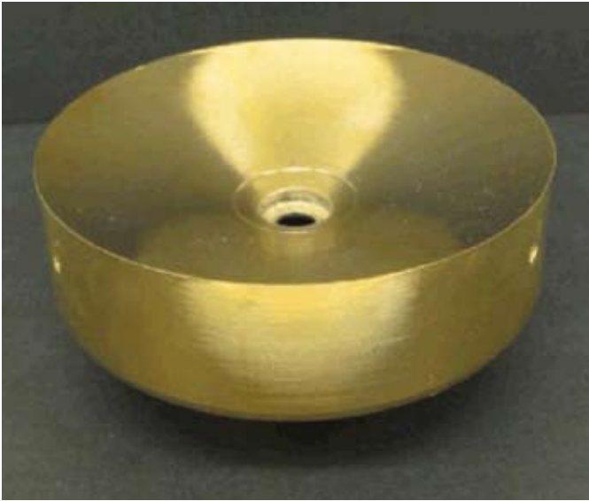
Figure 2. Rotating spinning disc manufactured from gold plated aluminum. Disc diameter is 100 mm.
