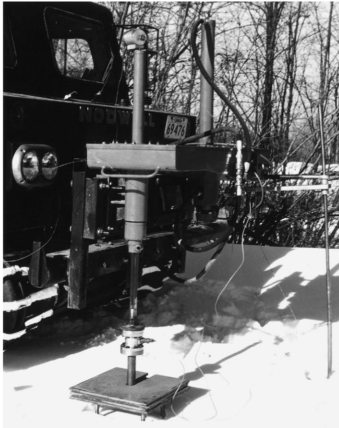
Figure 3.4: Shear tests using a vehicle-mounted bevameter
