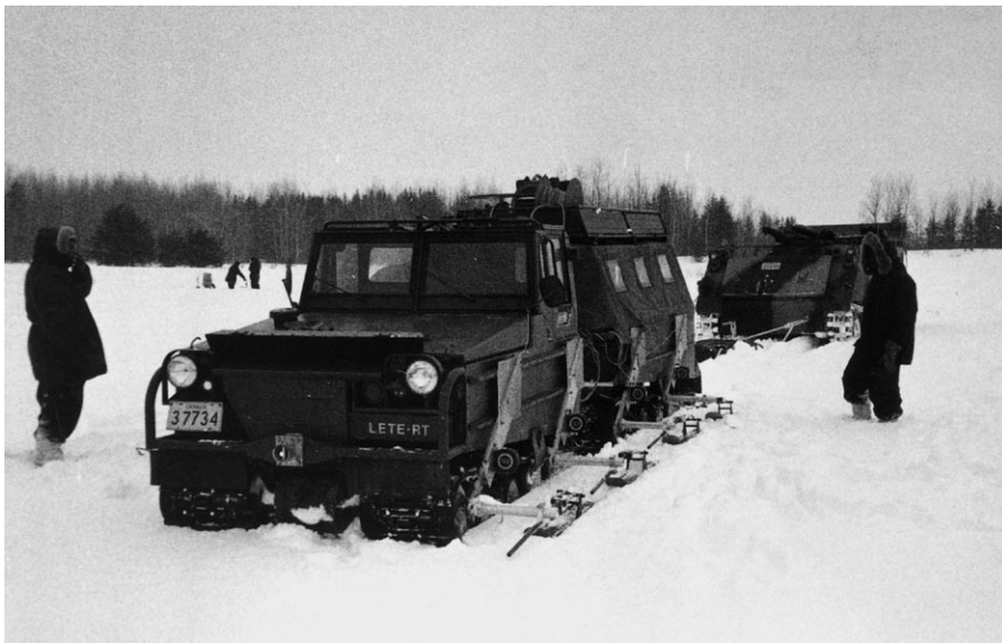
Figure 8.8: Instrumented Bv202 used in field tests
