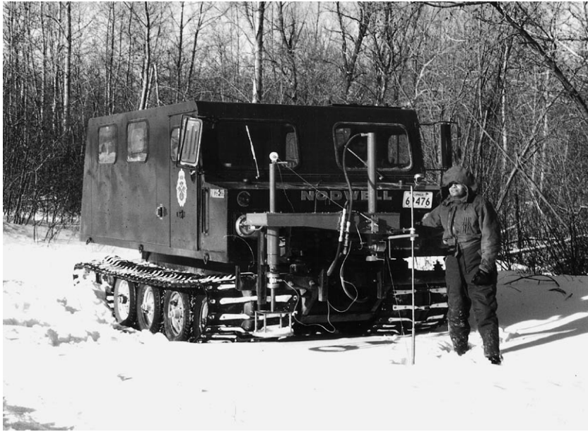
Figure 1.8: A vehicle-mounted beavometer for measuring terrain properties in the field
