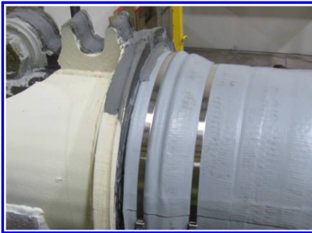
Figure 4. Mock-up for cable band sealing and cable wrapping.
