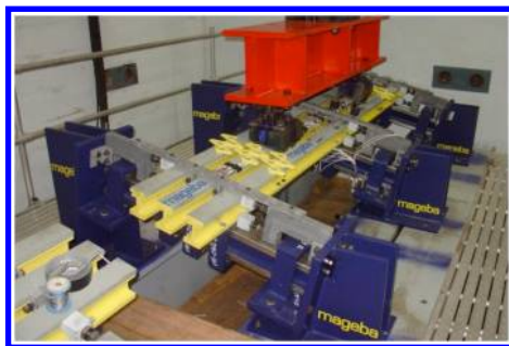
Figure 8. Fatigue testing of Tensa-Modular joint – one specimen.
