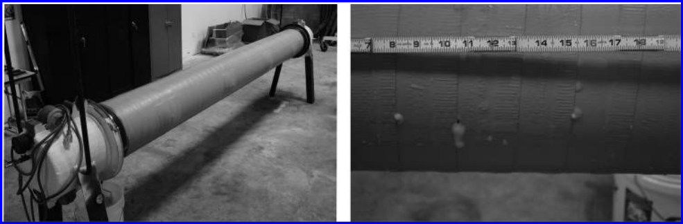
Figure 16. Test rig for wrapping demonstration (left); pressure test on test rig – soap bubbles indicate leaks in wrapping (right).
