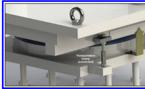
Figure 12. A disc bearing with the transport fixation in locked position.
