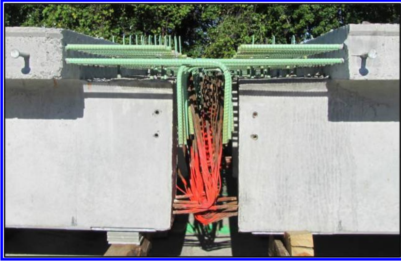
Figure 8. Continuity connection with extended strands.
