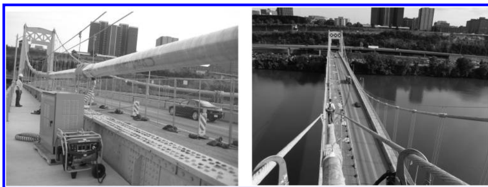
Figure 14. Flow trials on Philip Murray Bridge – temporary blower installed at mid main-span (left); view of main cable (right).
