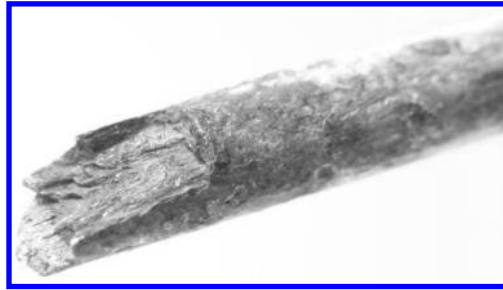
Figure 5. Wire fracture due to corrosion.
