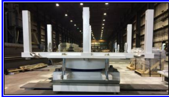
Figure 8. Disc bearing equipped with shim plate and adjustable presetting lugs ( Ohio River Bridge, Kentucky & Indiana ).
