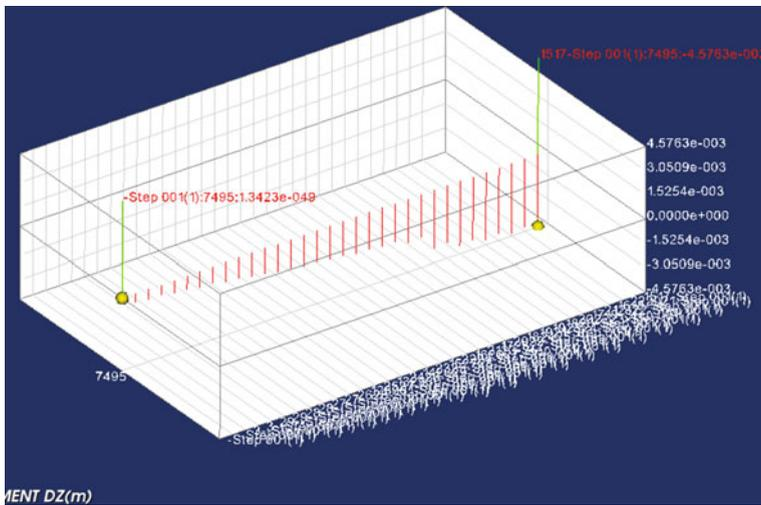
Fig. 4.15 Ground subsidence after excavation
