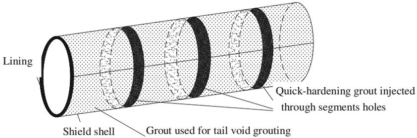
Fig. 2.36 Stability of hinged segments in weak strata
