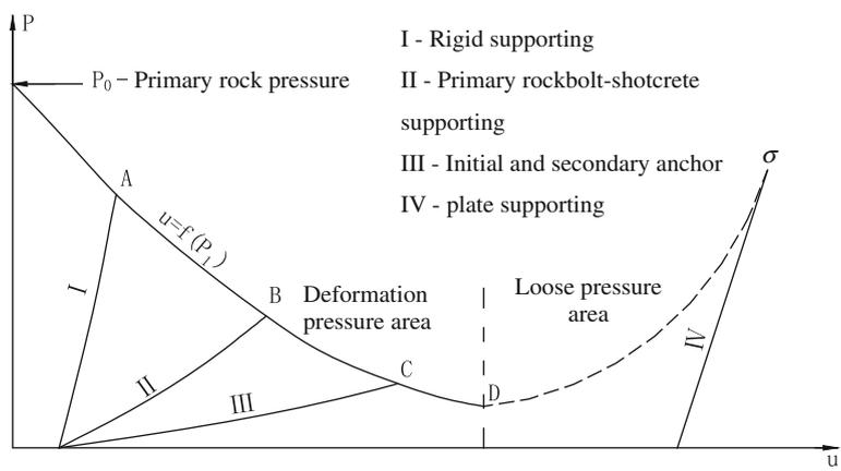
Fig. 1.6 Surrounding rock displacement supporting characteristics curve
