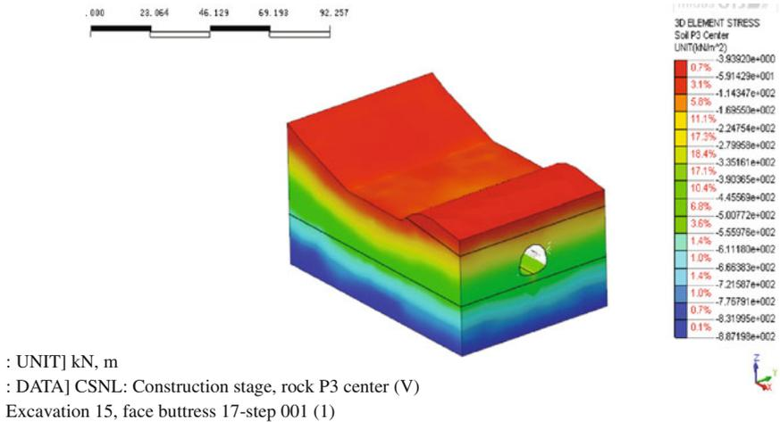
**Fig. 4.16** Contour plot of major principal stress after excavation
