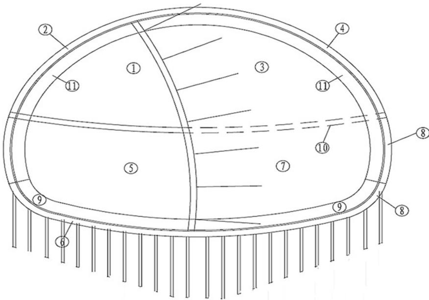
Fig. 3.7 Reinforcement of the tunnel base
