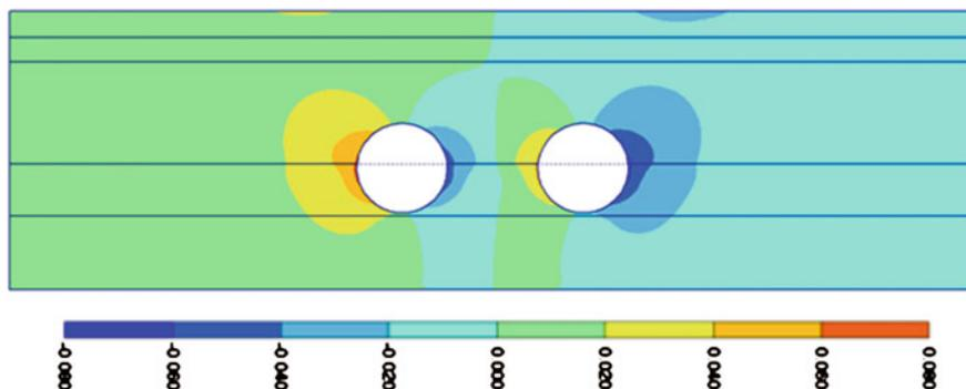
Fig. 5.15 Total displacement of the model after excavation of both lines
