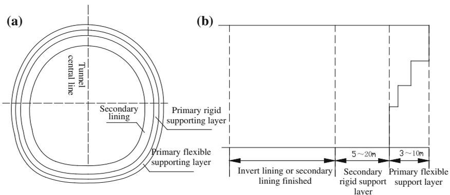
Fig. 2.16 Schematic diagram for construction and lining of class IV surrounding rock
