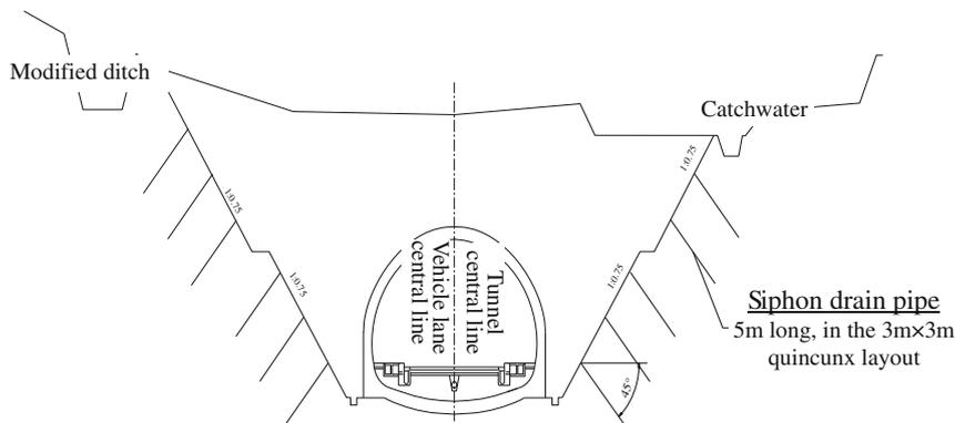
**Fig. 3.4** Drainage plan for the side slope of open cut sections
