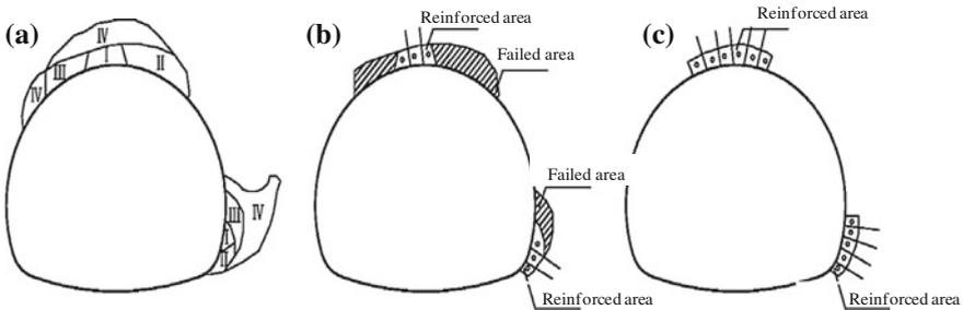
**Fig. 2.31** Evolution of space stability of mountain tunnels during excavation and supporting under general geological conditions
