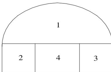
**Fig. 2.3** Construction order with hard bench
