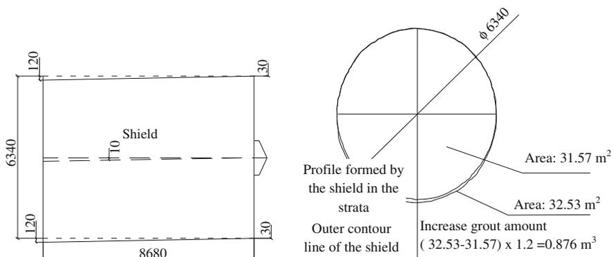
**Fig. 5.5** Illustration of relation between real posture and design construction parameters for 7# shield (all dimensions in mm)
