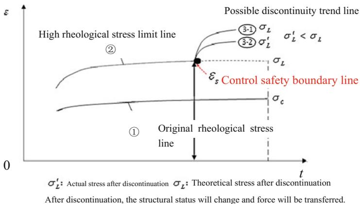
**Fig. 1.10** Characteristic diagram of control of discontinuity and conditional utilization of high rheological stress limit of rock/soil mass
