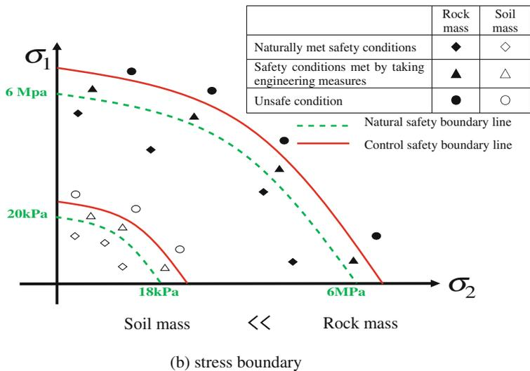
**Fig. 1.7** Safety boundary line for underground structures control in rock/soil mass (a) strain boundary (b) stress boundary
