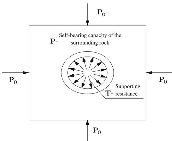
The surrounding rock pre-reinforcement force  $F$  equals to the bearing capacity of the “surrounding rock-supporting” structure system, i.e.
