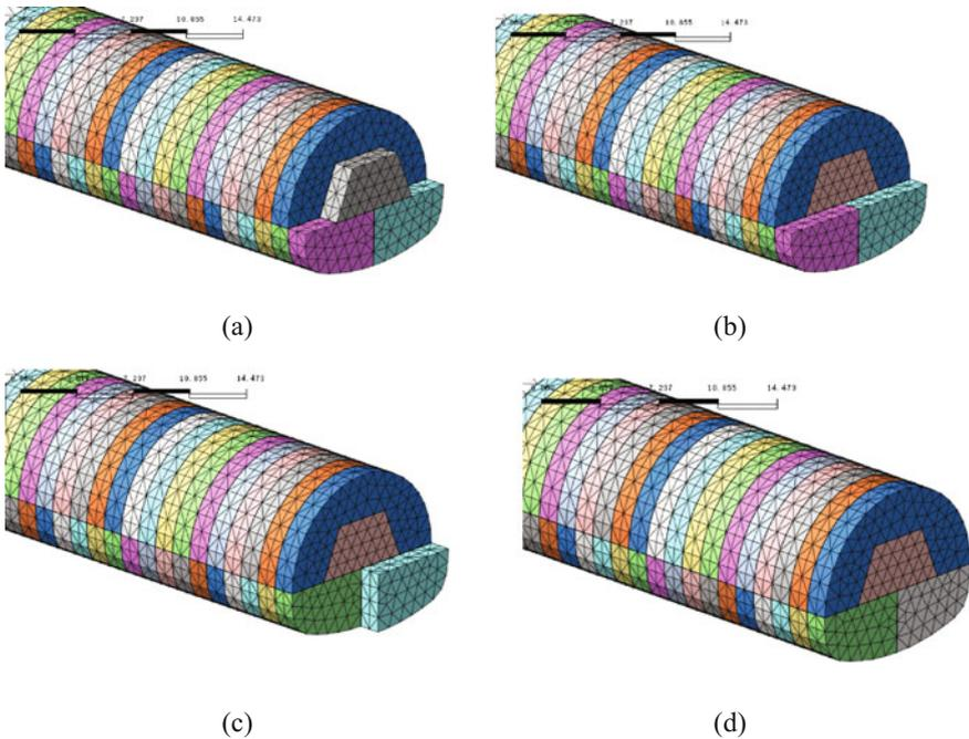
**Fig. 4.13** Simulation of excavation sequences
