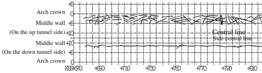
Fig. 2.21 Crack distribution diagram
