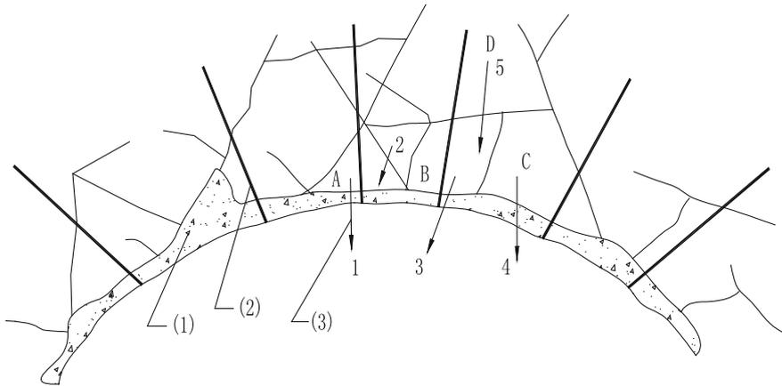
**Fig. 2.10** Schematic diagram of anchor-shotcrete supporting technique for blocky surrounding rock. (1) Shotcrete; (2) rockbolt; (3) potential collapse direction of the block; the potential collapsing order of blocks is 1, 2, 3, 4, and 5
