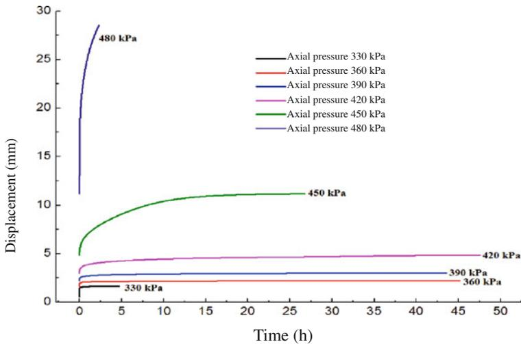
Fig. 3.9 Deformation response of soft soil to different axial stress
