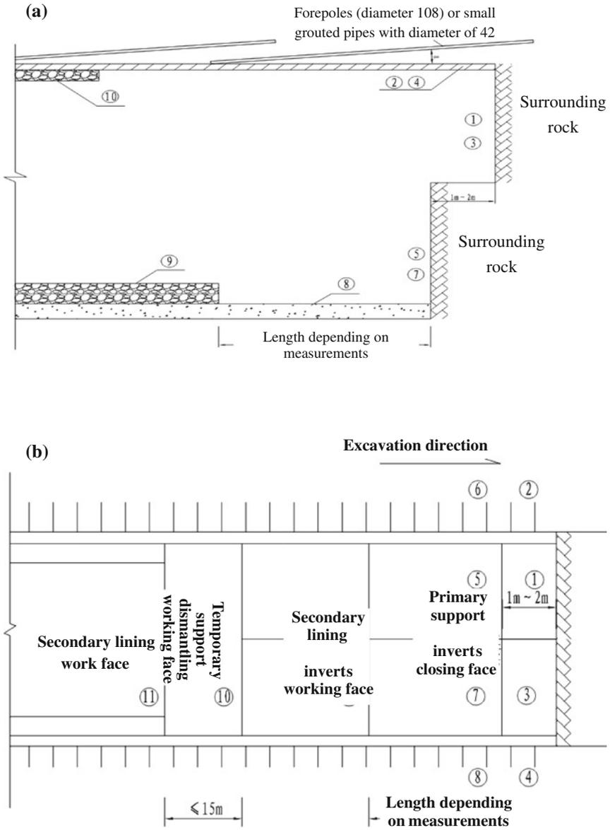
Fig. 3.5 Sequences of longitudinal excavation
