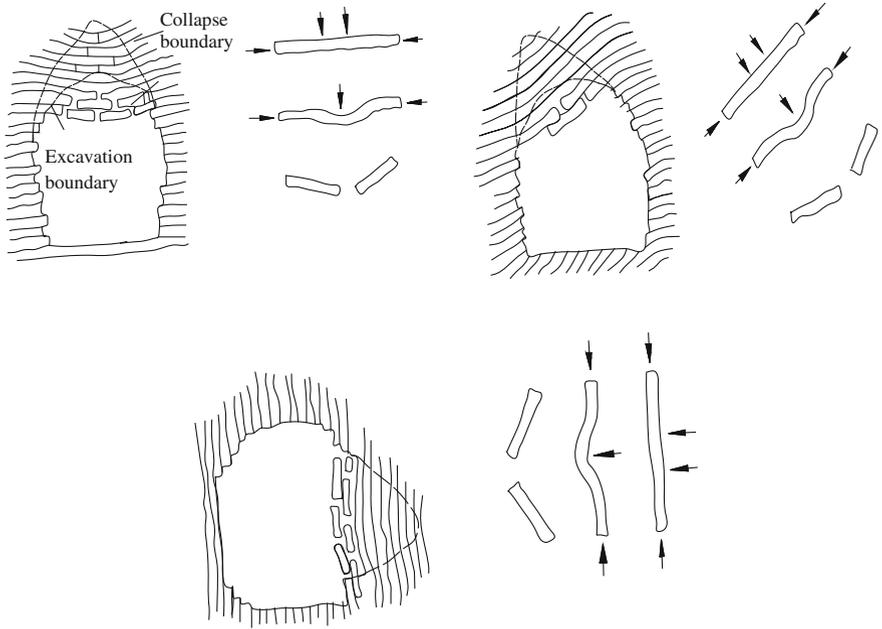
Fig. 2.11 Instability forms of stratified rock mass
