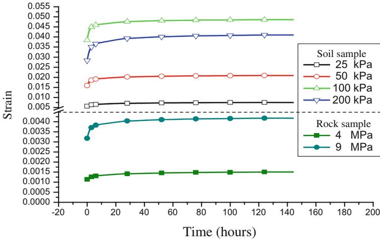
**Fig. 1.9** Rheological mechanics characteristics of rock/soil mass
