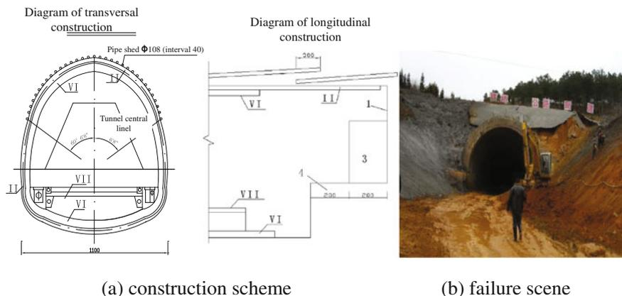
Fig. 4.3 Failure of shallow-buried tunnel construction scheme
