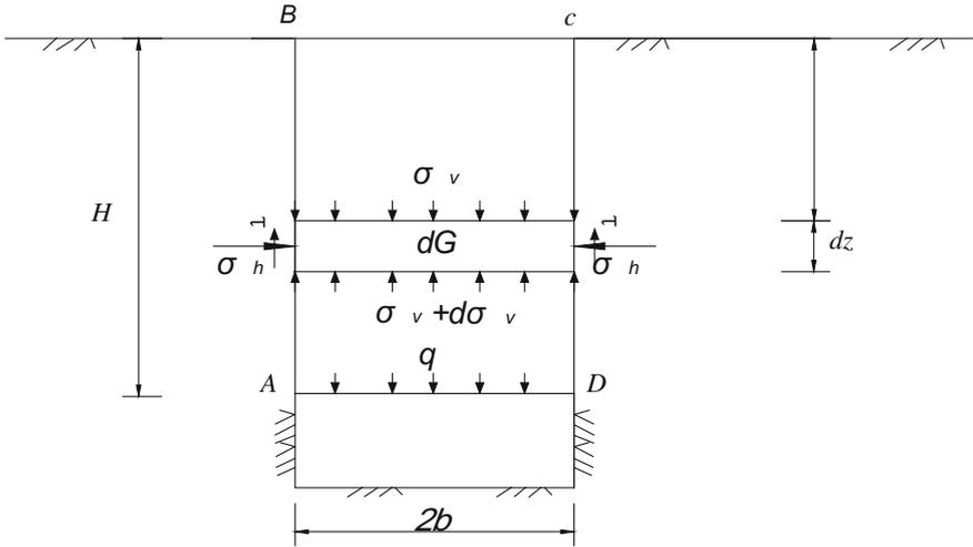
Fig. 1.4 Calculating chart of surrounding rock pressure with stable side walls
