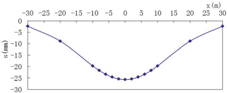
**Fig. 5.12** Horizontal subsidence of the stone embankment constructed in Ming and Qing dynasties
