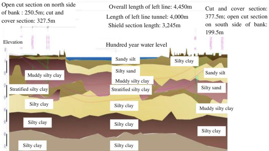
**Fig. 5.9** Schematic geological profile for Qianjiang tunnel
