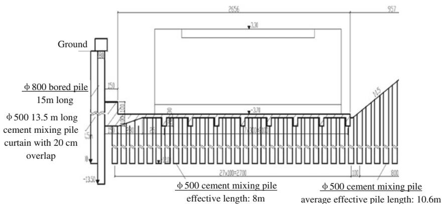
**Fig. 6.2** Design diagram of foundation retaining structure (all dimensions in cm except elevation)
