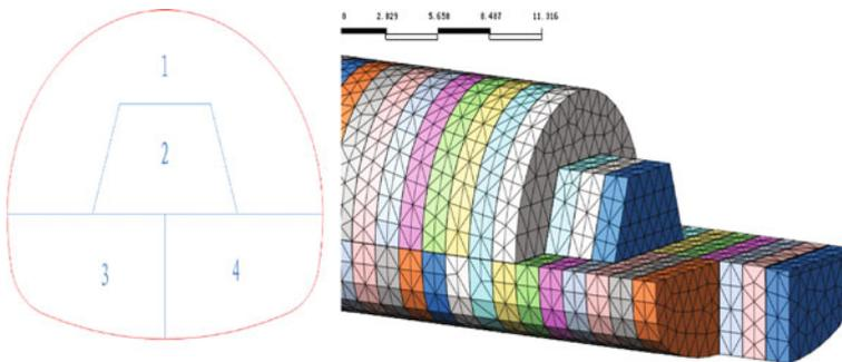
**Fig. 4.18** Numerical simulation for alternative scheme of highway tunnel excavation method
