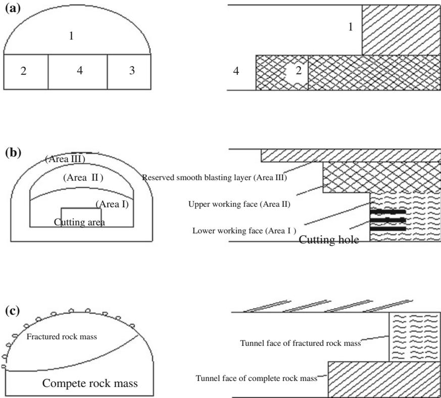
**Fig. 2.4** Schematic diagram of blasting excavation method. **a** Surrounding rock with soft upper part and hard lower part; **b** relatively hard surrounding rock; **c** half-soil half-rock surrounding rock
