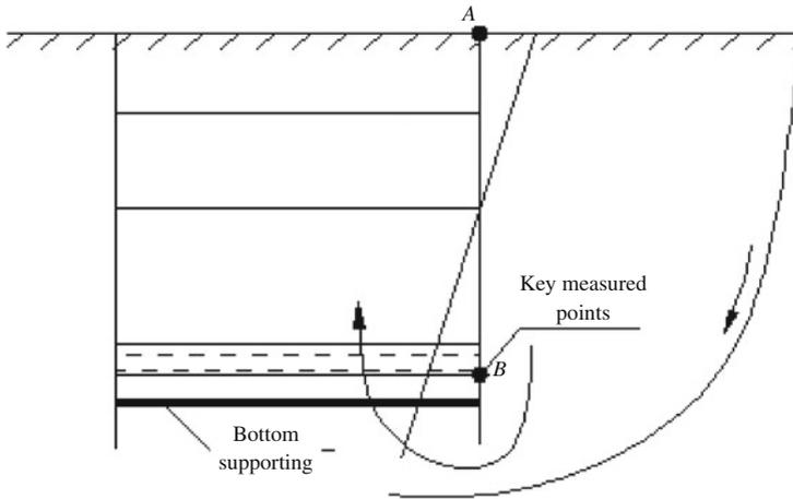
**Fig. 6.7** Schematic mechanism of deep foundation pit instability
