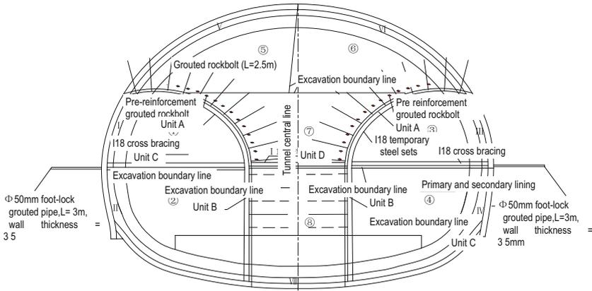
(a) Cross section drawing for construction
