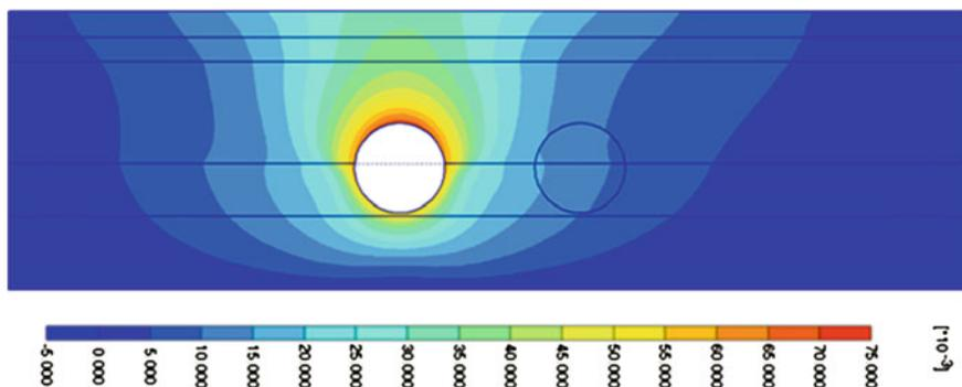
Fig. 5.14 Displacement contour of after excavation of west line
