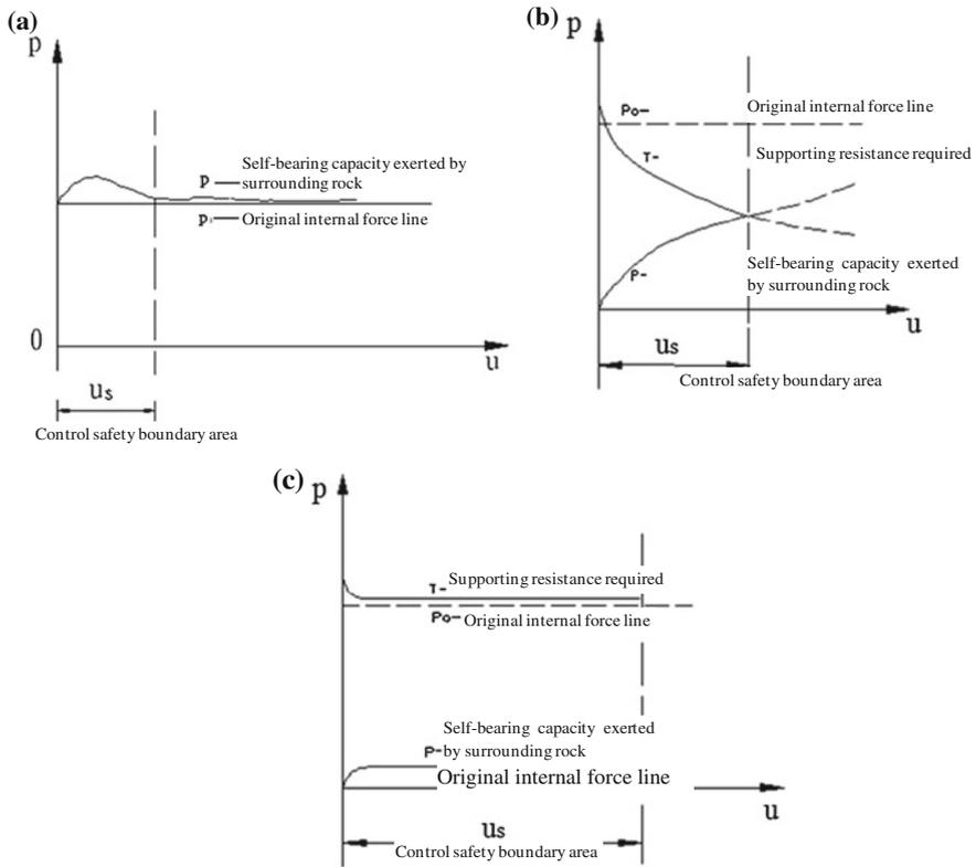
**Fig. 1.13** Three examples of force-displacement characteristic curve of underground engineering stable equilibrium theory (a) intact surrounding rock; (b) surrounding rock with fair self-bearing capacity; (c) surrounding rock with poor self-bearing capacity
