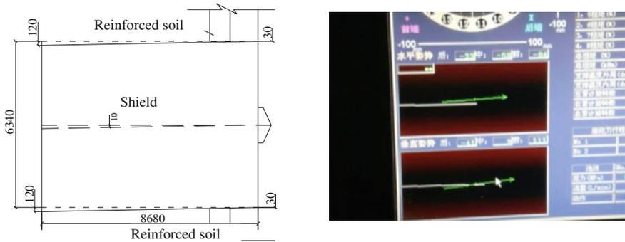
**Fig. 5.6** Postures of 7# shield in the reinforced soil (all dimensions in mm)
