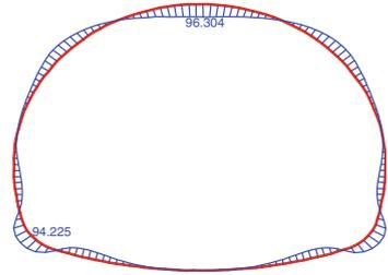
**Fig. 4.10** Displacement of primary support
