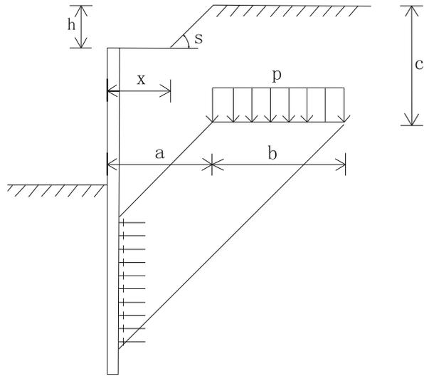
The foundation pit excavation should be carried out layer by layers and blocks by blocks in a good order. Supports should be provided in time; monitoring was required. For appearance of support axial force, structural deformation, foundation pit upheaval and ground surface subsidence, as well as misplace of diaphragm wall joint, water leakage and irregular underground water level, emergency measures should be taken according to the emergency plan.
