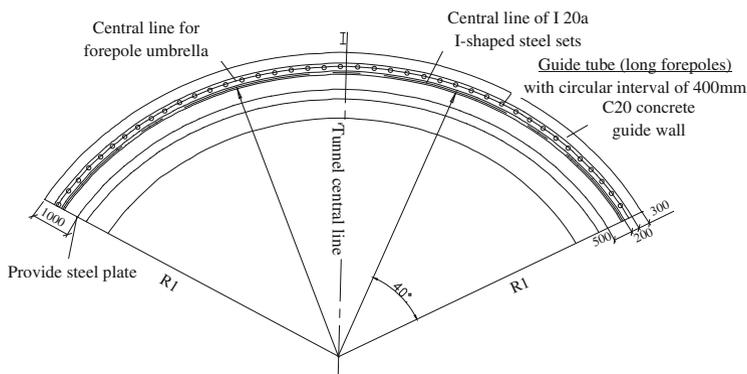
Fig. 4.4 Forepole umbrella support for railway tunnel
