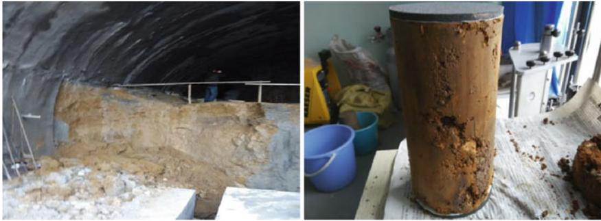
Fig. 3.8 Sampling location and prepared specimen
