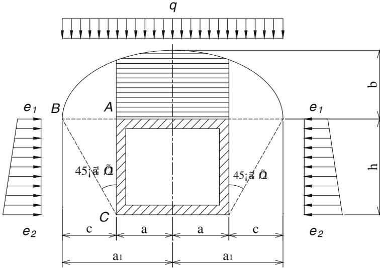
Fig. 1.3 Theoretical calculation chart of pressure arch
