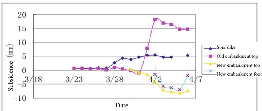
**Fig. 5.16** Subsidence during shield advancing in north embankment
