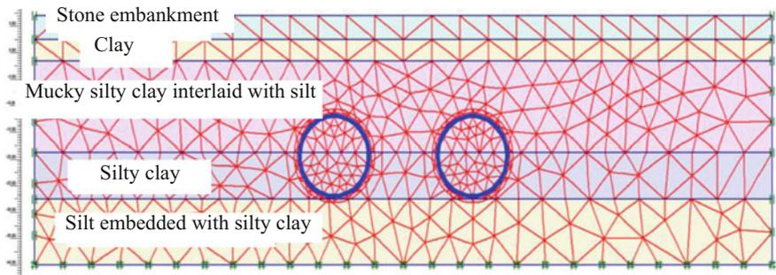
**Fig. 5.13** Elements of shield tunnel simulation model (stone embankment built in Ming and Qing dynasties)
