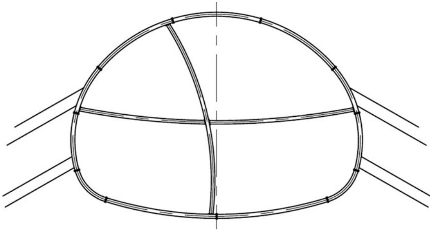
Fig. 3.6 Structural diagram of steel sets
