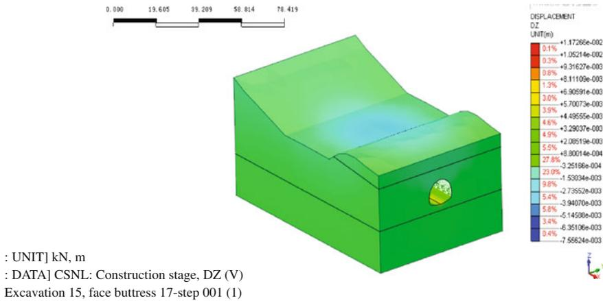
Fig. 4.14 Contour plot of vertical deformation
