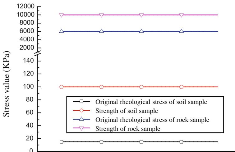
**Fig. 1.8** Comparison between original rheological stress and strength value of rock/soil mass
