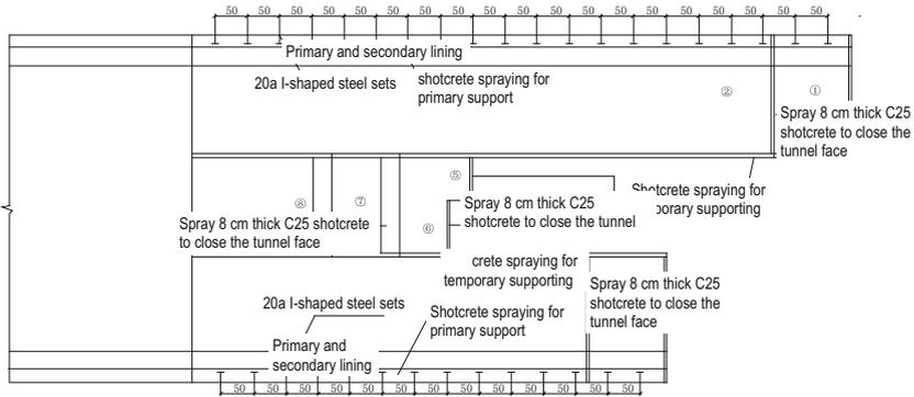
(b) Horizontal section drawing for construction
