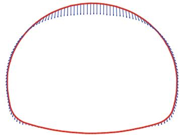
was provided within 100° of the roof; the grouted rockbolts of 4.0 m  $\Phi$ 25.5 were provided on sidewalls, at a circular space of 1.0 m.
