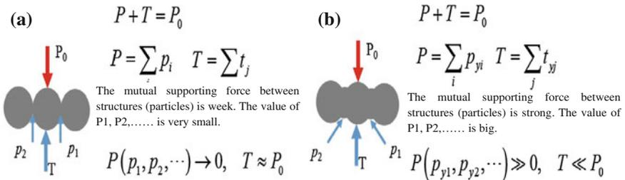
**Fig. 1.1** Schematic diagram for the engineering mechanics equation
