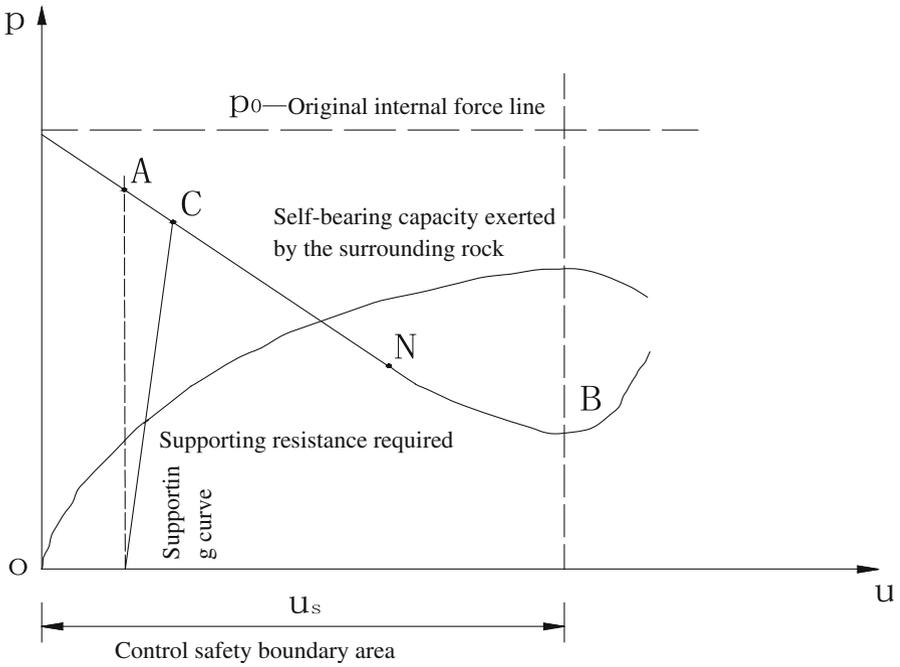
**Fig. 1.12** Force-displacement characteristic curve graph of underground engineering equilibrium stability theory
