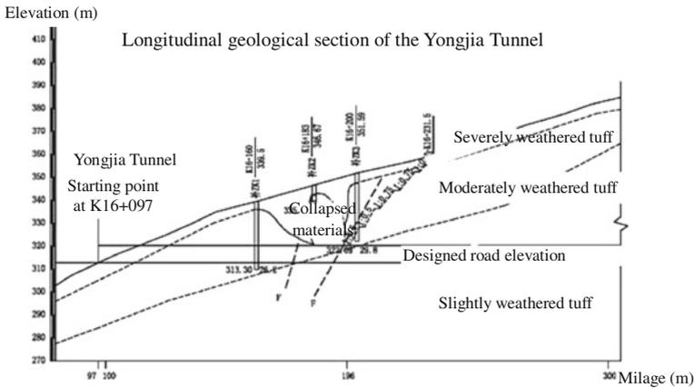
Fig. 2.32 Sudden collapse of about 2,420 m<sup>3</sup> in Yongjia Tunnel during excavation
