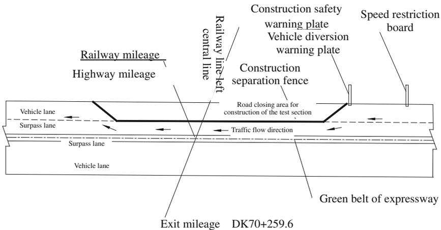
**Fig. 4.6** Traffic organization chart for the expressway during railway tunnel construction
