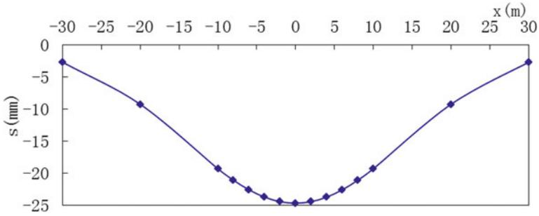
**Fig. 5.11** Horizontal subsidence of soil ridge embankment top on the north bank of the Qiantang river
