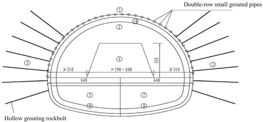
**Fig. 4.17** Alternative scheme for excavation and supporting of the highway tunnel
