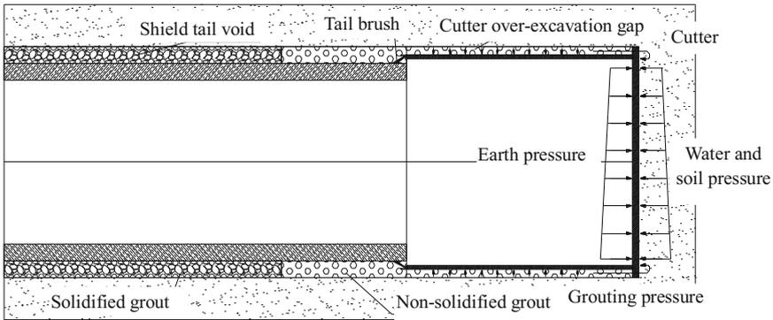
**Fig. 2.33** Schematic diagram of shield tail void and grouting
