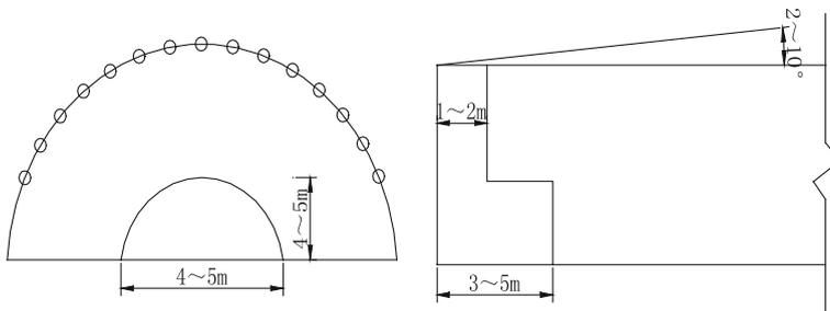
**Fig. 2.15** Schematic diagram for appropriate full-face excavation with pre-reinforcement and lower pilot tunnel ahead
