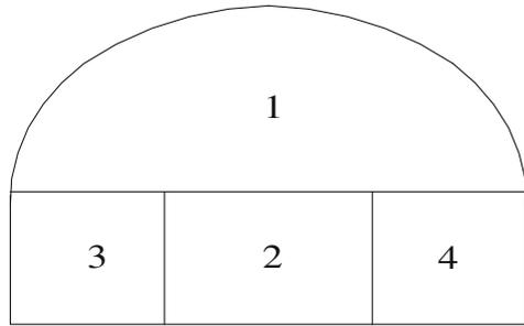
the two sides will be subjected to strong clamping effect in the horizontal direction. As the rock is hard, it takes strong blasting energy to break the rock mass, which requires high energy consumption and causes more obvious disturbance to the surrounding rock.
