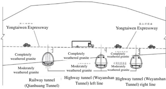
(a) cross section of the railway/highway tunnels
