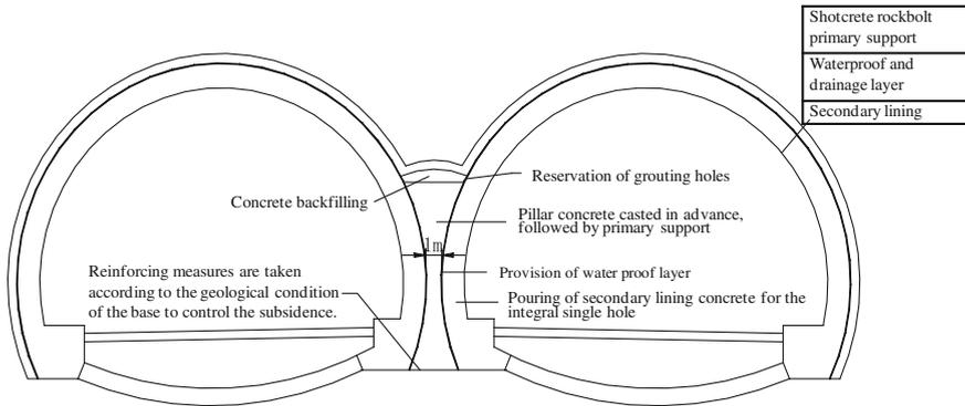
Fig. 2.23 Schematic diagram of improved section
