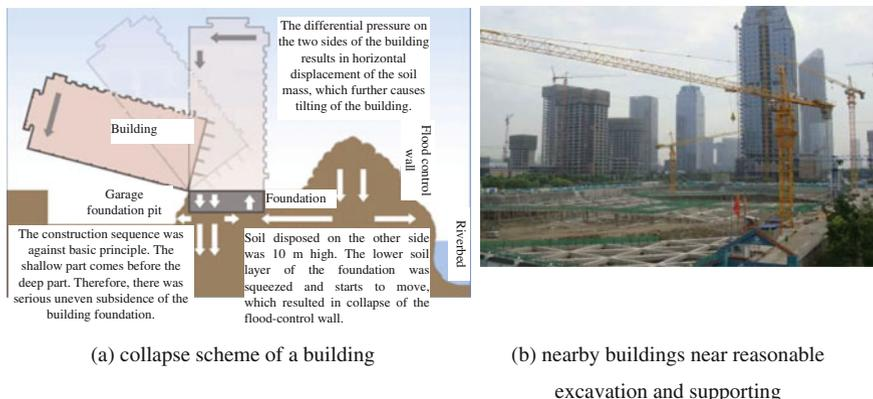
**Fig. 6.1** Building collapse caused by bad excavation of foundation pit and stability of nearby building guaranteed by reasonable excavation and supporting
