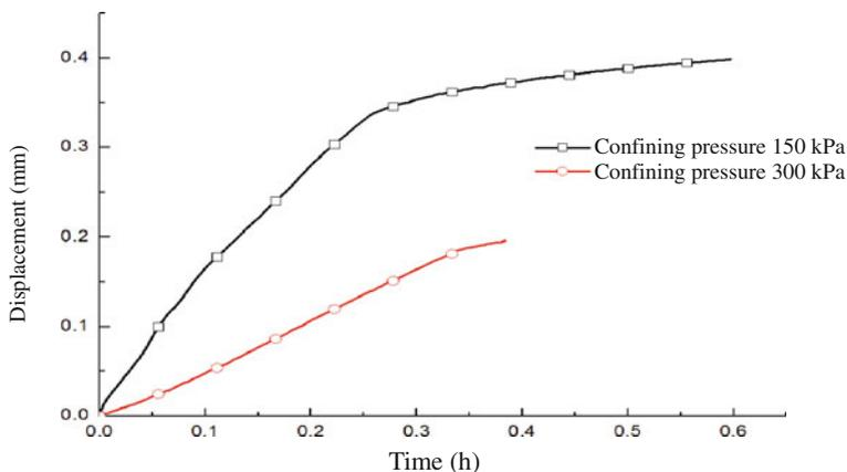
**Fig. 3.10** Deformation response of soft soil to different confining pressures
