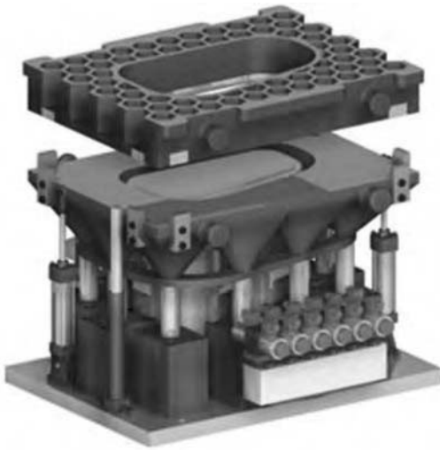
Fig. 13.18 Schematic of the cushion system built in the die. Source: Ref 13.15
