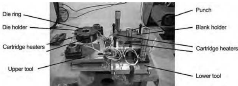
Fig. 11.23 Heated upper (left) and lower (right) tool sets used in the experiments. Source: Ref 11.16
