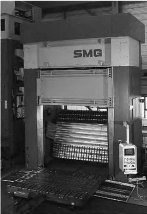
Fig. 12.24 A tryout press with moving bolster and rotating slide plate to allow quick reworking of the dies. Source: Ref 12.1
