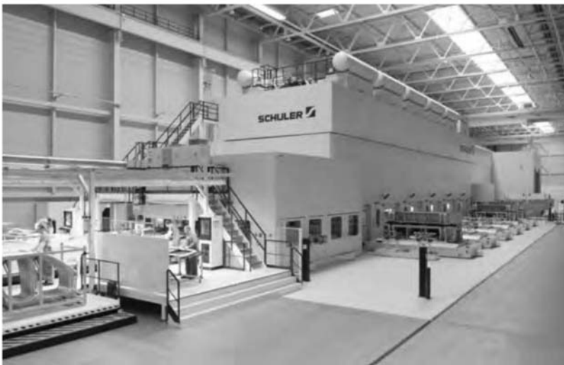
Fig. 11.28 Schuler servo-press line in BMW's plant in Leipzig, Germany. Source: Ref 11.21
