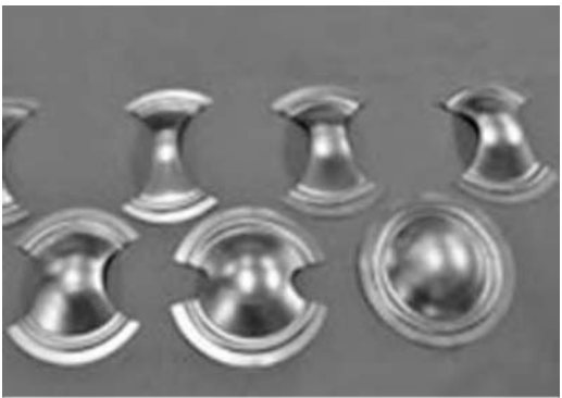
Fig. 4.34 Example specimens used in the limiting dome height test to obtain the forming limit curve (Ref 4.27)
