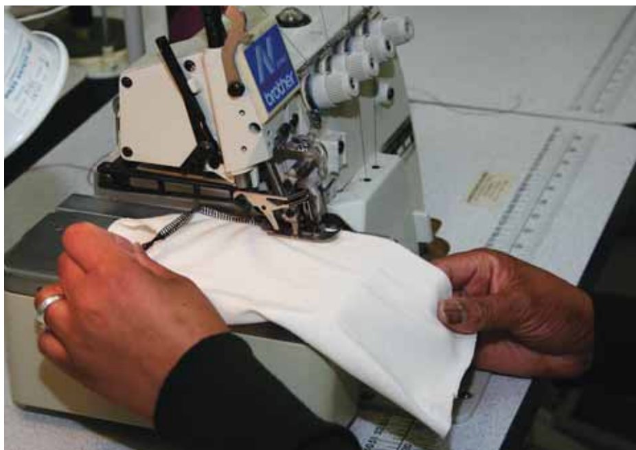
A 4-thread overlocking machine is used to sew knitted fabrics together.
