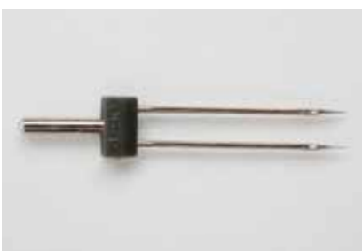
The Twin Needle is available with a sharp point or ballpoint and consists of two single needles inserted into an attachment to create a double stitch line. Both industrial and domestic machines use this needle. The twin needle is used mostly for topstitching.
