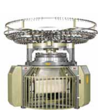
A circular knitting machine can produce single or double jersey.
