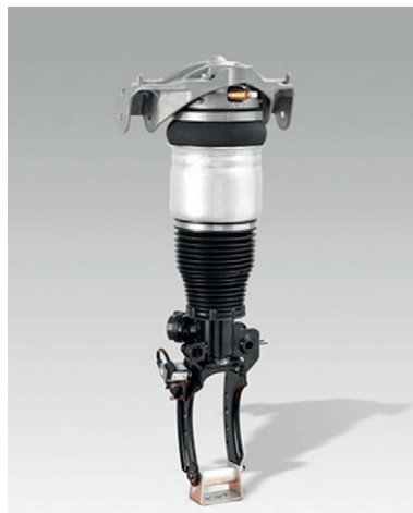
Figure 1.5: Example of a suspension of a luxury sedan (Audi A8), which integrates an electronically controlled gas spring with load-leveling capabilities, and a semi-active damper.
