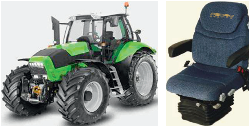
Figure 1.8: Examples of chassis-to-cabin (by Same Deutz-Fahr) and cabin-to-seat (by SEARS) semi-active suspension systems.
