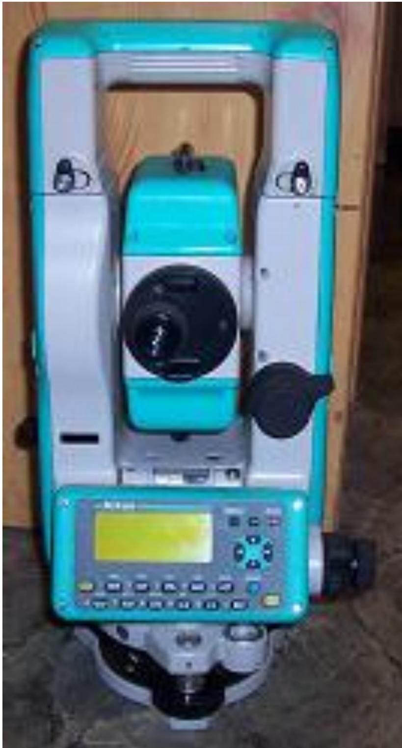
Figure 2: Example of Digital Theodolite
