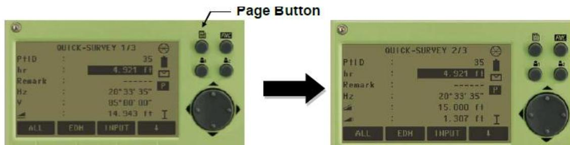
23. Press the **Page Button** to display the hz, Slope Distance (
