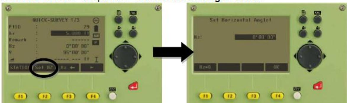
5. Aim at the back sight point then press **F1** “Hz=0”. Press **F4** “OK” to set the back sight angle. (Note: Press the button lightly so as not to change the alignment of the instrument!)
