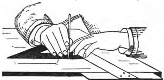
Fig. 10—Correct Manner of Holding a Ruling Pen.
