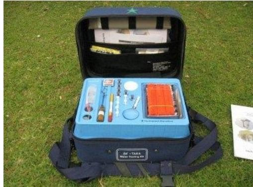
100 tests can be performed by this kit. However, 10 test for coliform can be done
