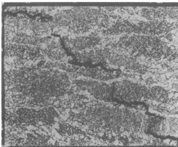
Figure 7.34 Chevron crack located in the recrystallised region of weld metal. (Photo.: Cranfield Institute of Technology.)
