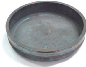
Figure 9. Flywheel plate of car with outer wall thickening.
