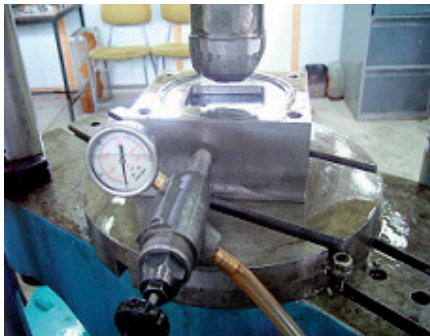
Figure 12. Photograph of the manufactured die set
