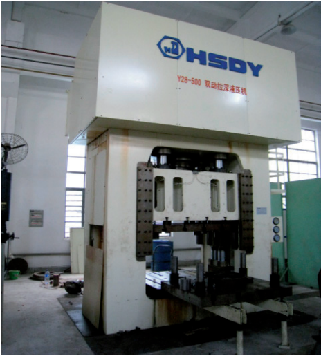
Figure 18. Dual-action deep drawing hydraulic press
