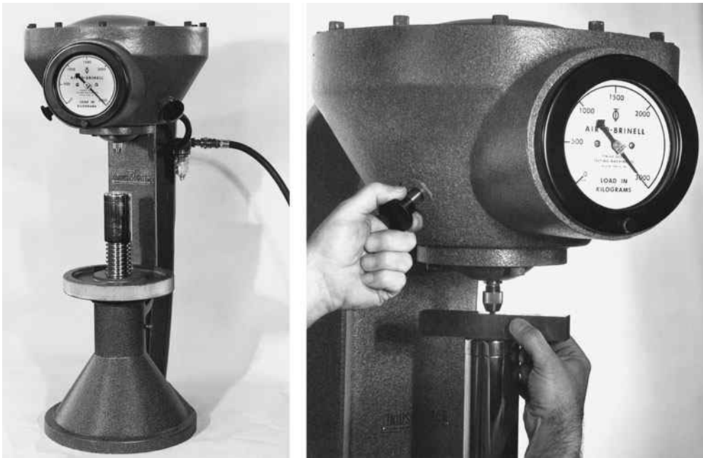
Figure 4.30 Brinell hardness tester (left), and indenter being applied to a sample (right). (Photographs courtesy of Tinius Olsen Testing Machine Co., Inc., Willow Grove, PA.)
