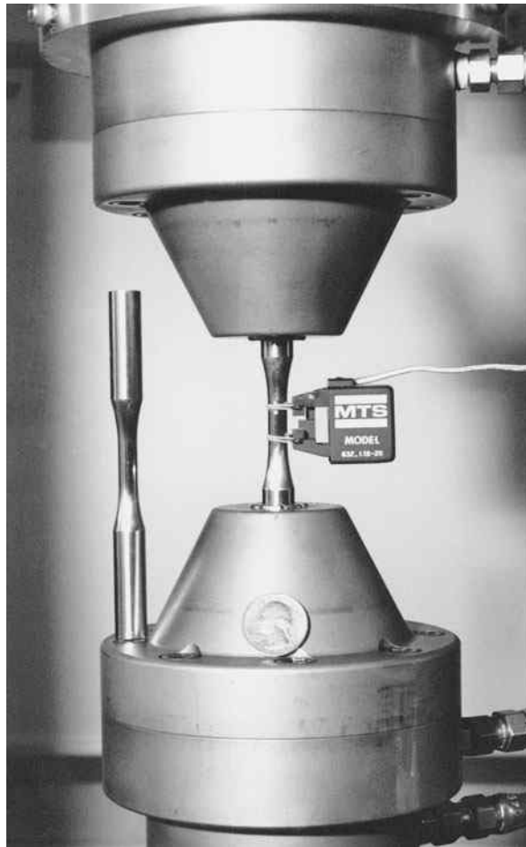
Figure 14.2 Test specimen, extensometer, and grips for strain-controlled fatigue testing. (Photo by G. K. McCauley, Virginia Tech.)
