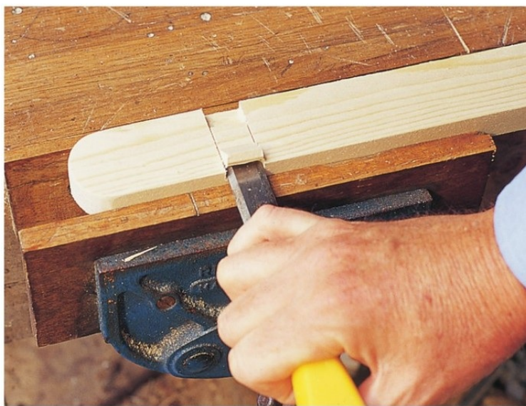
The waste is removed with the chisel.
