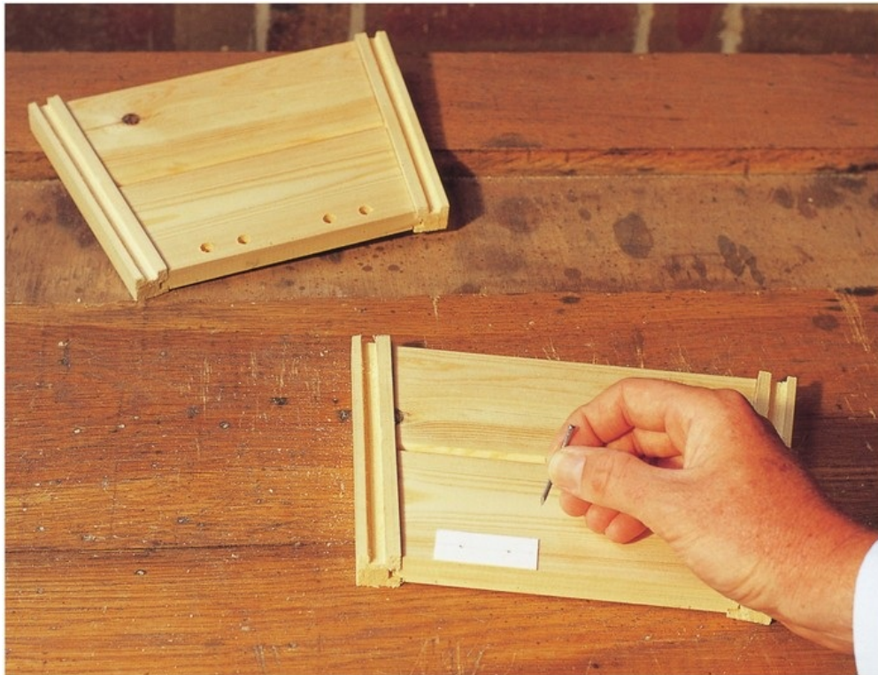
A card template and the point of a nail are used to mark in the dowel positions at the bottom of the two end panels.
