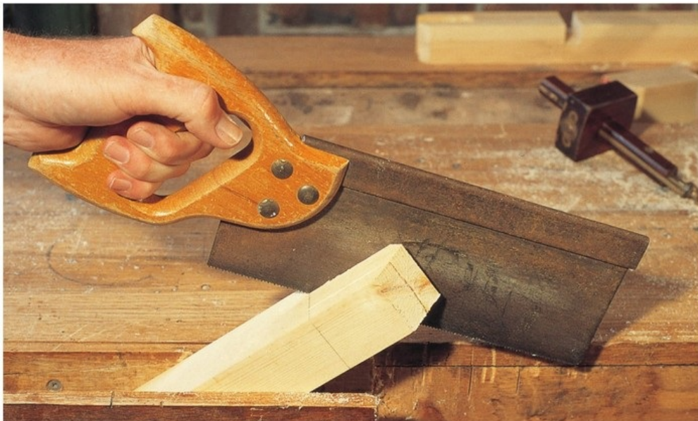
The post is clamped securely in the vice and the slot cut with the tenon saw.
