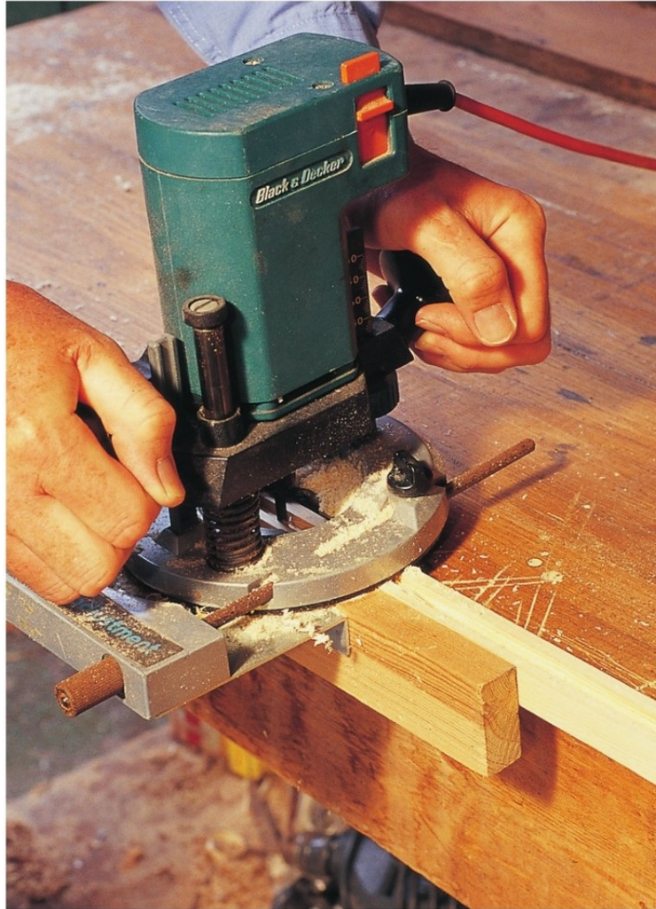
Preparing a groove with the electric router.
