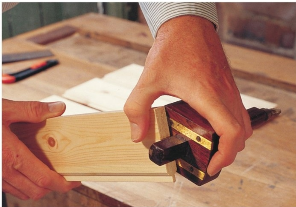
The tongue is marked on the end grain of each board with the mortise gauge.
