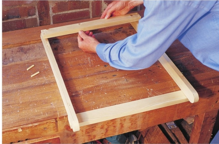
Fitting two crossbars to the back leg/front seat supports.
