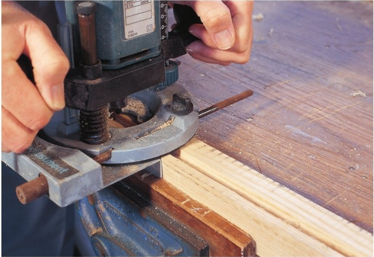
Cutting a groove with the electric router.
