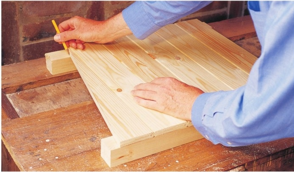
Mark the sloped edge on to the legs in pencil.
