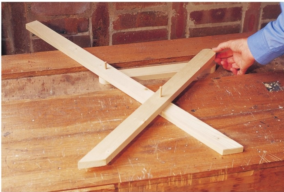
Make a trial fitting of a side assembly.
