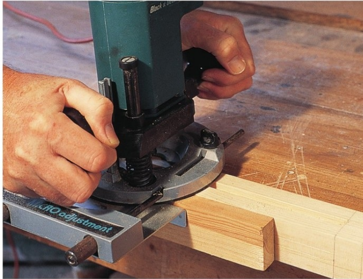
Cutting out the groove with the electric router.
