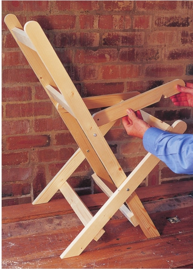
The seat rails are added to the chair frame.
