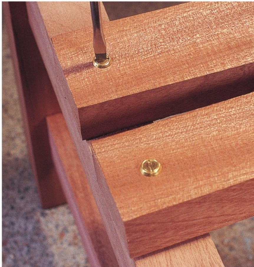
Assembling the seat slats with brass screws and cup washers.
