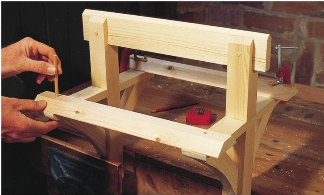
A dowel is fitted into its hole to join the rail, crossbeam and strut.
