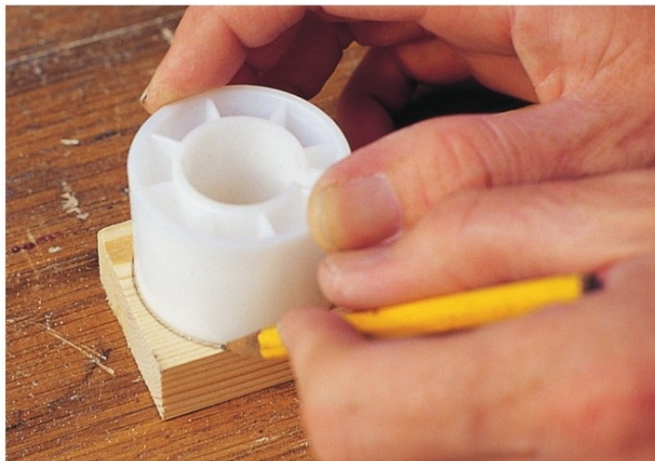
Use a pair of compasses, or any convenient round object, to mark the end of each upright.
