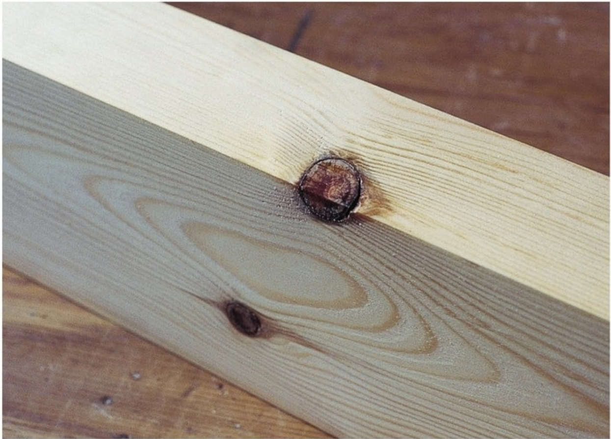
Knots such as this one are hard to avoid in softwoods such as pine.
