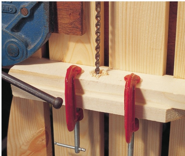
A piece of waste wood is clamped beside the rail to allow the auger bit to bore cleanly through without splitting the underside.
