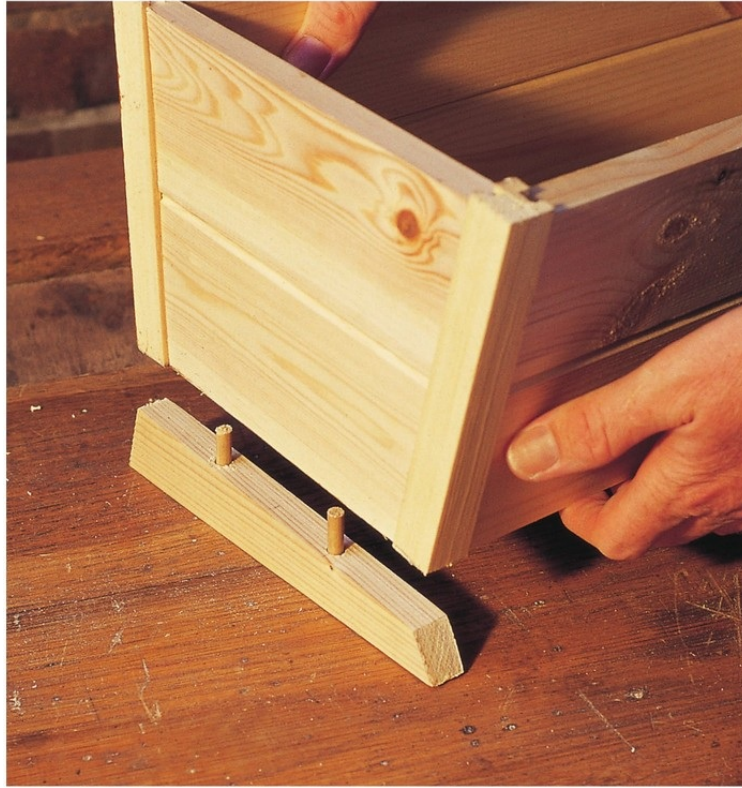
A foot is attached to the window-box with dowel joints.
