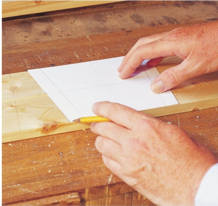
Using a card template to mark out the shape of an end panel.
