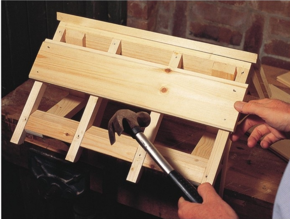
Fitting the roof covering, which is fastened to the rafters with glue and nails.
