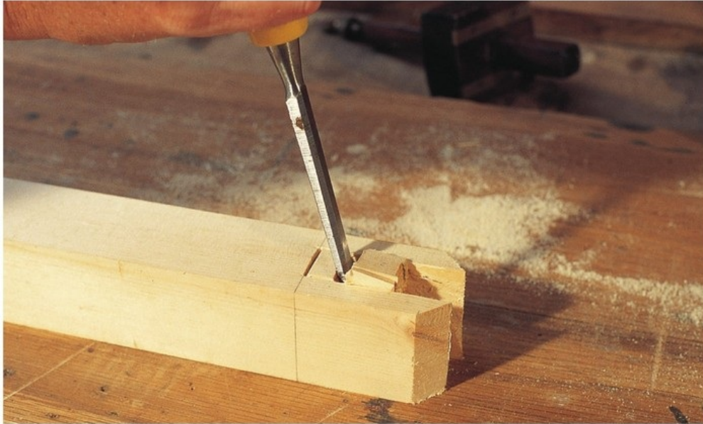
The waste is chopped out with the chisel, leaving the finished slot.
