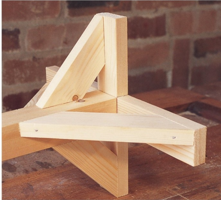
The cross is dowel-jointed to the top end of the supporting pole and strengthened with braces.
