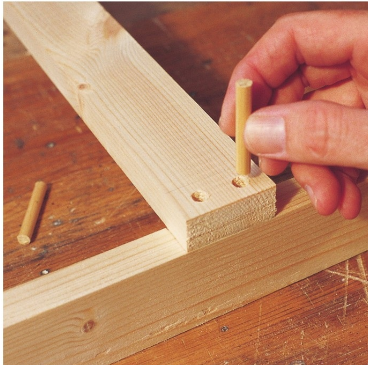
Assembling a crossbar to a leg with dowels.
