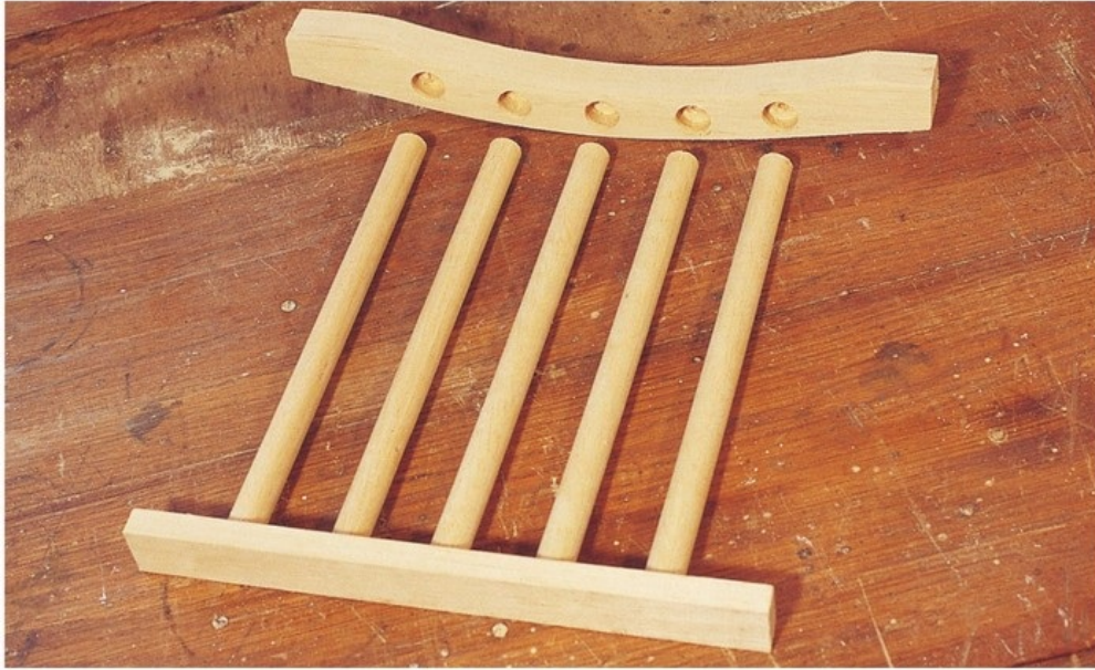
Assembling the backrest.
