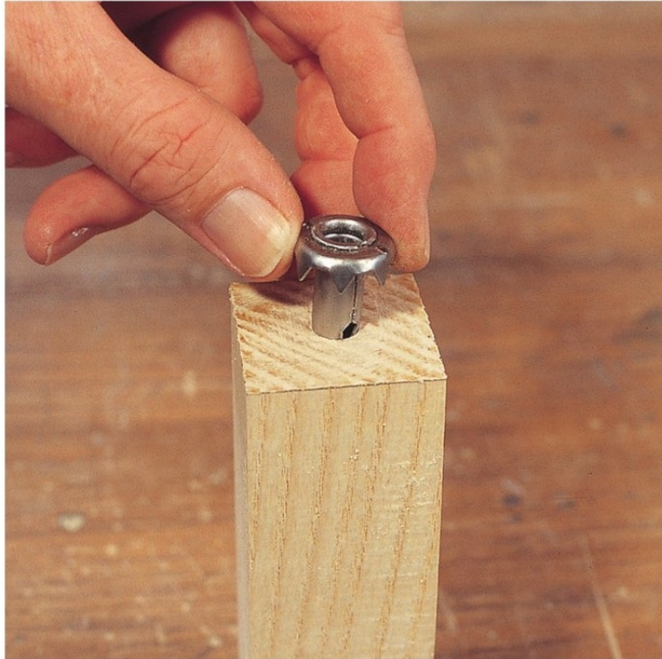
Fitting a wheel socket in the bottom of a leg.
