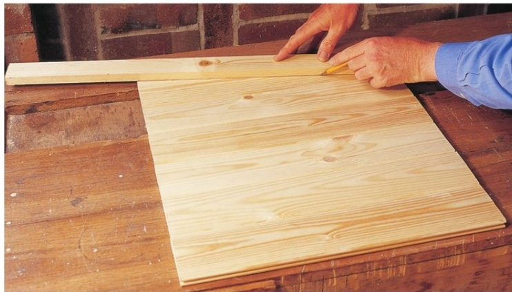
A straight-edge is used to mark in the slope along the top edge of a side panel.
