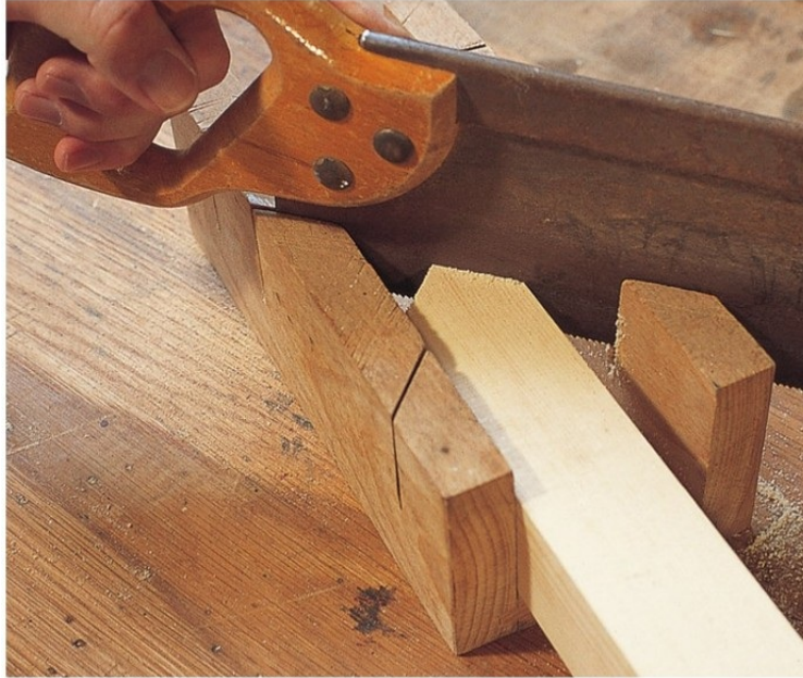
Mitres are cut at the end of a post, using the tenon saw and a mitre box.
