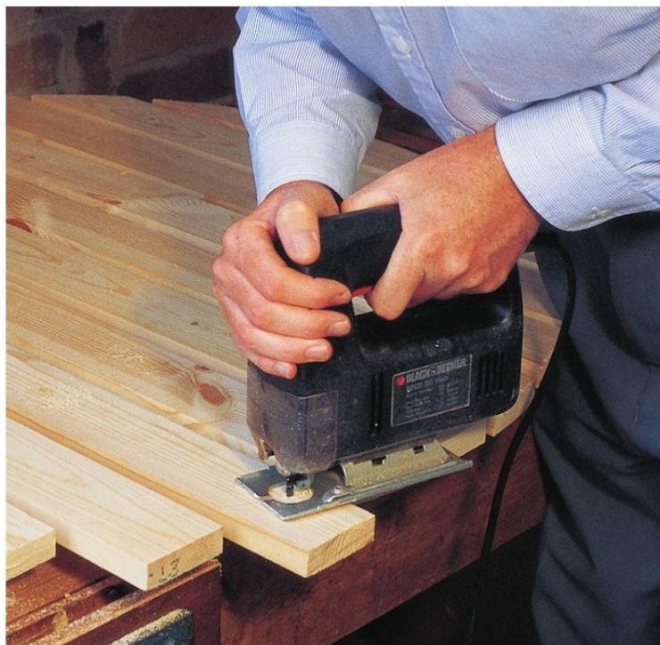
Cut around the curved pencil lines with the jigsaw to form the circular shape.
