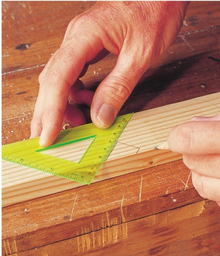
Mark a 45-degree mitre at the bottom of a back leg/front seat support piece using a geometrical set square.
