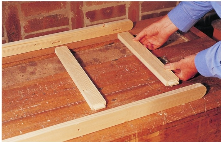
Tenons are cut at the ends of the two backrest slats to fit into mortises cut in the legs.
