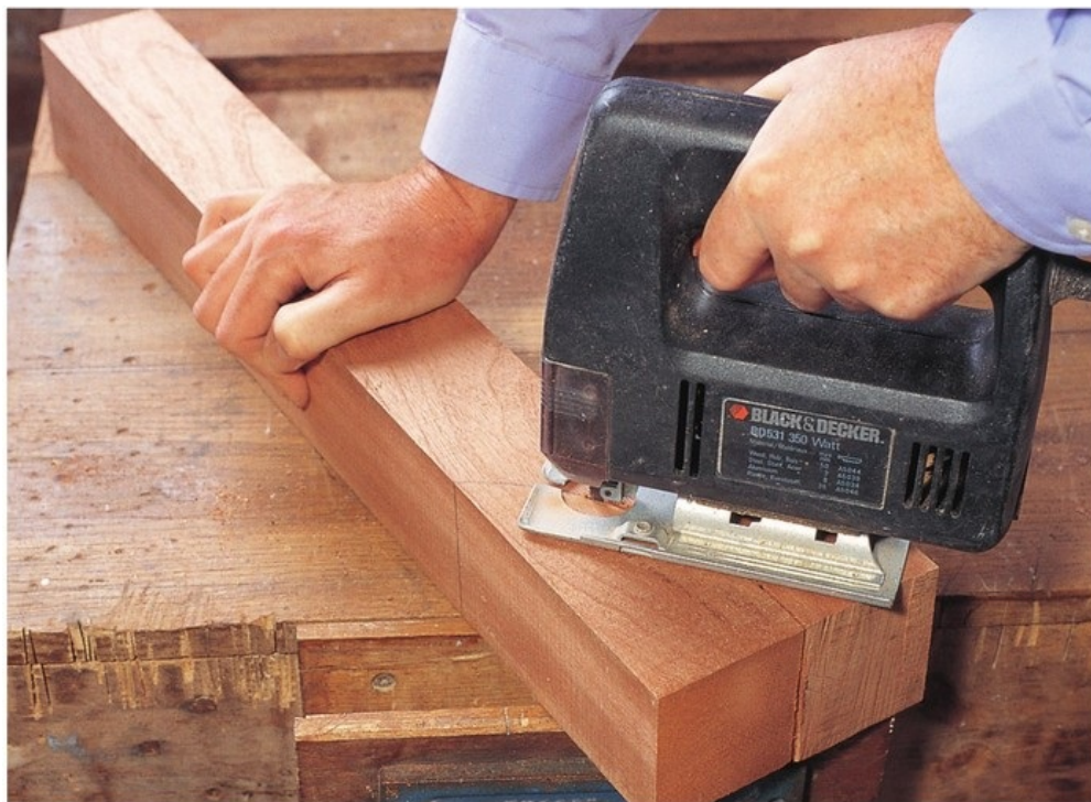
Cutting the front leg to shape with the jigsaw.
