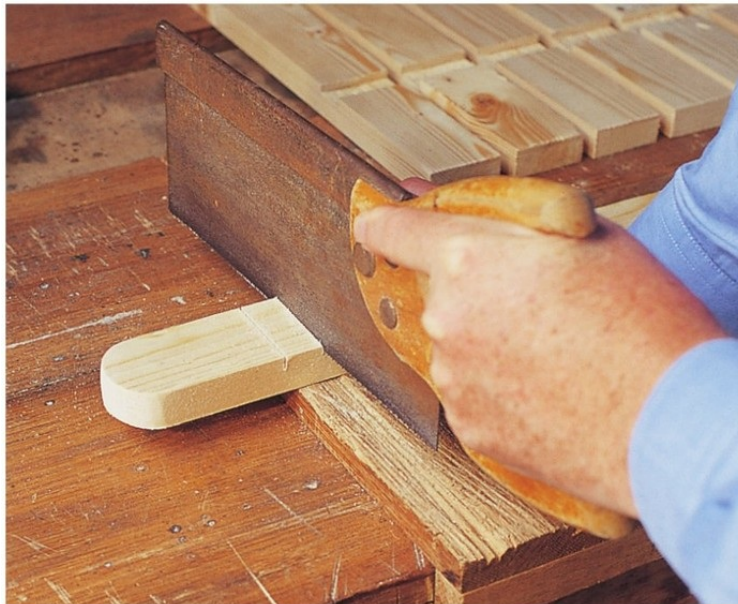
Cutting a notch with the tenon saw.
