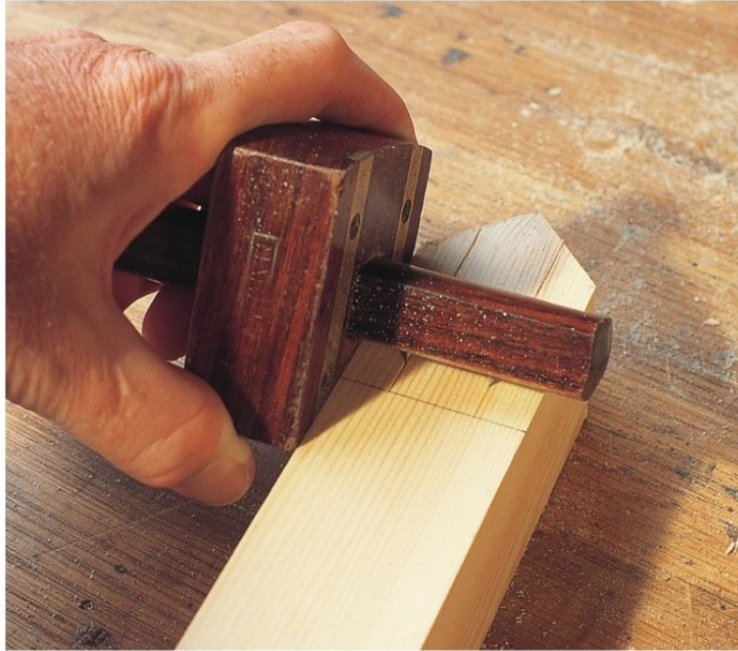
Scribing a pair of parallel lines at the top of the post with the mortise gauge.
