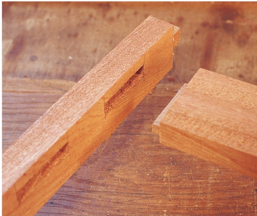
The completed bare-faced tenon cut in a table-top slat.
