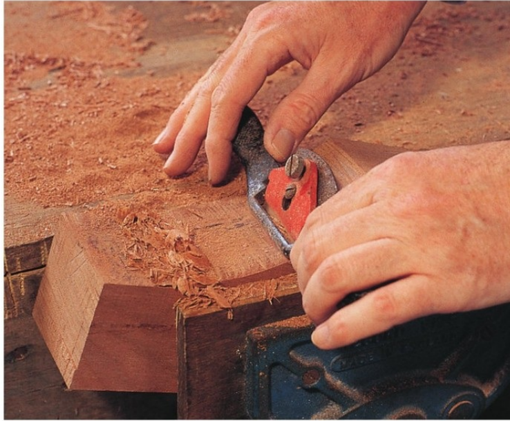
Shaping the curve of the front leg with the spokeshave.
