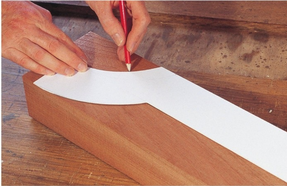
Marking out the front leg with the template.
