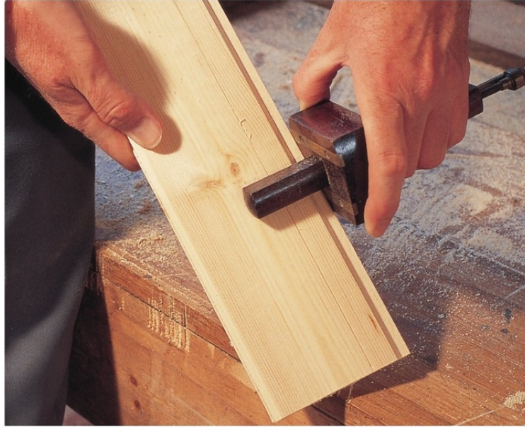
A line is scribed along the length of one board with the marking gauge to show how much waste needs to be removed.
