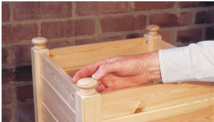
Ready-made wooden door knobs add a touch of decoration to the tops of the posts.
