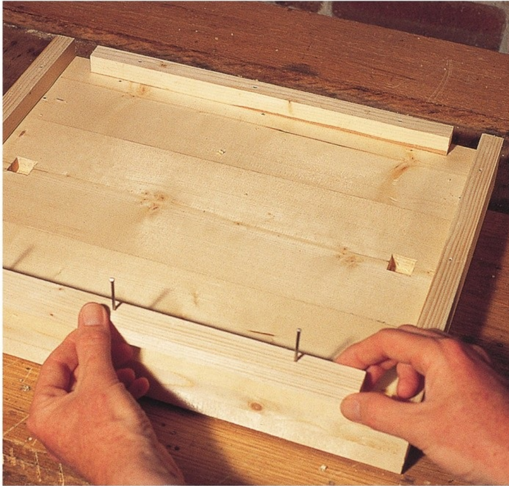
Four pieces of ledging are glued and nailed to the top surface of the base. Note the gaps left at the corners for cleaning out.
