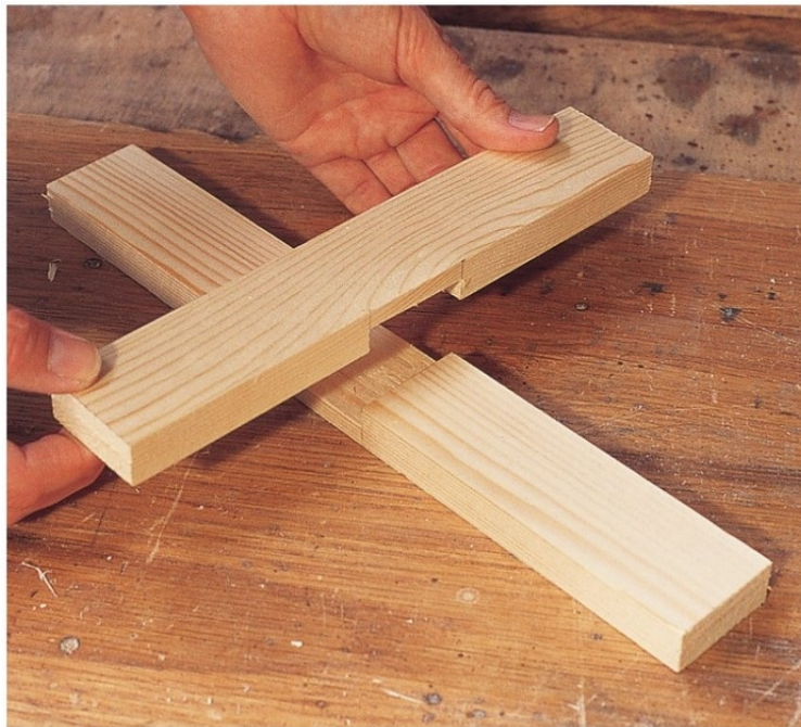
The two arms of the small uppermost cross are half-jointed together.
