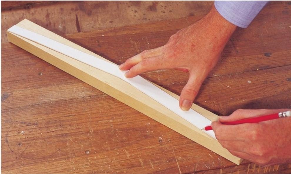
The back leg is marked out with a template.
