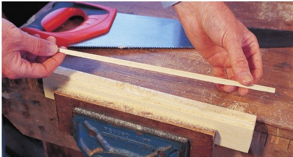
Cutting a rebate in the rail.
