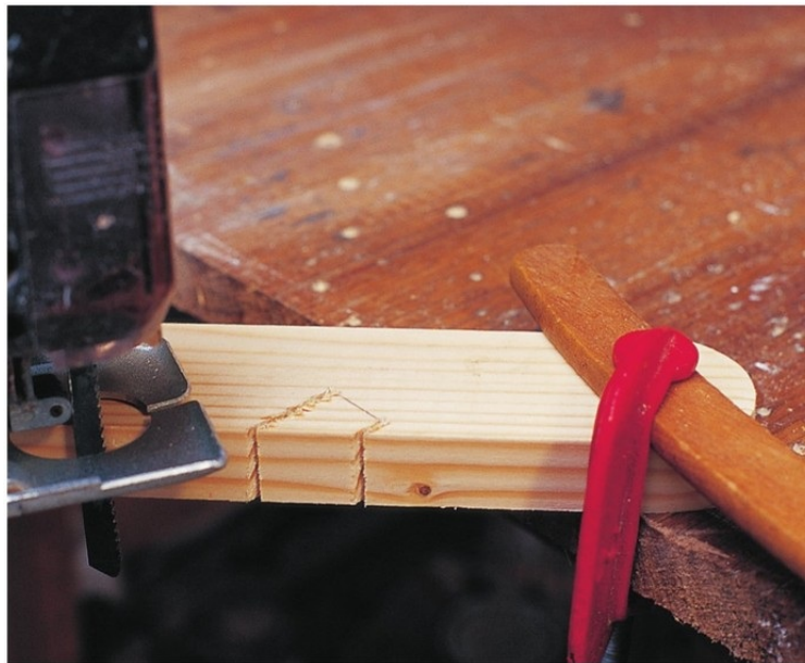
An angled slot is cut into the bottom edge of a seat rail with the jigsaw.
