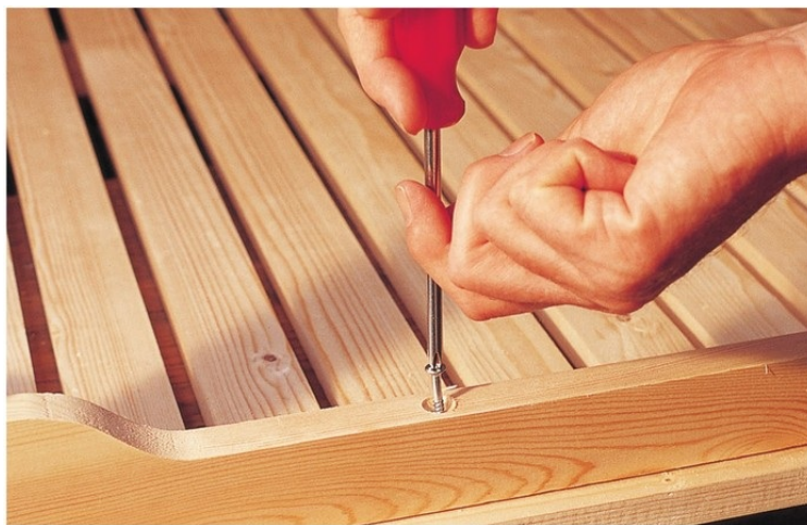
The leg sub-assembly is screwed to the underside of the table top.
