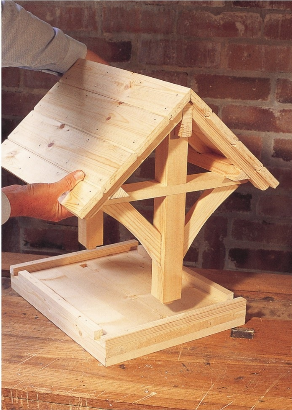
The main assembly of the bird house is attached to the base with mortise and tenon joints.
