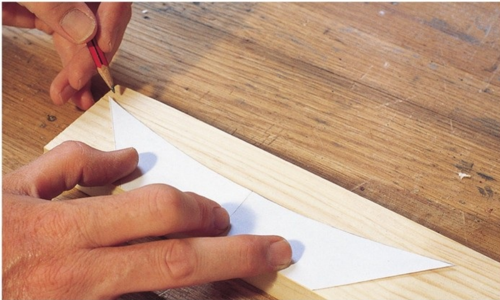
A card template of a strut is placed on the wood and marked out.
