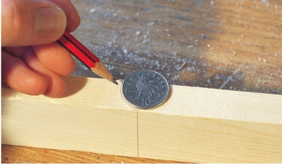
The curved ends of two crossbeams are marked simultaneously using a pencil and coin.
