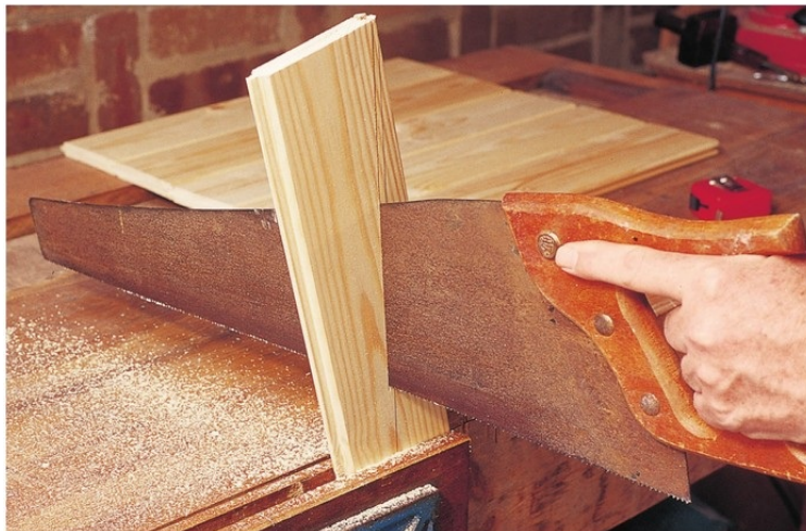
Cut away the waste with the handsaw.
