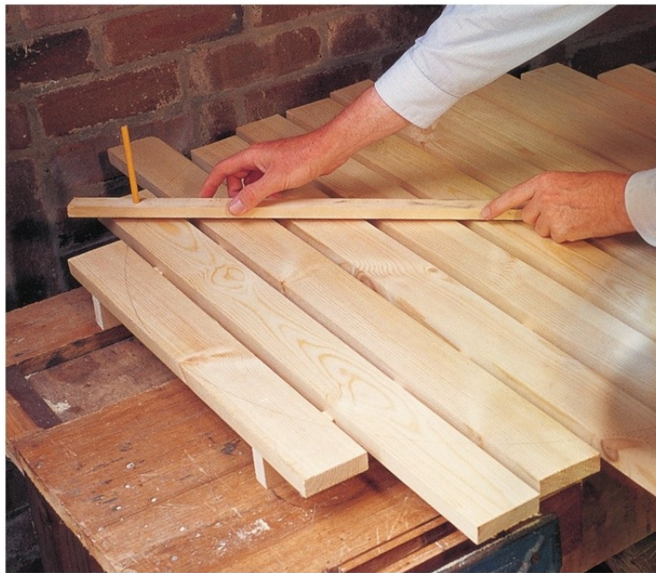
Mark in the circular table-top pattern with the home-made 'compass'.
