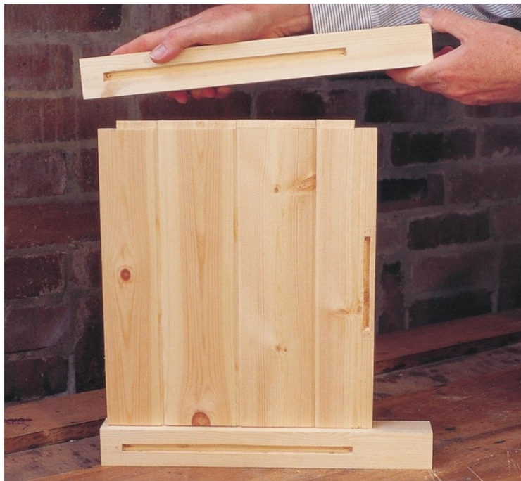
Assemble each of the four panels to their legs to check that the joints fit perfectly.
