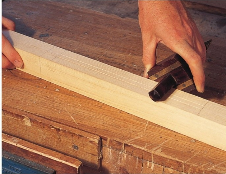
Marking a groove along the length of the post material using the mortise gauge.
