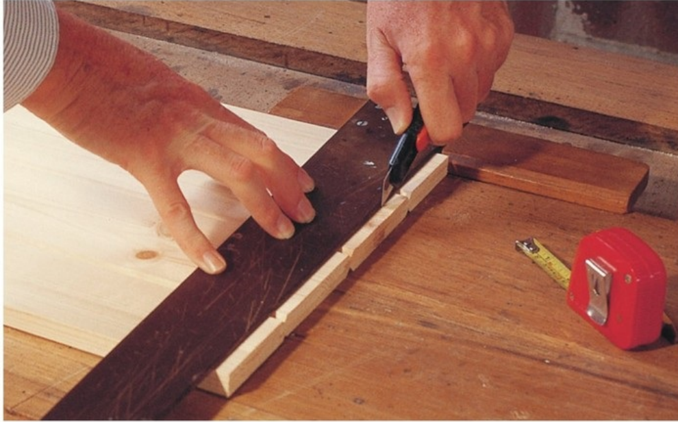
Use a straight-edge to mark the tongue positions at each end of the temporarily-assembled boards.
