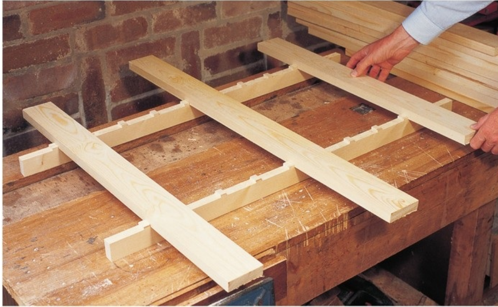
Assembling the table-top slats in their notches.
