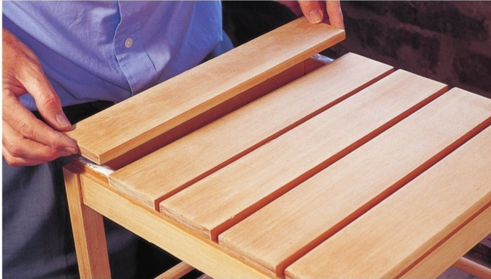
Placing the table-top slats in position.
