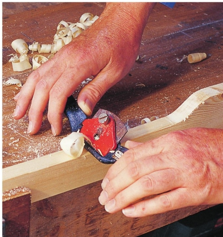
Shape the bottom edge of the bottom rail with the spokeshave.
