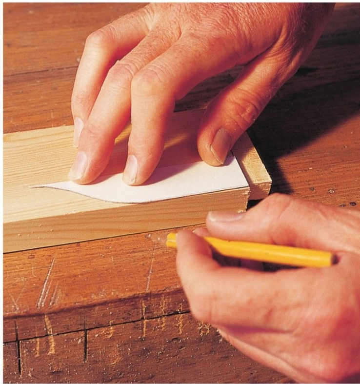
Mark the curve on the bottom edge of each rail with a card template.
