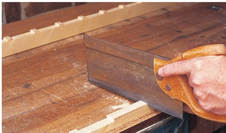
Cutting the lines for the notches with the tenon saw.
