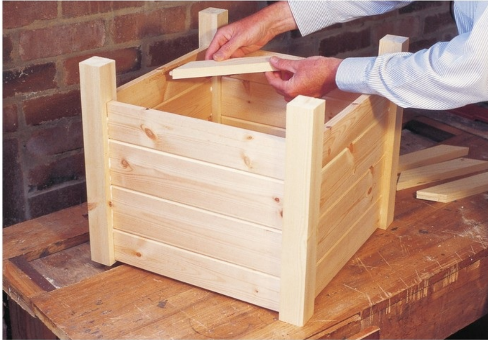
A batten is slotted into position on the underside of the assembled box.
