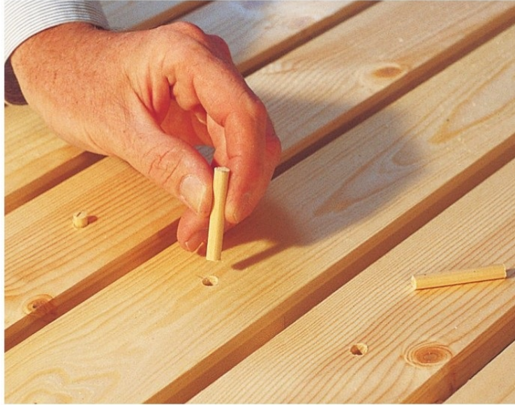
Fit the dowels into their receiver holes to join the table-top slats to the two rails.
