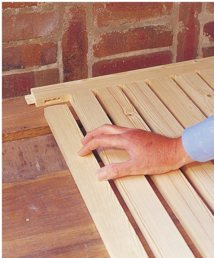
Making a trial assembly of the table top.
