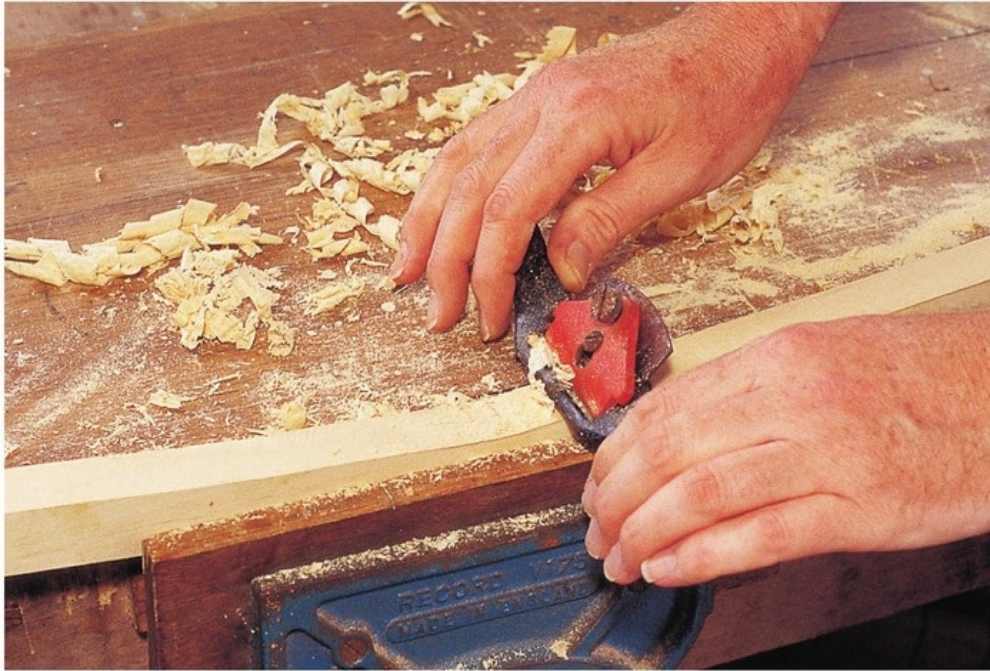
Shaping the back leg with the spokeshave.
