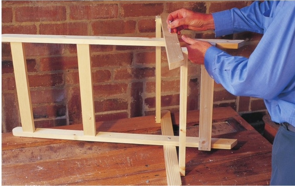
The first two parts of the chair frame are assembled.
