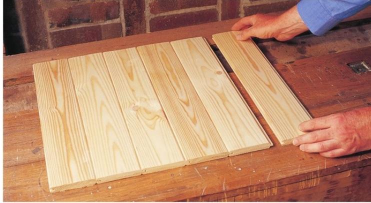
Six boards are cut and joined together to form a side panel.
