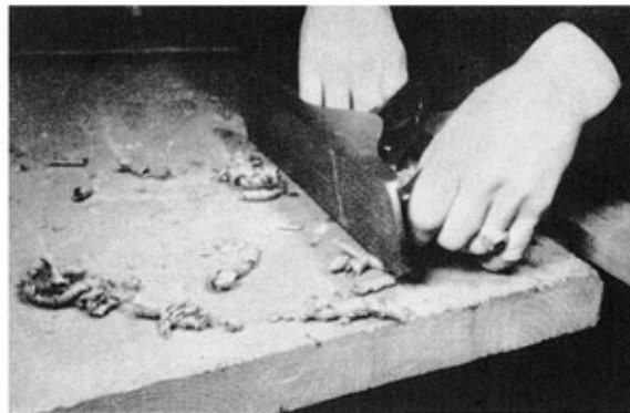
Fig. 3A. Correct method of laying plane on bench when not in use.
