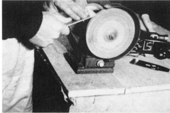
Fig. 2. Grinding the plane blade. Note carefully how the blade is held.
