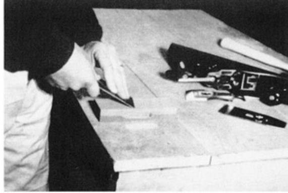
Fig. 3. Whetting the plane blade. Note the angle of the blade resting with bevel flat upon oilstone. Whet blade with a circular motion covering entire stone to keep stone as flat as possible.
