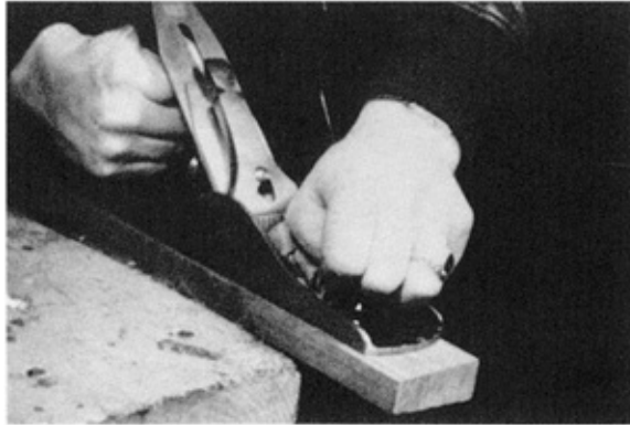
Fig. 5. Unless the stock is badly warped, keep the plane parallel to the edges. This helps to keep the surface flat.
