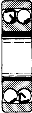
Figure 9.12 Double-row internal self-aligning bearing.
