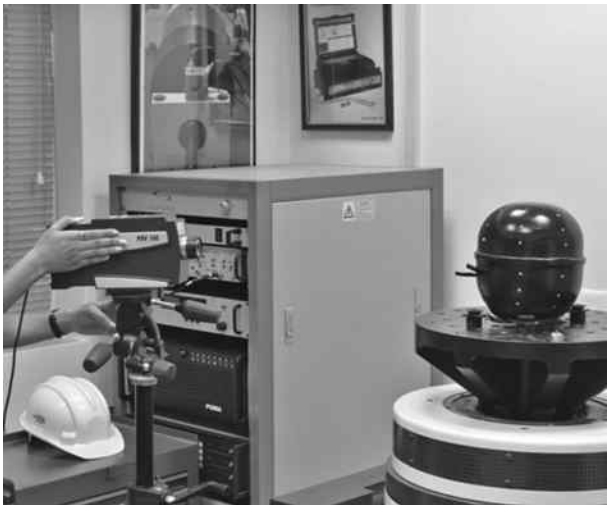
FIGURE 6.8 Compressor vibration measurements using a laser vibrometer.
