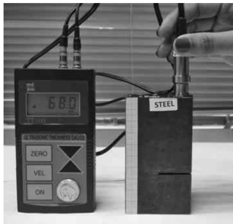
FIGURE 6.16 Ultrasonic wave traversing a sample.
