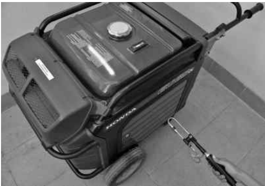
FIGURE 8.5 Sound intensity measurements on a portable generator.
