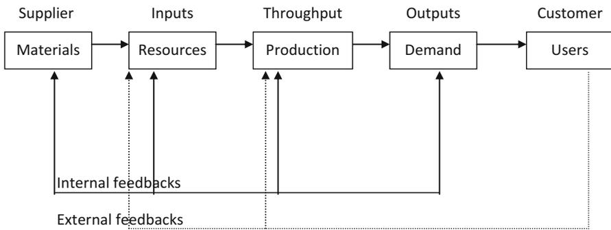
The above diagram represents the production system of a factory. By constructing this system with its major five blocks and by finding the feedbacks that affect its function the team of the factory can explore potential problem areas, such as:
