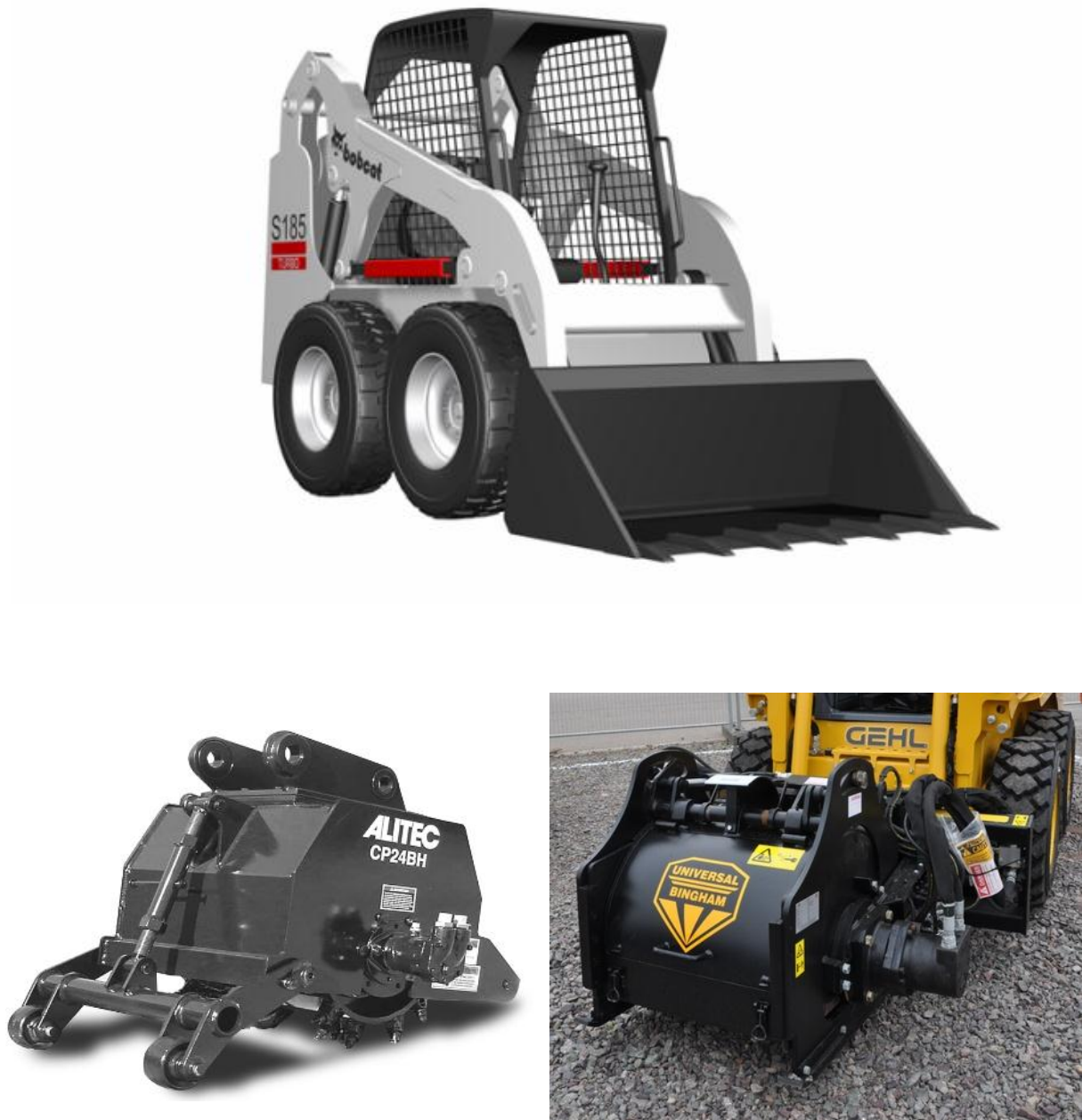
Figure 17 – Skid Steer tractor and cold milling attachments for bitumen pavement re-cycling
