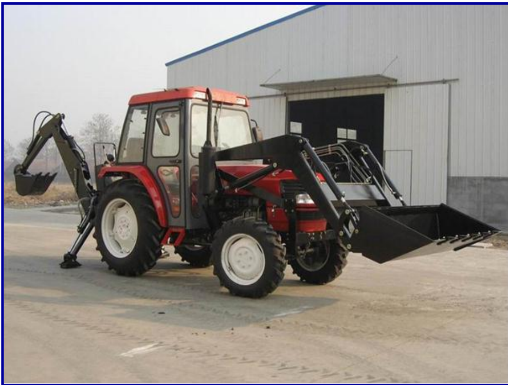
Figure 6 – Front end loader and backhoe attachments
