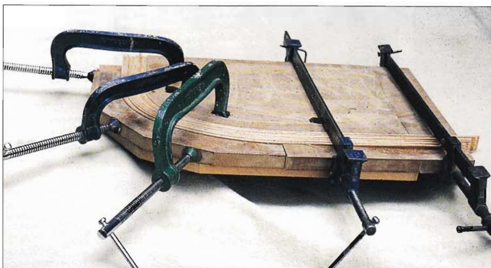
ABOVE: Arm gluing-up in jlg
