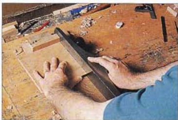
ABOVE: No cross-cut saw! Use a shooting board to square the ends of carcass components
