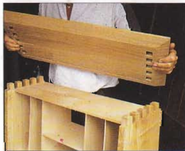
BELOW: Top with 30° chamfer ready for assembly – note mortices
