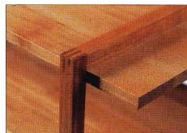
ABOVE: Plenty of gluing area makes this joint both strong and attractive
