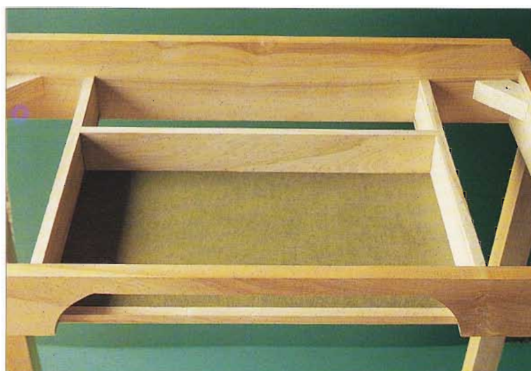
BELOW: Internal structure of desk, corner blocks are used to fix the top
