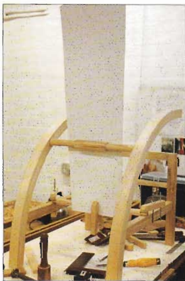
TOP: Adjustable bevel being used to establish backrest angle in relation to turned rails
