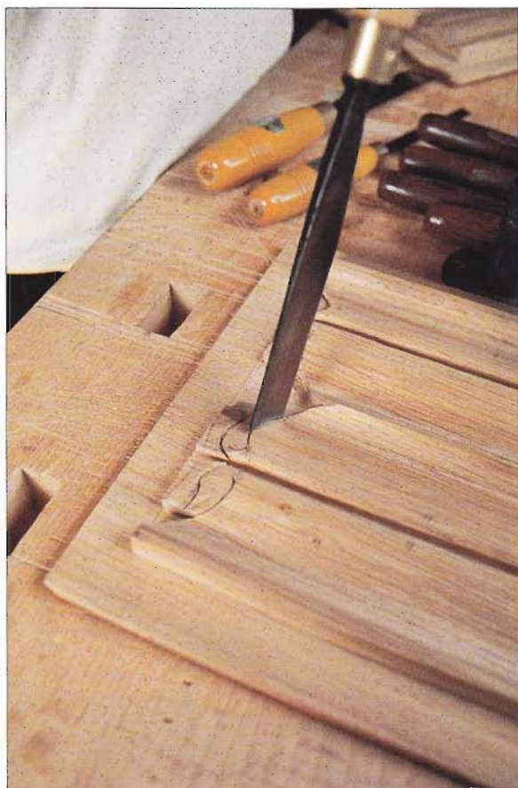
ABOVE: The previously drawn folds are now marked out with the appropriate chisels
