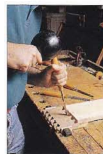
ABOVE: Chopping out the pins – note the angle at which the chisel is held; doing this from both faces leaves a 'hill'
