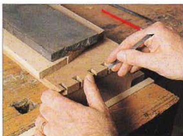
ABOVE: Marking pins from tails – note the weight holding things in position and the double-ended, alternate bevel marking knife
