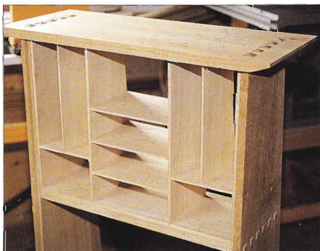
ABOVE: Dry-fit assembly of carcass
