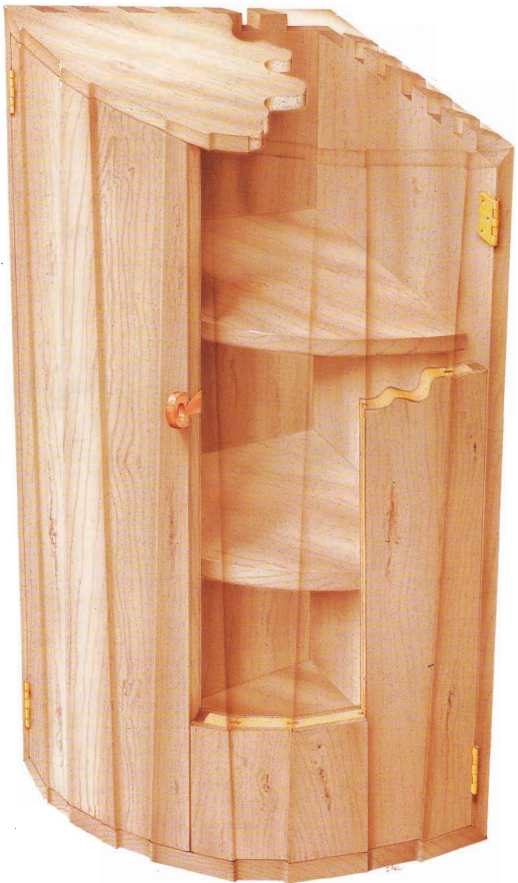
ABOVE: Photo 6 Pin sockets cut – the mitred corners frame the doors nicely
