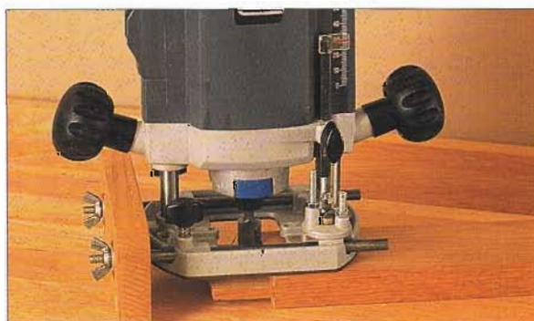
BELOW: Bob's levelling foot in action
