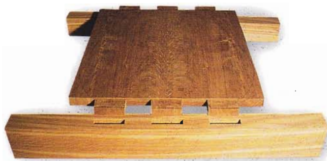
ABOVE: Three tenons at each end join trestle-ends to feet and bearers
