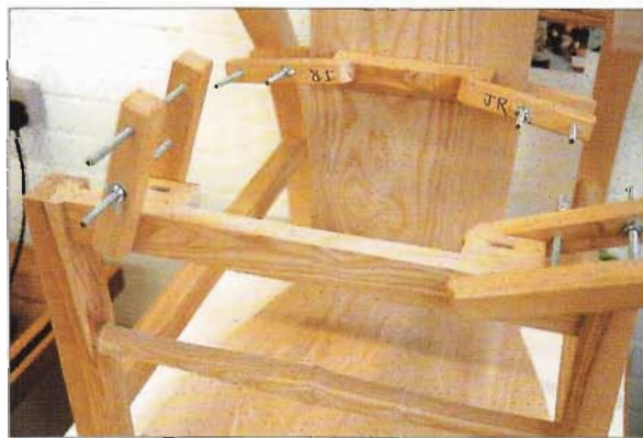
BELOW: Slotted blocks and glue block on backrest to fix seat
