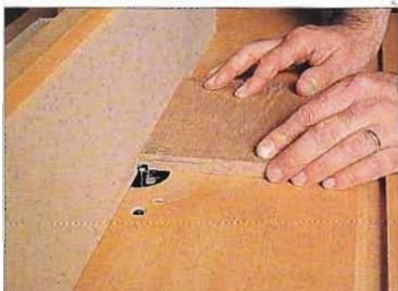
ABOVE: As the ends of the carcass joints are mitred, the back's rebate can be run through. Here a table-mounted router is used, but a rebate plane would do as well
