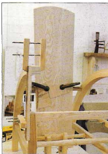
BELOW: Backrest glued and clamped into position
