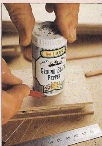
ABOVE: That essential workshop aid, the pepper pot, is used to mark out the inlay design
