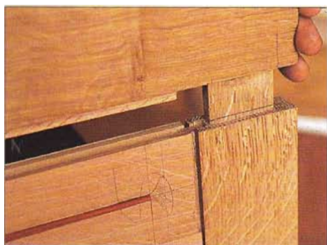
FAR RIGHT: Close up of groove for one of the segments of the inlaid door panel
