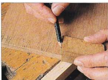
ABOVE: Marking the carcass dovetails using a home-made wooden block and a pencil sharpened to a chisel point. Note the hatching of the waste area to be cut out
