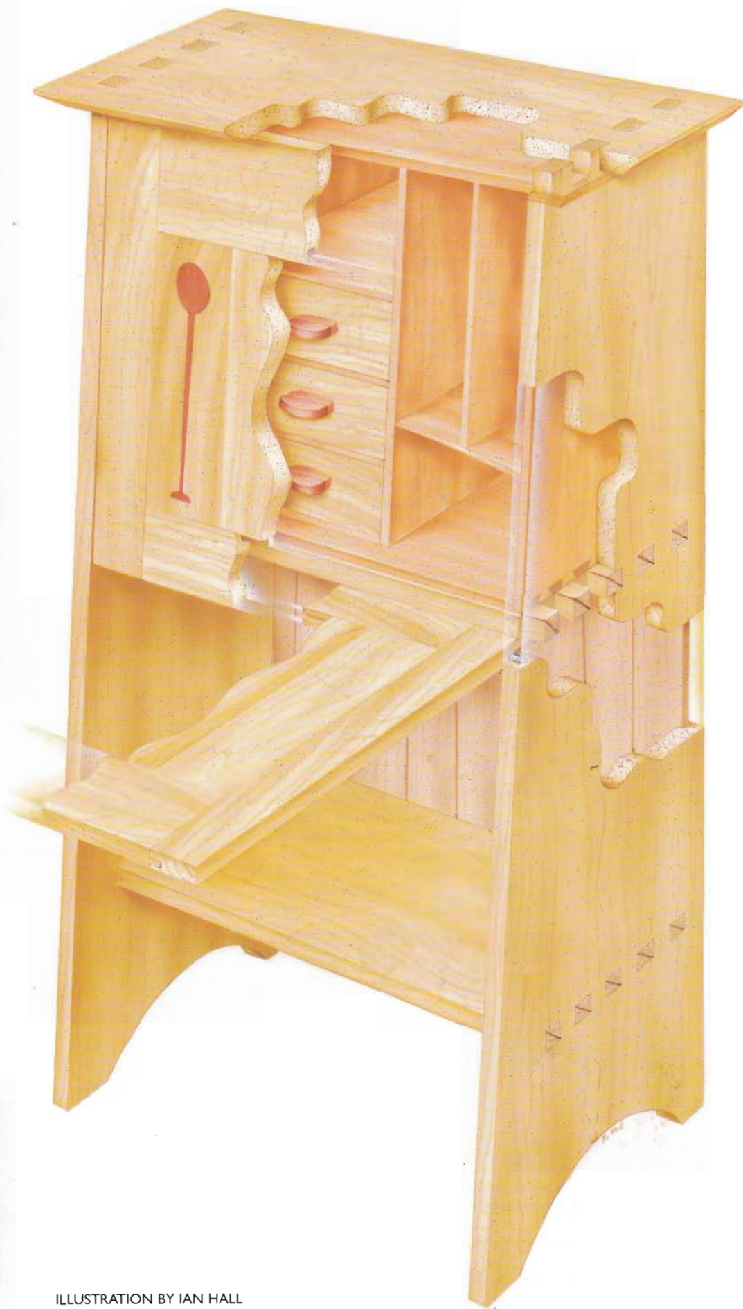
ABOVE: Complete interior carcass assembled and being tried for fit
