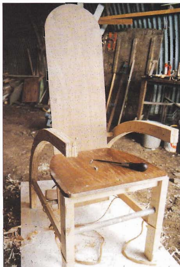
ABOVE: Full-size mock-up used at home to test out the practical reality of the design
