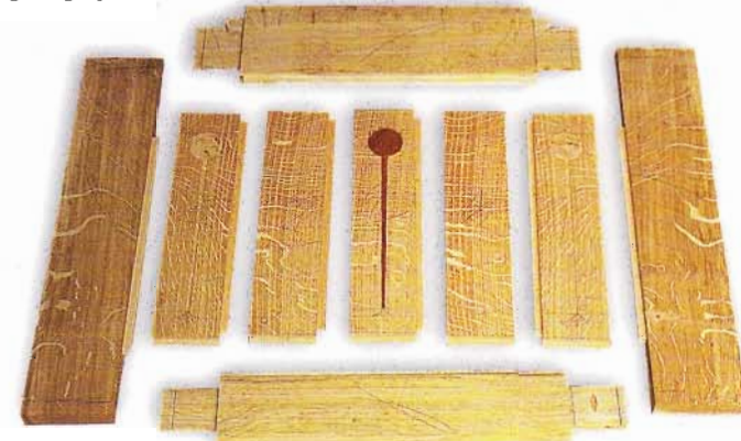
BELOW: Door components, splines and inlay almost ready for gluing up
