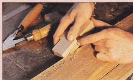
BELOW: Cutting a bead with the screw's slot
