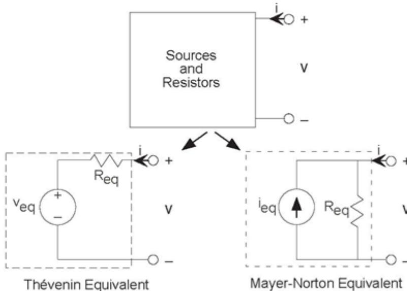
**Figure 3.20 Thevenin and Mayer-Norton equivalent** All circuits containing sources and resistors can be described by simpler equivalent circuits. Choosing the one to use depends on the application, not on what is actually inside the circuit.
