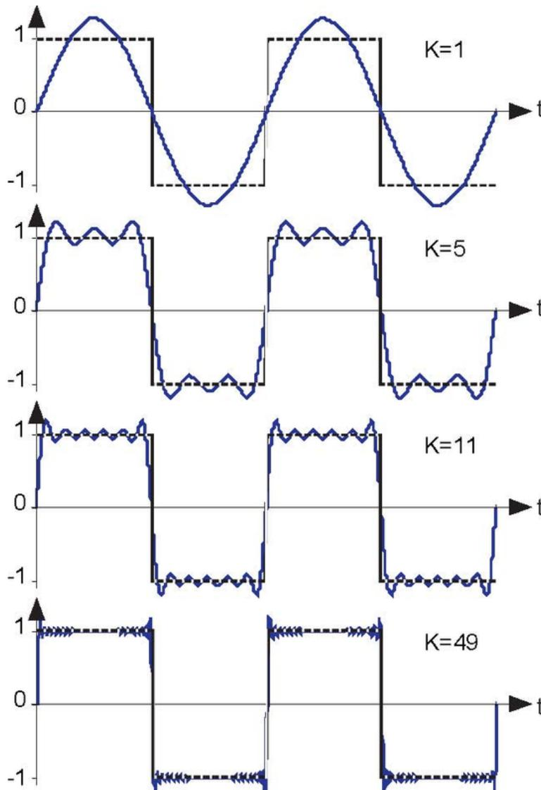
Figure 4.8 Fourier series approximation of a square wave Fourier series approximation to  $\text{sq}(t)$ . The number of terms in the Fourier sum is indicated in each plot, and the square wave is shown as a dashed line over two periods.
