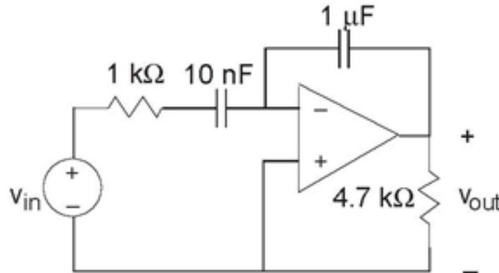
Figure 3.86 op-amp circuit
