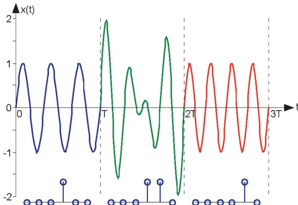
**Figure 4.9 Encoding Signals** The encoding of signals via the Fourier spectrum is shown over three "periods." In this example, only the third and fourth harmonics are used, as shown by the spectral magnitudes corresponding to each  $T$ -second interval plotted below the waveforms. Can you determine the phase of the harmonics from the waveform?
