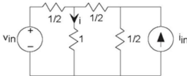
Figure 3.55 Superposition Principle
