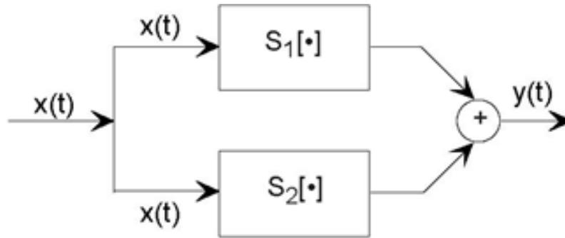
Figure 2.11 The parallel configuration.
