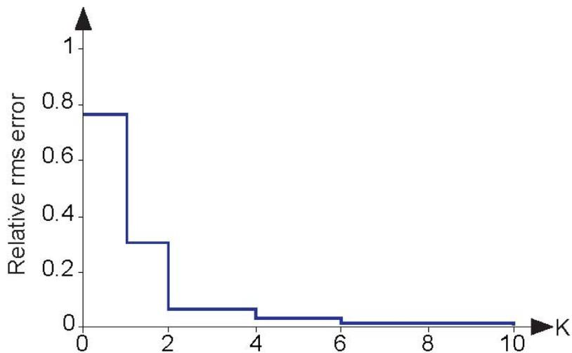
**Figure 4.6 Approximation error for a half-wave rectified sinusoid** : The rms error calculated according to (4.25) is shown as a function of the number of terms in the series for the half-wave rectified sinusoid. The error has been normalized by the rms value of the signal.
