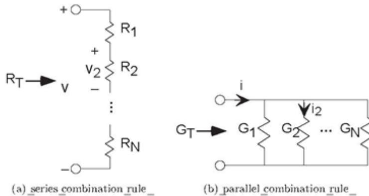
Figure 3.15 Series and parallel combination rules
