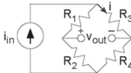
Figure 3.59 Bridge Circuits
