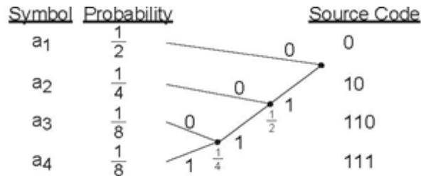
Figure 6.18 Huffman Coding Tree
