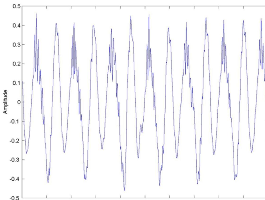
**Figure 1.1 Speech Example** A speech signal's amplitude relates to tiny air pressure variations. Shown is a recording of the vowel "e" (as in "speech").
