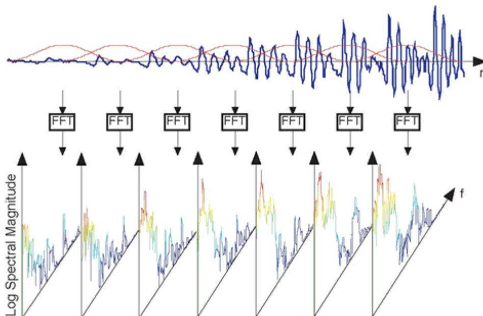
**Figure 5.17 Overlapping windows for computing spectrograms**
