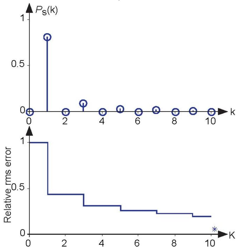
**Figure 4.7 Power spectrum and approximation error for a square wave** The upper plot shows the power spectrum of the square wave, and the lower plot the rms error of the finite-length Fourier series approximation to the square wave. The asterisk denotes the rms error when the number of terms  $K$  in the Fourier series equals 99.
