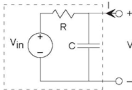
Figure 3.28 Simple RC Circuit
