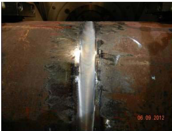
Figure 7. Photograph of a completed weld trail using the ExxonMobil root arc weld approach.
