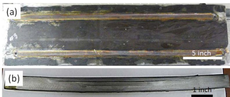
Figure 3 (a) Top view of finished weld (b) cross sectional image of MM-FSW steel sample.
