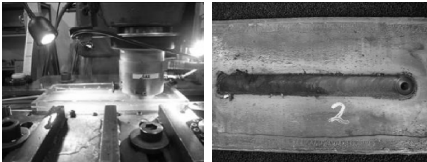
Figure 1: (a) Photograph showing the progress of underwater FSP of HY80 steel plate (b) typical appearance of an underwater FSP carried out at 400rpm/2ipm
