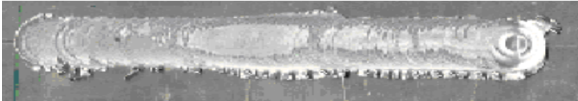
Figure 4. Photograph of FSW joint with varying weld traverse speed (Weld 2)
