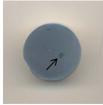
Figure 1. AA6061 Cylinder Samples with AA 2195 markers 1/3 radius position
