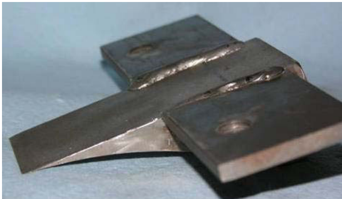
Figure 4. Cross-section of the run-off ramp.
