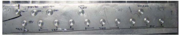
Figure 23 (Fasteners made in coupon tool for assessing diameter) 9 second fastener process time, 5782 N forge (Z), 2625 RPM with 0.418 in diameter
