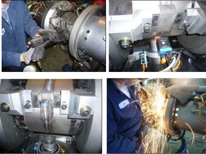
Figure 5. a) The run-off ramp is attached to the pipe allowing for a small amount of weld overlap, b) the tool approaches the run-off ramp, c) the tool traverses onto the run-off ramp with a change in weld parameters to increase the heat input, and d) the run-off ramp is removed by grinding.
