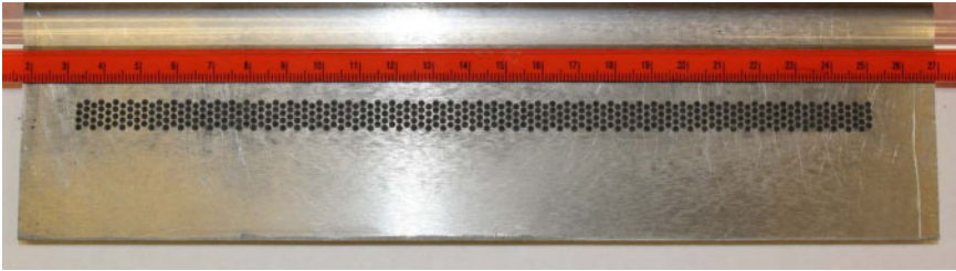
Figure 1. Top view of the staggered holes of eight rows in 5024 Al base metal and filled with B 4 C powder.
