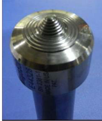
Figure 1. Photograph of a standard convex scroll shoulder step spiral (CS4) pcbn tool.
