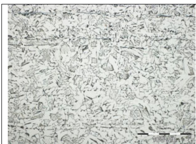
Figure 3.- Optical micrograph of the transverse section of the as received steel (500x)
