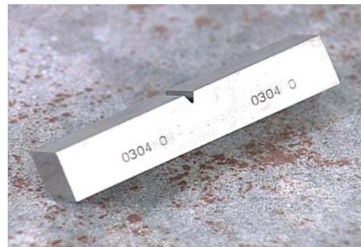
Illustration 7-3 – Charpy V-Notch Bar
