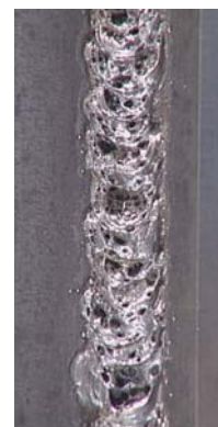
Illustration 12-3 – left to right: Linear Porosity, Clustered Porosity, Uniformly Scattered Porosity
