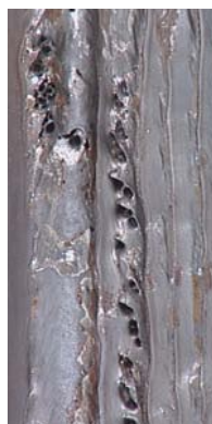
Illustration 12-3 – left to right: Linear Porosity, Clustered Porosity, Uniformly Scattered Porosity
