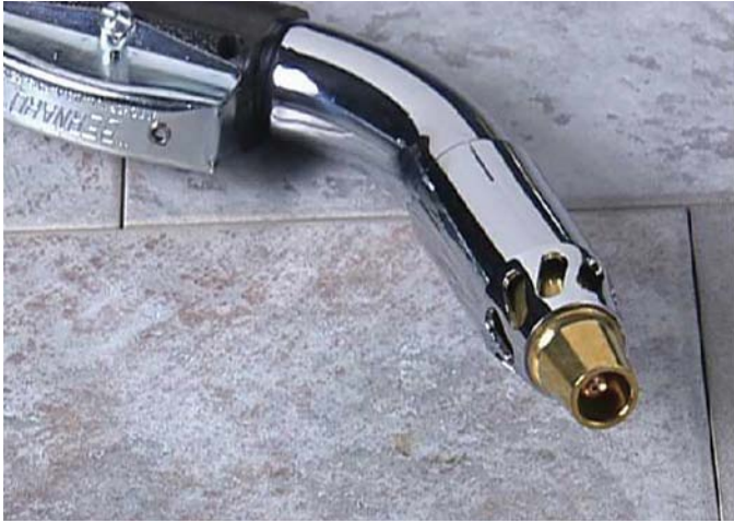
Illustration 3-14 –Fume Extractor Nozzle
