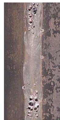
Illustration 12-3 – left to right: Linear Porosity, Clustered Porosity, Uniformly Scattered Porosity
