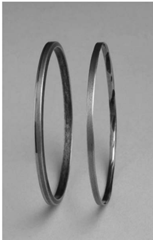
Fig 11-17. Worn oil ring on right (Source: TRICO Corporation, Pewaukee, Wisconsin)
