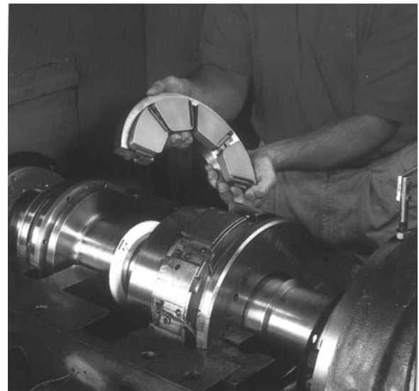
Figure 12-36. KingCole's unique split-ring design makes installation easier than standard bearings.
