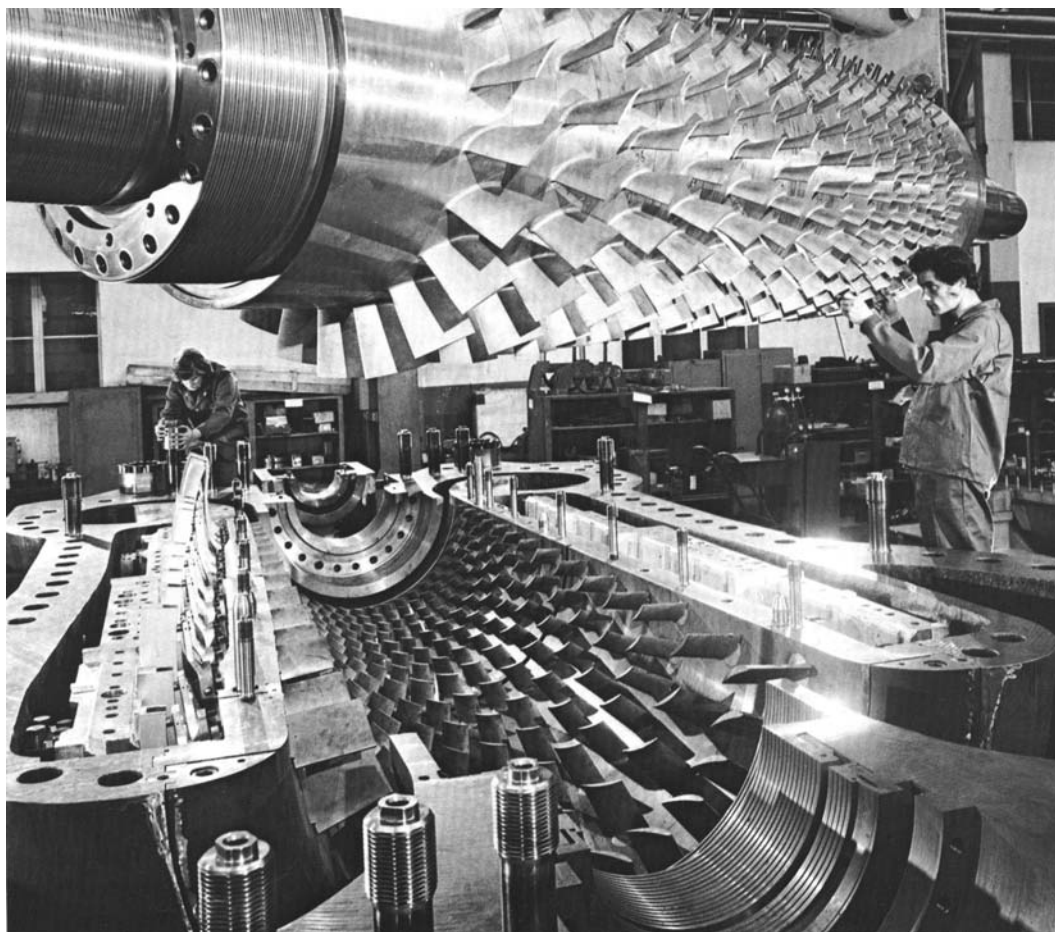
Figure 15-1. Axial turbocompressor being assembled. (Source: Sulzer Brothers, Winterthur, Switzerland)
