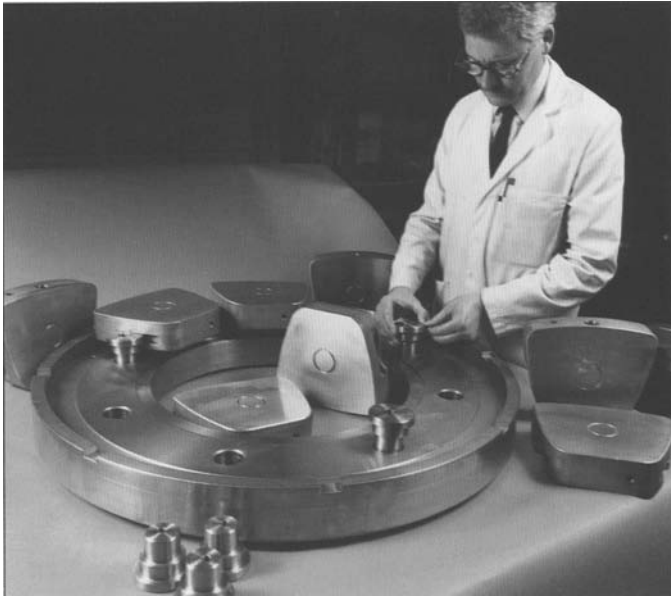
Figure 12-22. Glacier bearing featuring high pressure jacking oil for start up and run down. Jacking oil annulus can be seen on the surface of each thrust pad.
