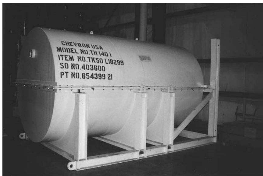
Figure 18-11. Shipping container for turbomachinery rotor. Although immersed in pressurized nitrogen, the rotor is protected by RUST-BAN 392. (Source: Sulzer-Hickham Industries, Inc., LaPorte, Texas)
