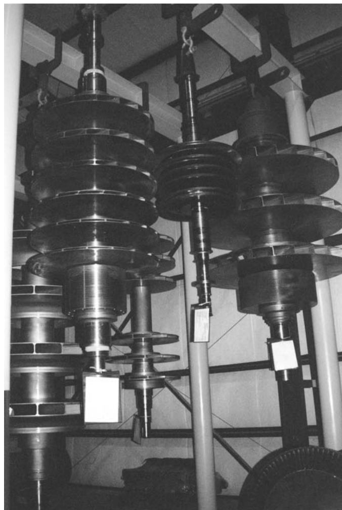
Figure 18-9. Turbomachinery rotors in humidity-controlled indoor storage at Sulzer-Hickham Industries, Inc., LaPorte, Texas.
