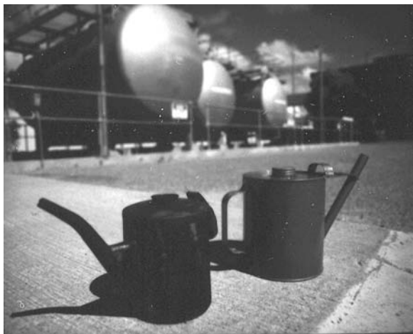
Figure 18-2. Rusty, or galvanized containers, are unsuitable for reliability-conscious lube transfer.
