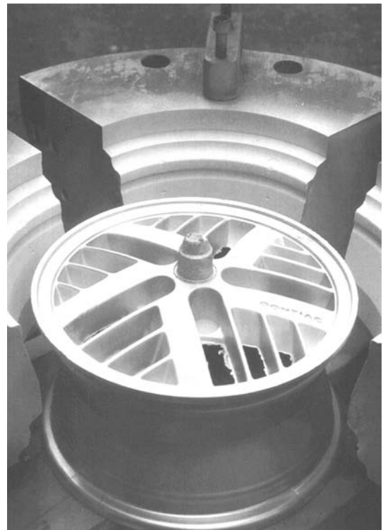
Figure 10-1. Releasing the mold of an aluminum rim.
