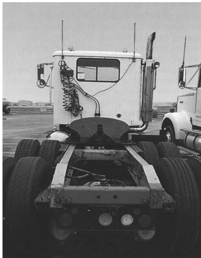
Figure 9-4. LIDOK EP 2 Moly is recommended for applications characterized by sliding or oscillating movements, such as the fifth wheel shown above.
