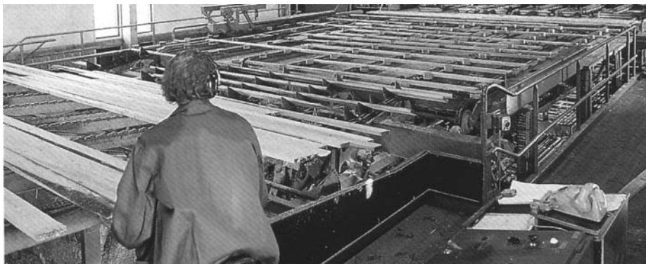
Figure 11-7. Forest product processing machinery using open, centralized lubrication. (Source: Safematic, Inc., Alpharetta, Georgia, and Muurame, Finland.)
