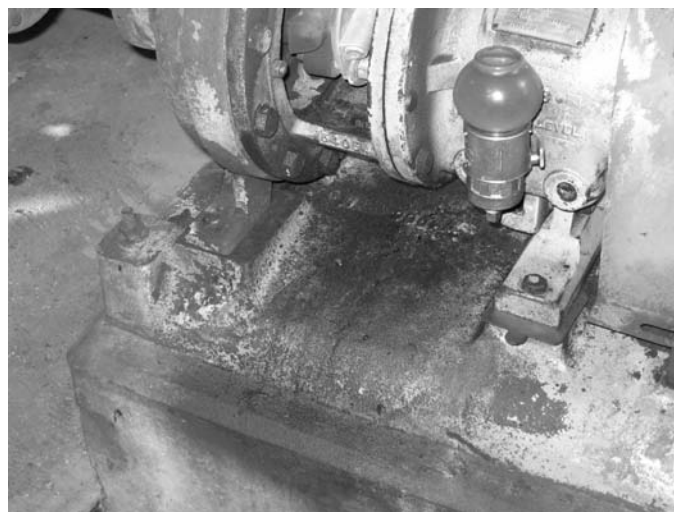
Figure 11-18. Conventional "non-balanced" constant level lubricator, shown here in overfilled condition
