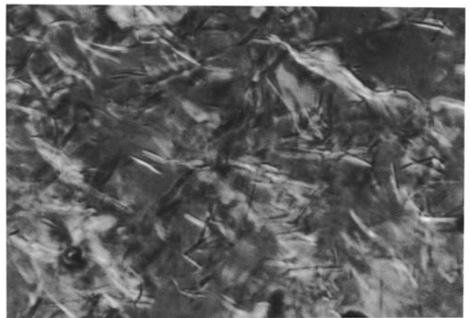
Figure 7-19. At -18°C, SYNESSTIC 32 (top photo) has no wax crystals, while a typical mineral oil (bottom photo) shows significant crystallization. The dark spots in the SYNESSTIC photo are air bubbles in the sample.
