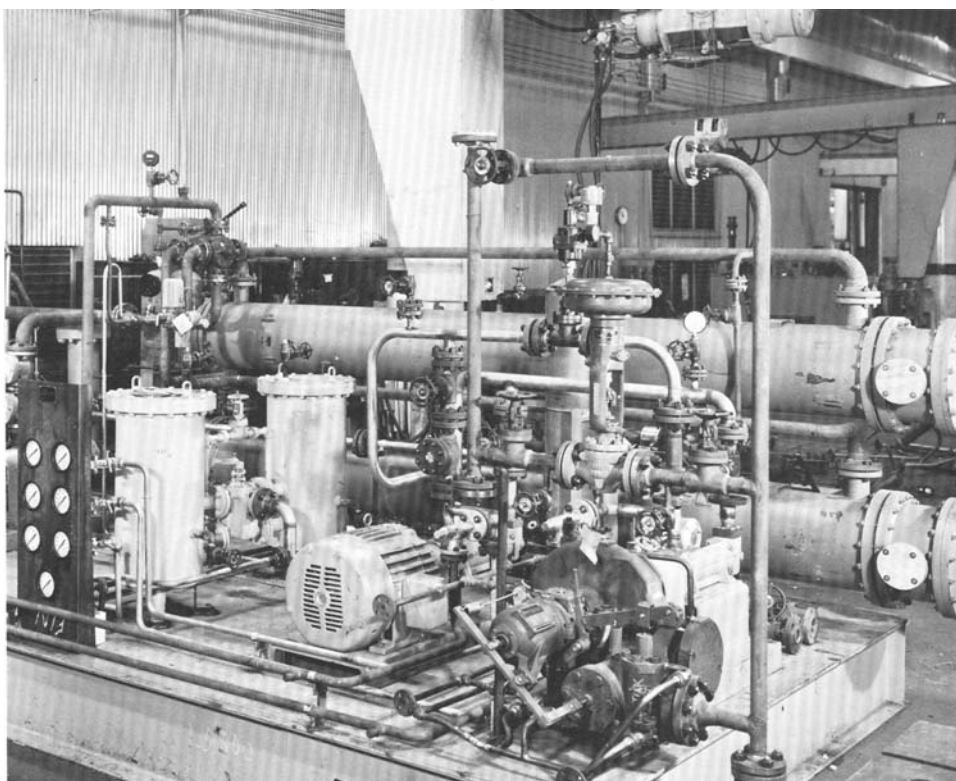
Figure 15-12. Lube/seal oil skid for a centrifugal compressor. (Source: Elliott Company, Jeanette, Pennsylvania).
