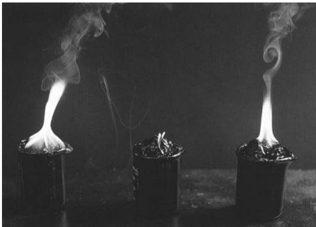
Figure 9-6. This demonstration dramatically illustrates the flame-retardant capabilities of FIREXX Grease (center) compared with two conventional greases (lithium complex and aluminum complex, respectively). The FIREXX Grease sample resisted ignition and, once lit, extinguished itself within seconds. The photograph was taken approximately 20 seconds after igniting the conventional greases and 12 seconds after igniting the FIREXX Grease.
