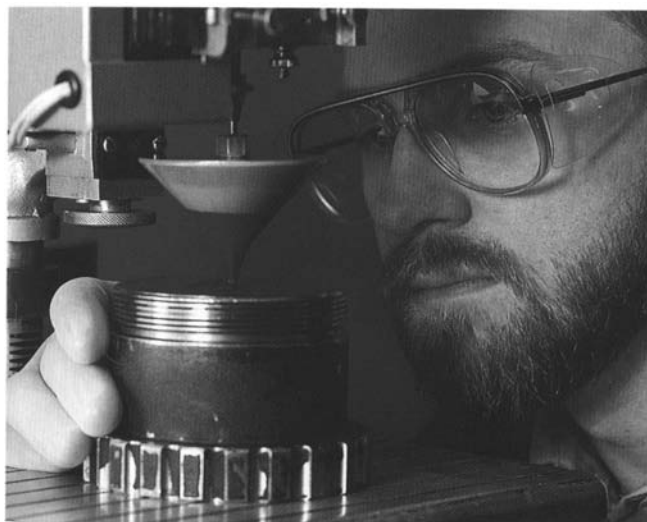
Figure 9-1. Greases are graded according to their consistency, i.e., resistance to deformation under the application of force. Consistency is measured with a penetrometer—shown here—and is reported as the tenths of a millimeter that a standard cone will penetrate the test sample under conditions prescribed by ASTM D 217. The softer the grease, the higher the penetration number.
