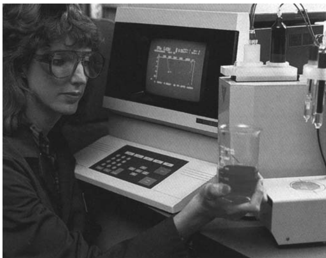
Figure 9-2. A technical specialist at Exxon's Pittsburgh grease plant measures the acidity/alkalinity of grease components on a titrator.
