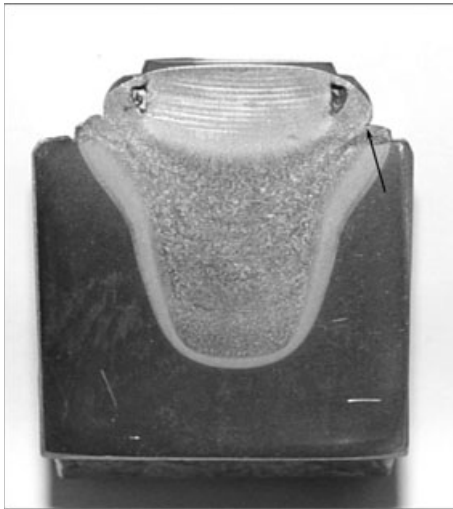
7.14 Friction taper stud weld made in 40 mm plate of 10CrMo910 creep-resistant steel. The tool is a consumable in this process and has been cut off after completing the weld. In practice the protruding part of the stud tool would be ground back to the surface with care taken to eliminate the 'flash crack' (arrow).
