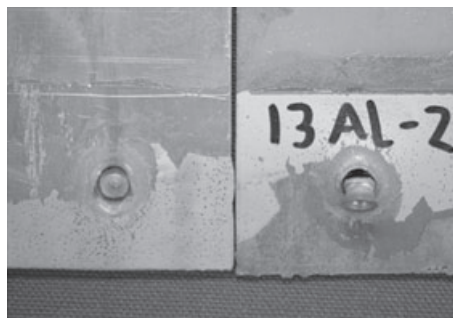
11.12 Bond strength test results for Dow Betamate 4601 and Betamate 1480 joining 2-mm AA5182-O to 1.6-mm DP600: (a) load versus displacement curve; (b) failure mode.
