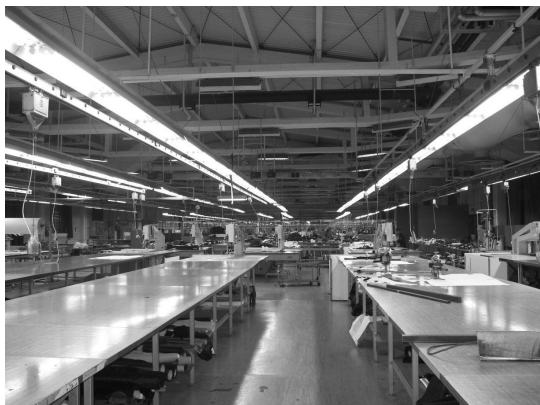
Figure 5.14 Cutting tables and overhead electrical cords
