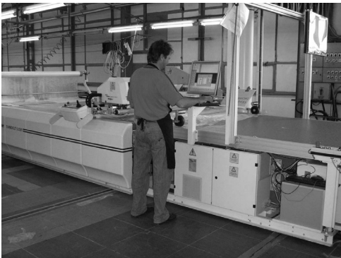
Figure 5.19 CAM system for cutting
