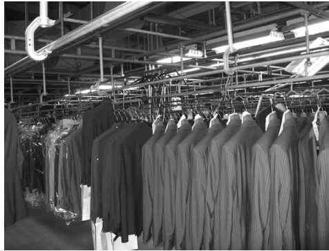
Figure 5.38 Storage with overhead conveyor
