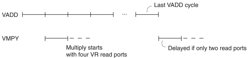
Figure 3.20 For logically independent vector instructions, the number of access paths to the vector register (VR) set and vector units may limit performance. If there are four read ports, the vector multiply (VMPY) can start on the second cycle. Otherwise, with two ports, the VMPY must wait until the VADD completes use of the read ports.
