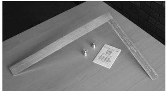
**Fig. 8.13** *Stanley and Smallwood steel roofing squares*
