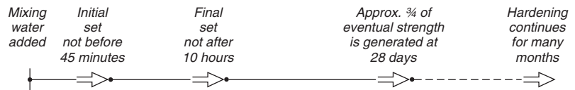
Figure 2.8 Typical setting and hardening timescale for ordinary Portland cement
