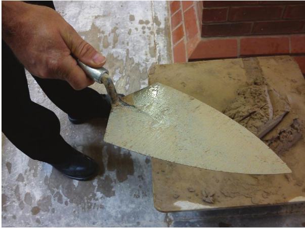
Fig. 106 Correct method of holding the trowel.
