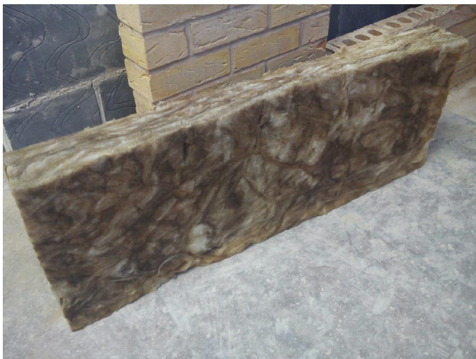
Fig. 173 Full-fill cavity-wall insulation.
