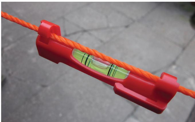
Fig. 52 Line-level attached to the ranging line.
