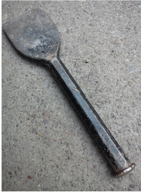
Fig. 80 Narrow bolster chisel with worn 'mushroom' head.
