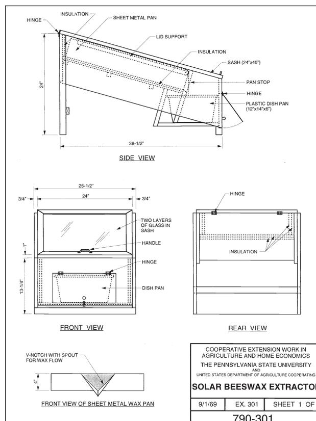
**Figure 66.** Plans for constructing a solar beeswax extractor.
