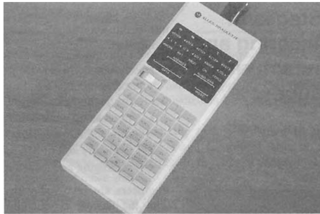
(b) A typical hand-held PLC programmer
