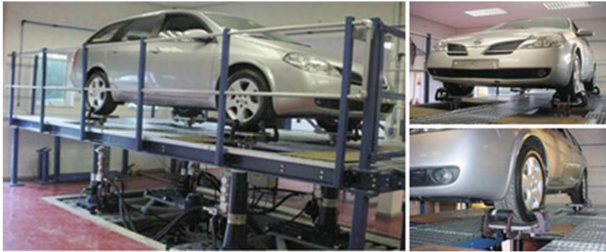
Fig. 4.26 Four poster dynamic test rig
