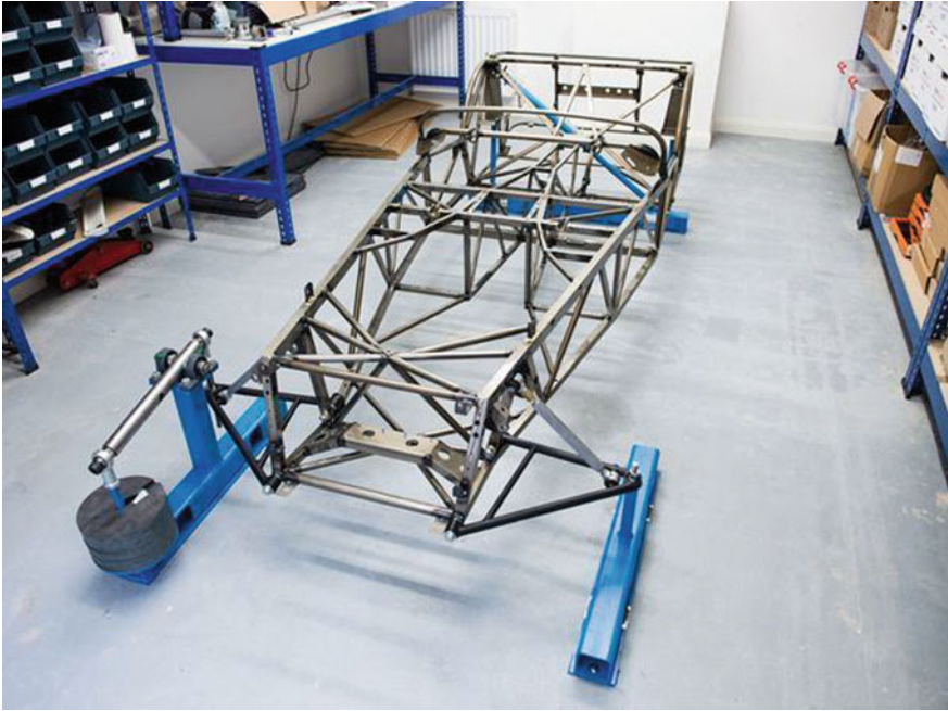
Fig. 4.7 Torsional test of space-frame chassis.
