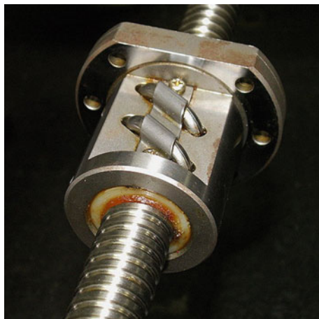
Fig. 2.21 Recirculating ball screw as used on a steering system.
