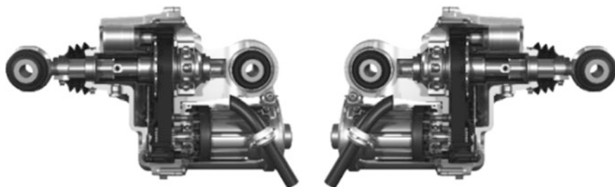
Fig. 2.55 Image of a dual actuators—each rear wheel steered independently. Reproduced with kind permission of ZF © ZF Friedrichshafen AG
