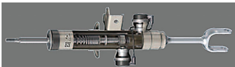
Fig. 3.43 Two external CDC valves used to control bump and rebound continuously and independently.
