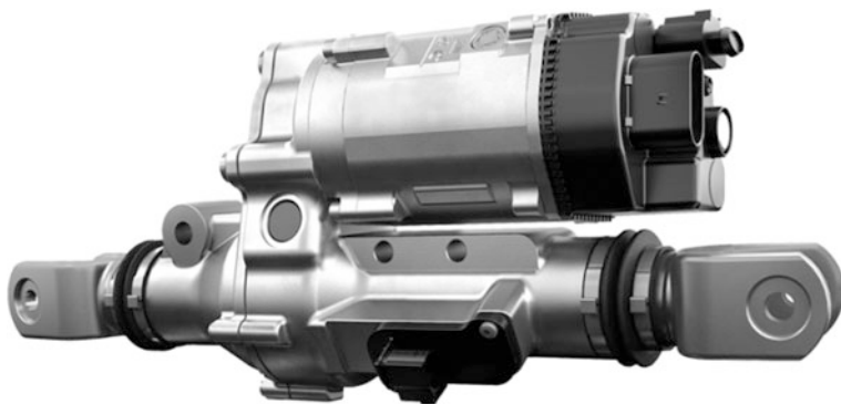
Fig. 2.54 Image of a single (central) actuator that steers both rear wheels together. Reproduced with kind permission of ZF © ZF Friedrichshafen AG
