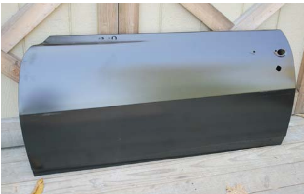
This is a new Dynacorn door for the Firebird. It has a black E-coating, which makes it easy to check for flaws. Sighting down the body line on the door, it's easy to see how straight the line is.
