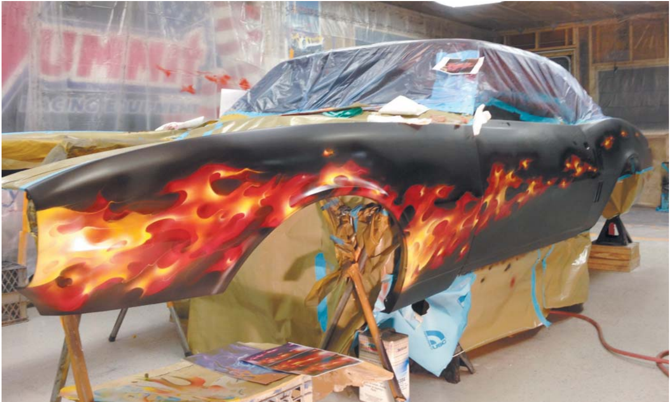
The real fire flame artwork has been completed on the Firebird. Now it must be clearcoated to protect and level out the layers of the artwork.
