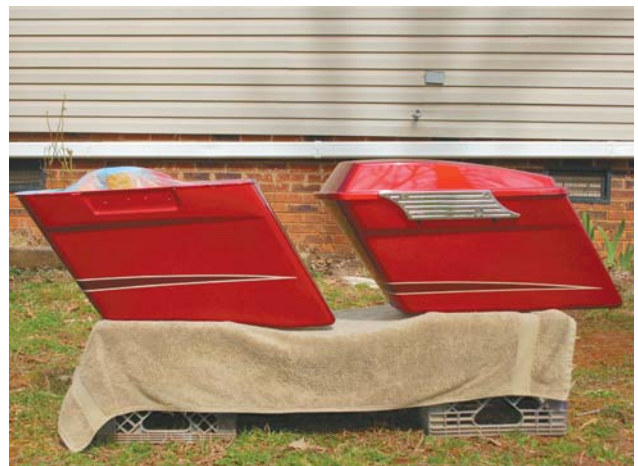
One last color match: candy red pearl with a dark red pearl graphic and off white pearl pinstripe. This was a toughie as I had to use flop adjuster in the base and also in the candy pearl color, which was layered over the base. I got the red candy pearl and the dark red pretty close. The pinstripe is a little light. It took many samples to get all three colors matched up. Eight days were spent doing the color match for this job alone.
