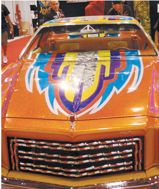
Here's a lowrider with graphics by Craig Fraser. The hood and top surface of the car were layered with flake, and then Craig applied the graphics.
