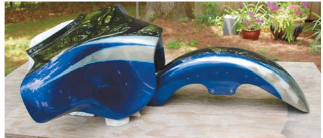
Left: Now the real test—it's easy enough to match a small sample piece, but will the colors sprayed onto a large fairing match up? The candy has to be sprayed evenly, using the same gun speed, the same pattern overlap, and the same concentration as the sample. In the sun, the fairing I painted appears to be a good match to the fender I'm trying to match. Right: Again, it even matches up pretty well in the shade. For this paint job, I actually had to match four colors and one textured silver effect.
