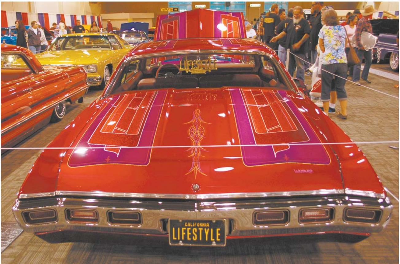
This is a classic lowrider-style paint job. Note the use of the flake paint in the graphics. Complex designs are simply a matter of breaking down the elements of the design, creating the order in which the elements will be painted, and then, one by one, painting those elements.
