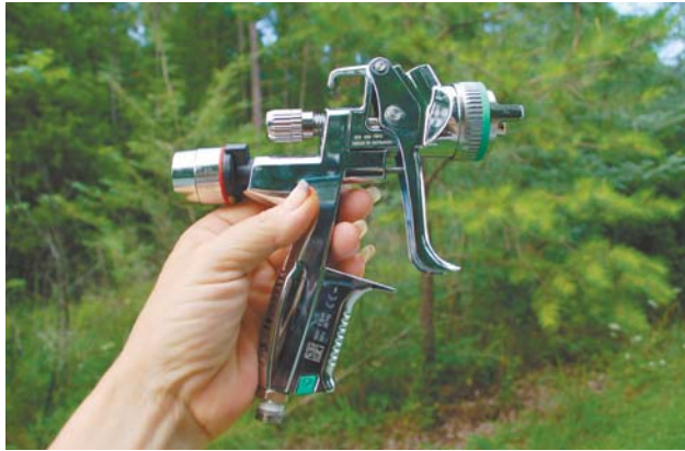
This is the SATA 4000 HVLP spray gun with its WSB (water-soluble basecoat) 1.25 mm nozzle set installed.
