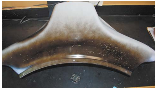
This motorcycle fairing was ready for paint but the cloth used to clean it was contaminated. It's easy to see how the contamination was wiped across the surface. All the black paint was sanded off the surface, and the gray primer was wiped several times with precleaner.
