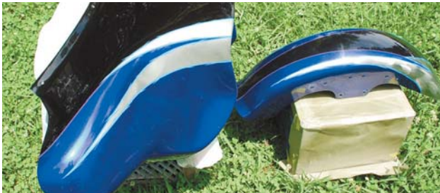
Left: Now the real test—it's easy enough to match a small sample piece, but will the colors sprayed onto a large fairing match up? The candy has to be sprayed evenly, using the same gun speed, the same pattern overlap, and the same concentration as the sample. In the sun, the fairing I painted appears to be a good match to the fender I'm trying to match. Right: Again, it even matches up pretty well in the shade. For this paint job, I actually had to match four colors and one textured silver effect.
