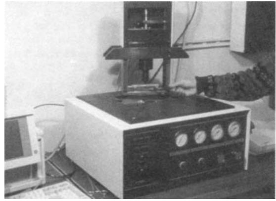
Bending Beam Rheometer
