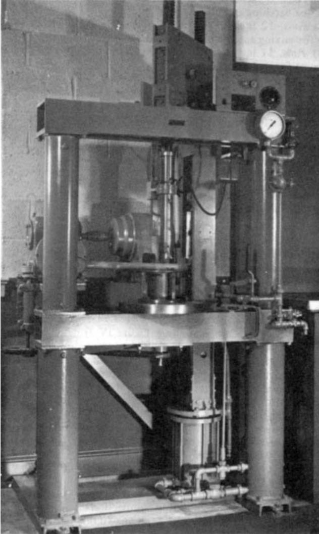
Figure 31 - Kneading Compactor and Diagram of Tamping Foot
