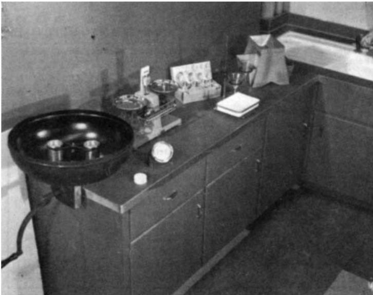
Figure 29 - Apparatus for the Hveem CKE Test
