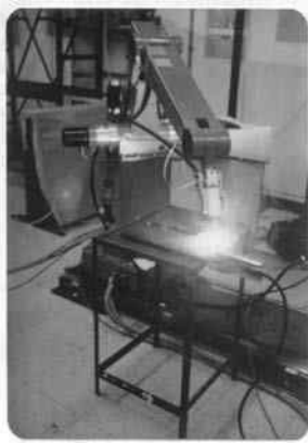
15.41 Welding carried out by ASEA robot
