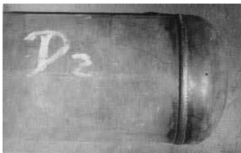
5.46 Appearance of liquid acetylene vessel welded using the present method
