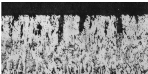
Figure 17.10 Lead corroded from copper–lead bearing by oxidized oil. Source: Adapted from Burgess, 1953.
