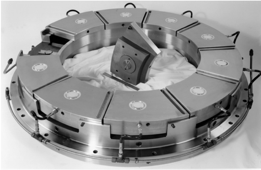
Figure 7.13 Pivoted pad thrust bearing with leading edge oil feed groove and oil lift pockets for low-friction starting. Source: Courtesy of Kingsbury, Inc.
