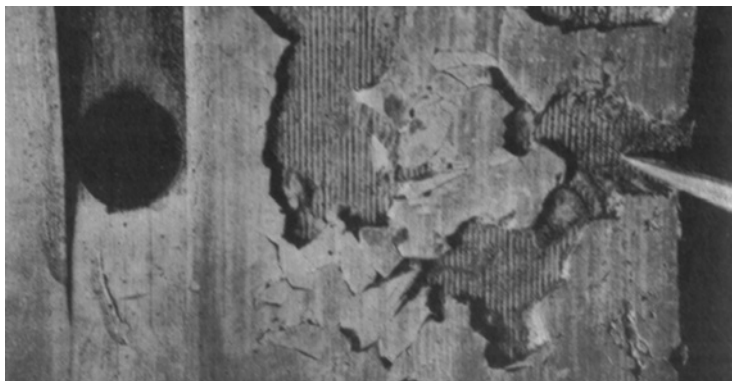
Figure 17.7 Fatigue failure of babbitt bearing. Source: Adapted from Burgess, 1953.
